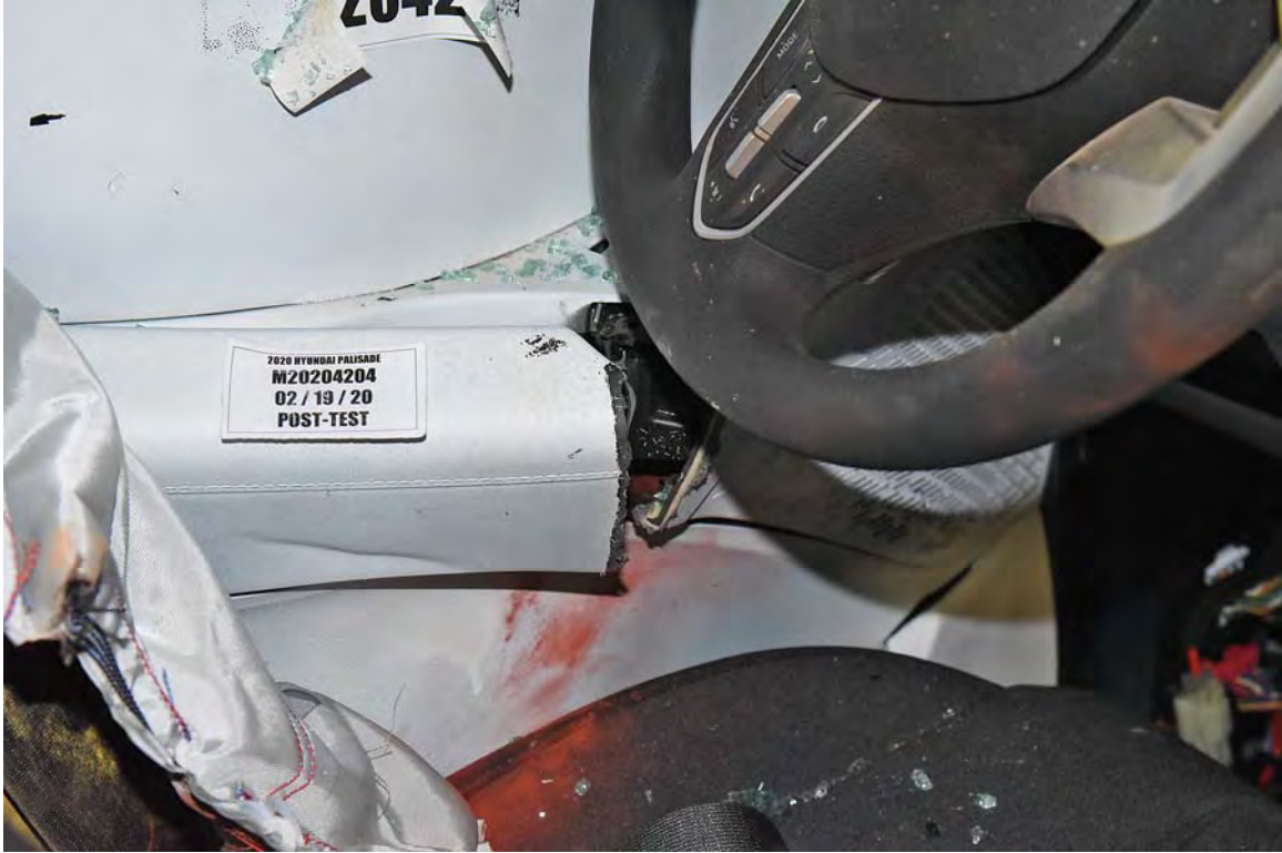
FIGURE 71. Post-Test View of Shattered Vehicle Inner Door Panel
