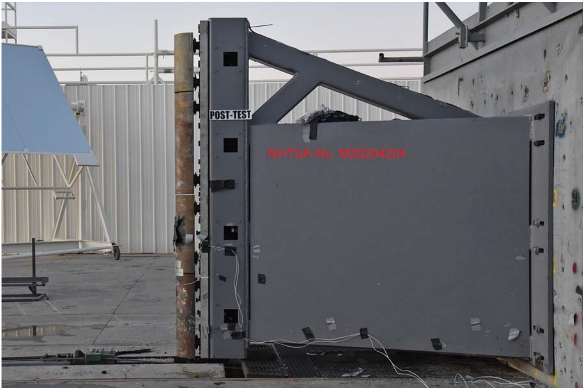
FIGURE 60. Post-Test Pole Barrier Side View
