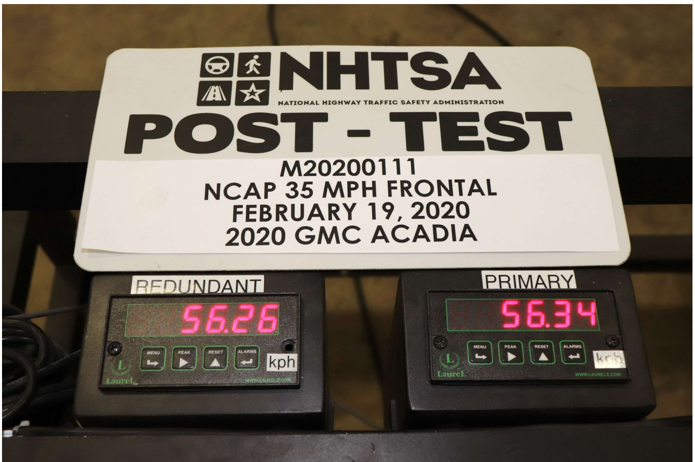
Photo No. 076 - Post-Test Speed Trap Read-Out
