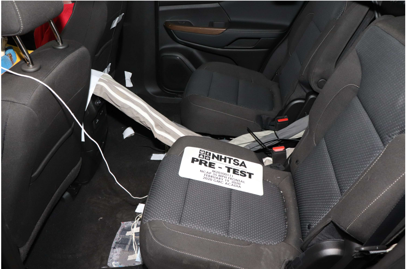
Photo No. 028 - Pre-Test Dummy Cable Routing
