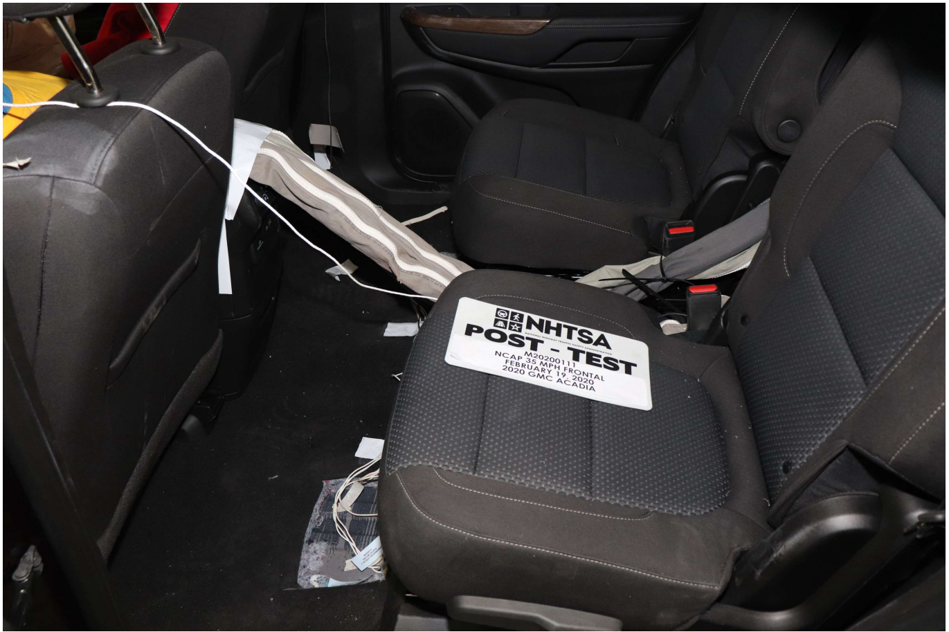
Photo No. 029 - Post-Test Dummy Cable Routing
