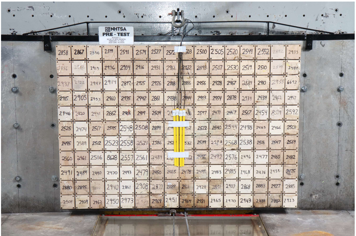
Photo No. 002 - Pre-Test Load Cell Wall
