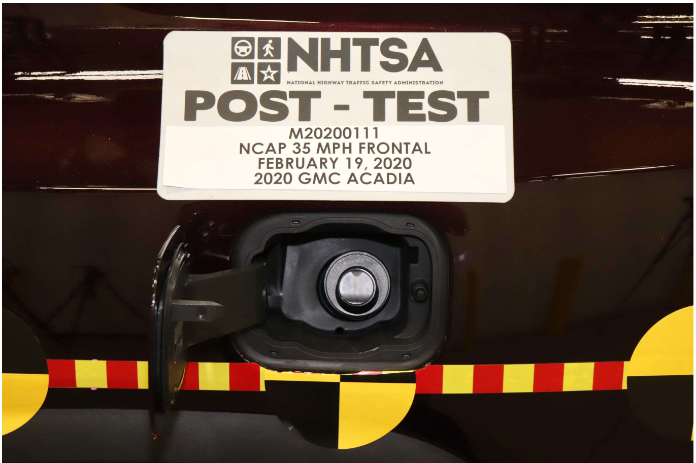
Photo No. 023 - Post-Test Fuel Filler Cap View
