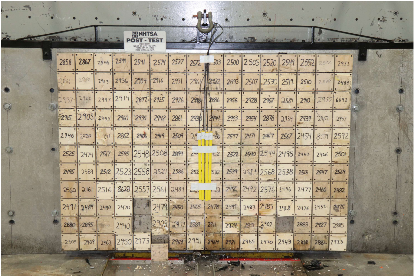
Photo No. 003 - Post-Test Load Cell Wall
