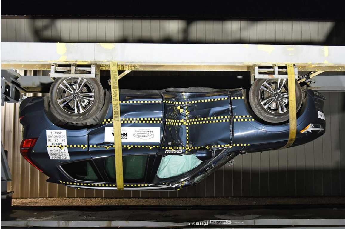
FIGURE 65. FMVSS No. 301 Static Rollover 180 Degrees
