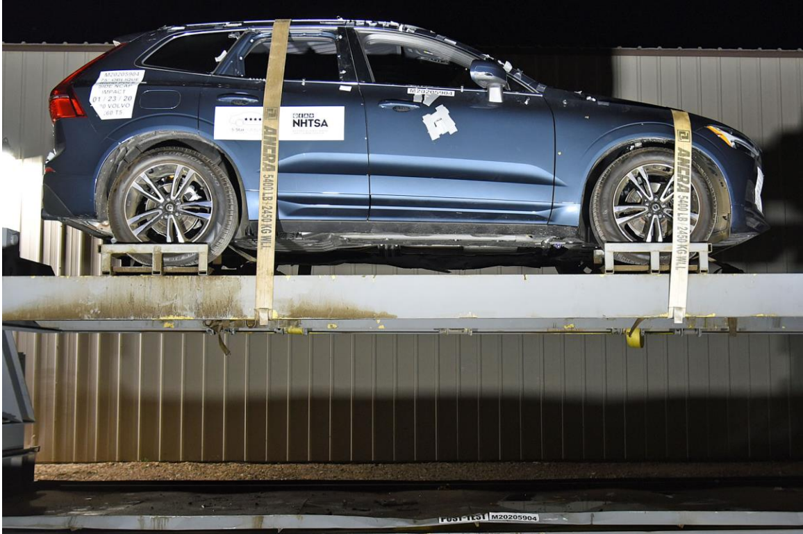
FIGURE 67. FMVSS No. 301 Static Rollover 360 Degrees
