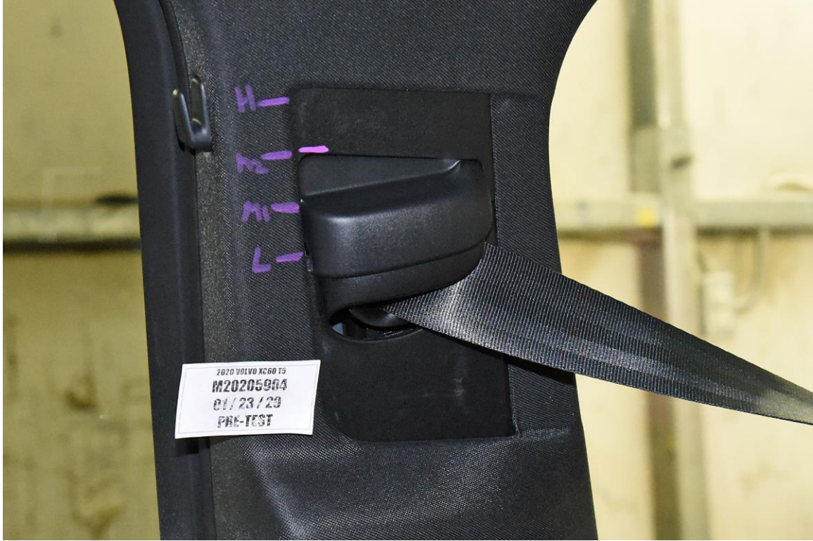
FIGURE 33. Pre-Test View of Belt Anchorage for Dummy
