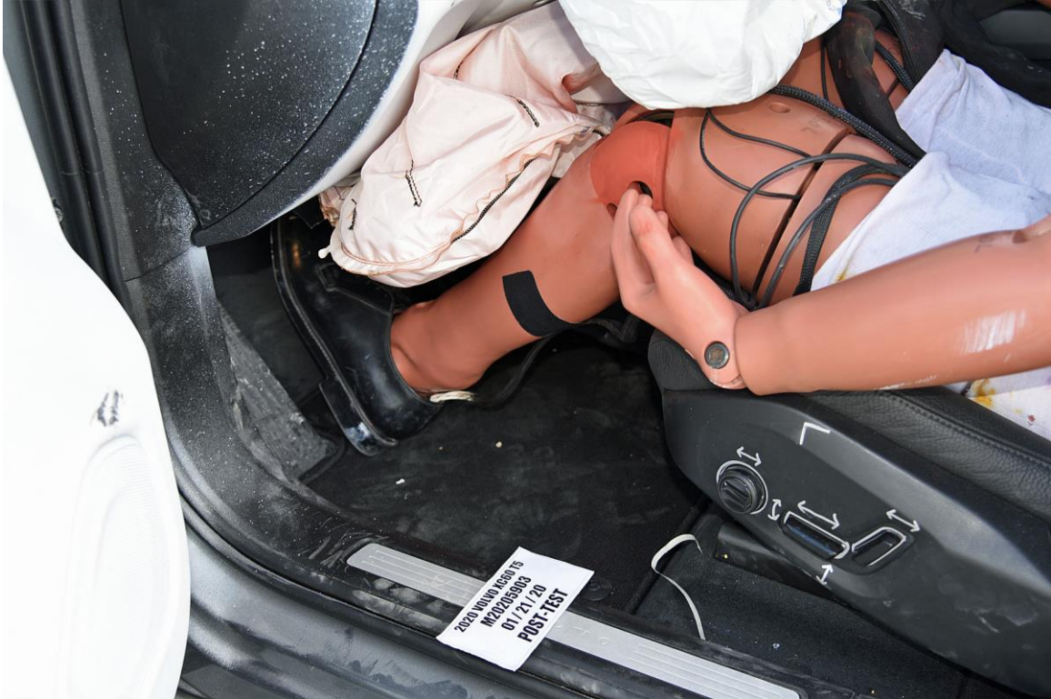
FIGURE 43. Post-Test Driver Dummy Feet
