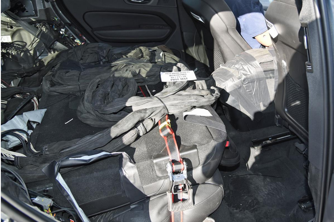
FIGURE 29. Post-Test Dummy Cable Routing
