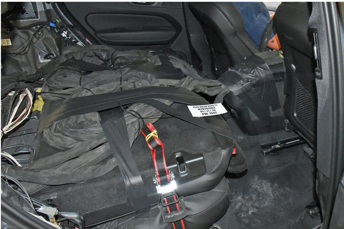
FIGURE 28. Pre-Test Dummy Cable Routing
