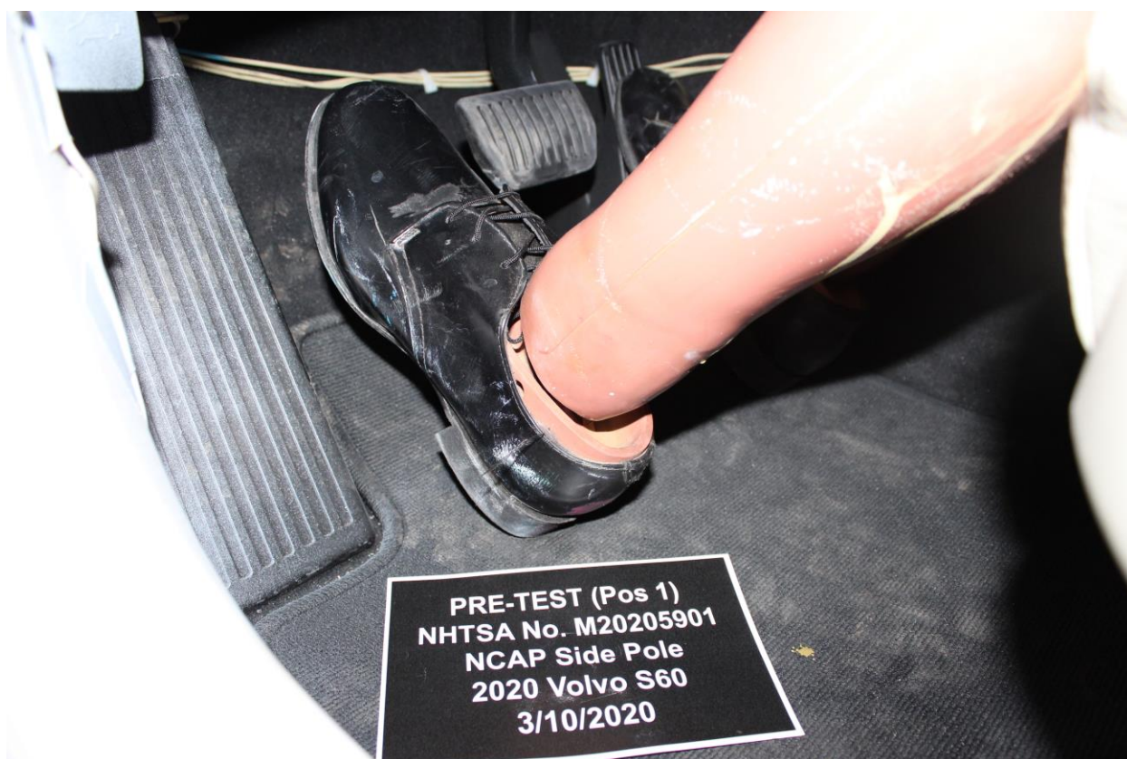
Figure A-32: Pre-Test Placement of Dummy's Feet
