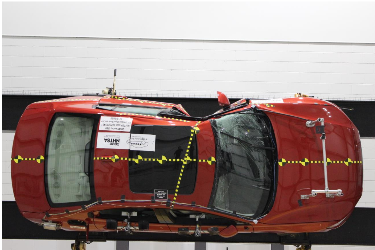
Figure A-64: FMVSS No. 301 Static Rollover 90 Degrees
