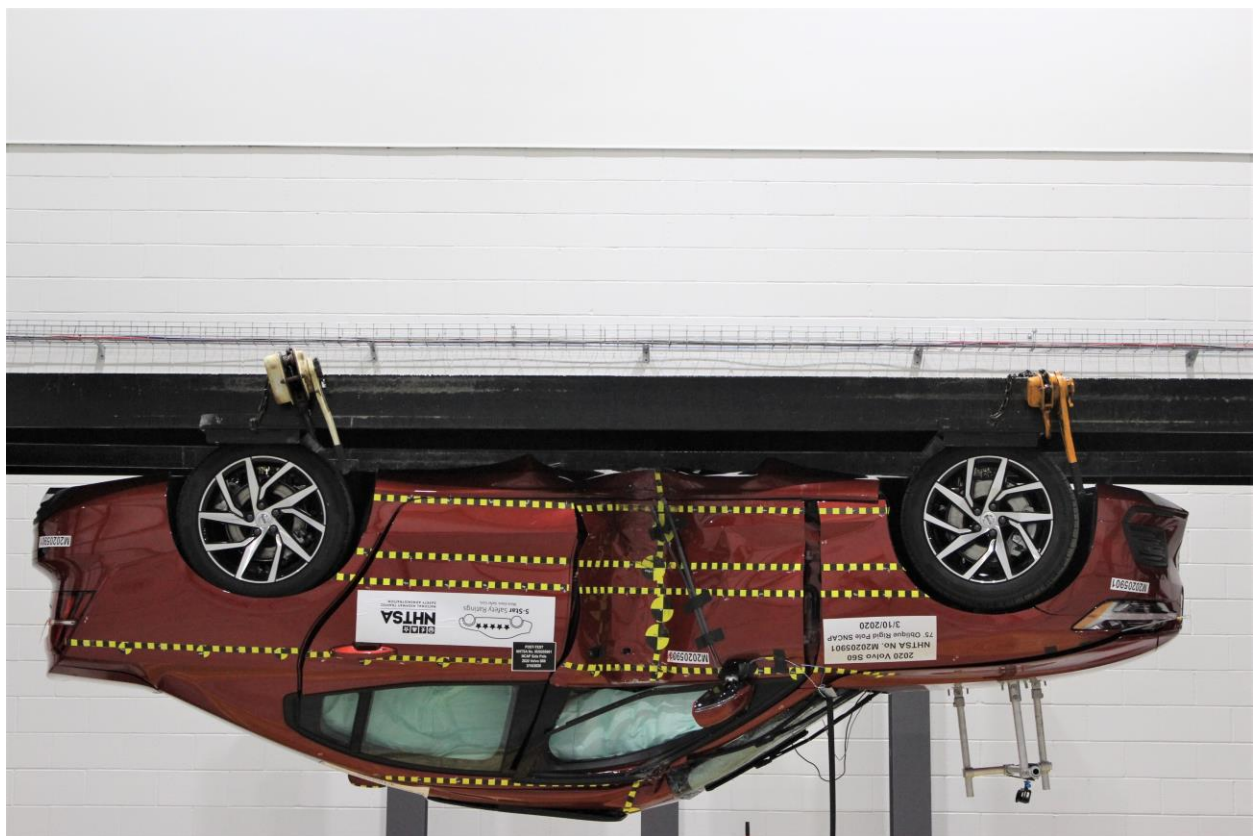
Figure A-65: FMVSS No. 301 Static Rollover 180 Degrees
