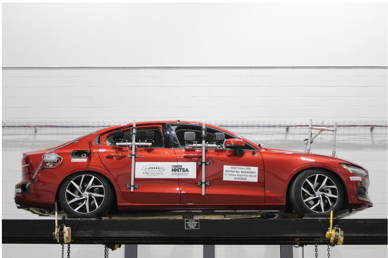
Figure A-67: FMVSS No. 301 Static Rollover 360 Degrees
