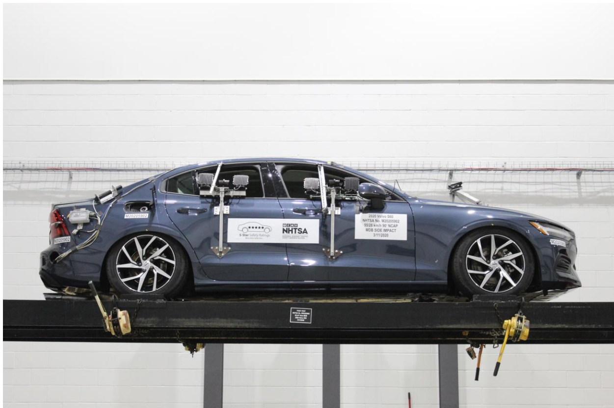
Figure A-96: FMVSS No. 301 Static Rollover 0 Degrees
