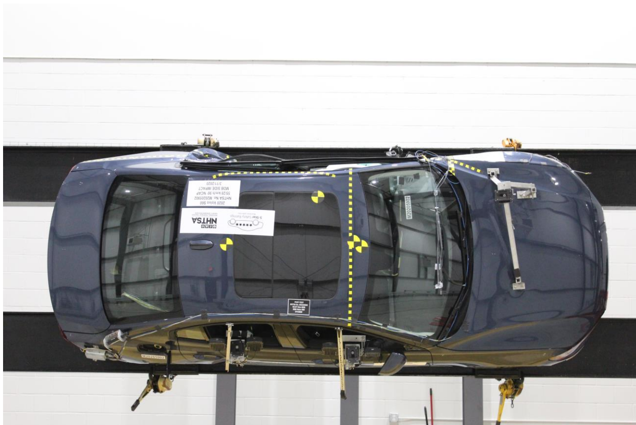
Figure A-97: FMVSS No. 301 Static Rollover 90 Degrees
