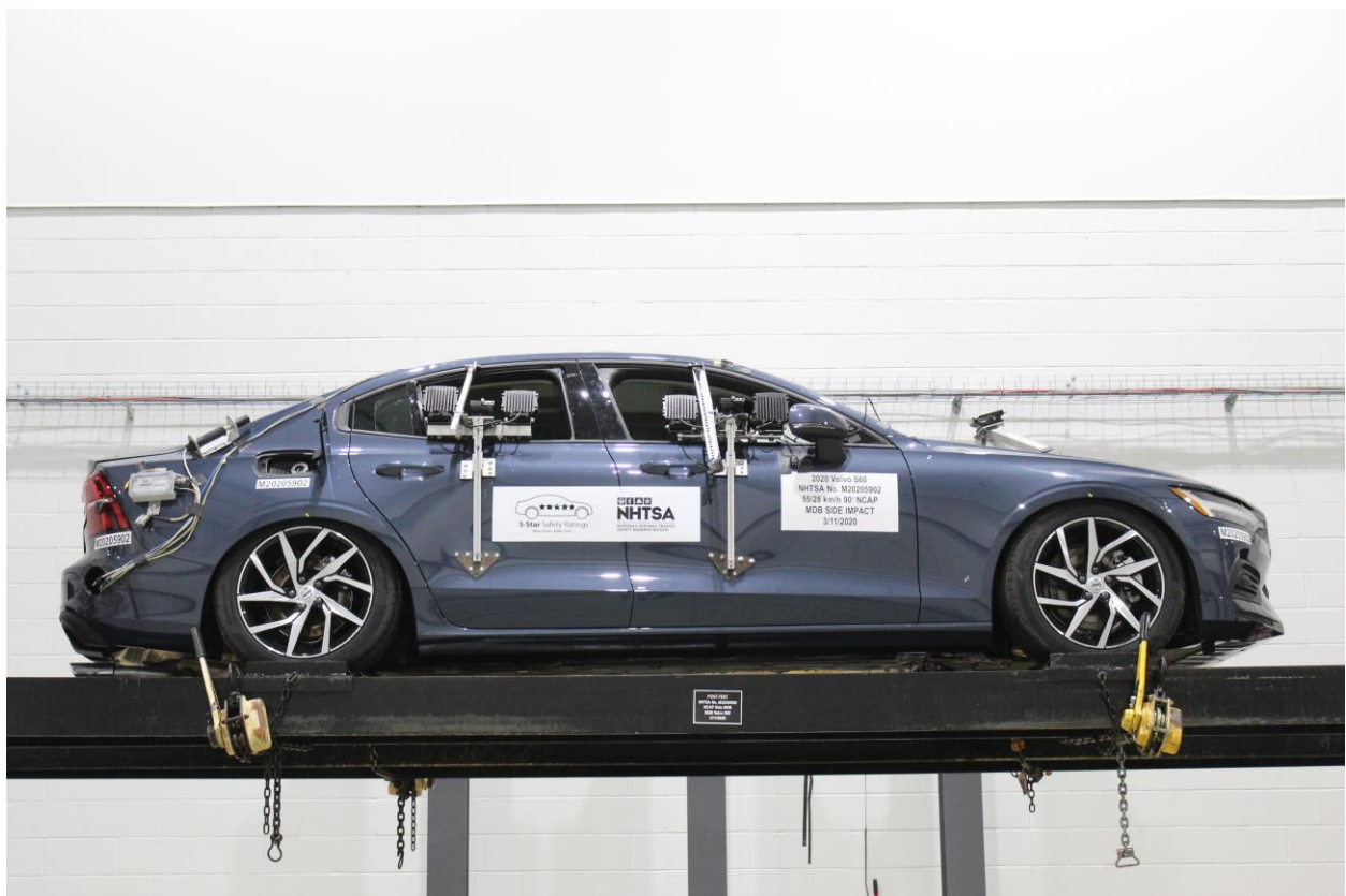
Figure A-100: FMVSS No. 301 Static Rollover 360 Degrees
