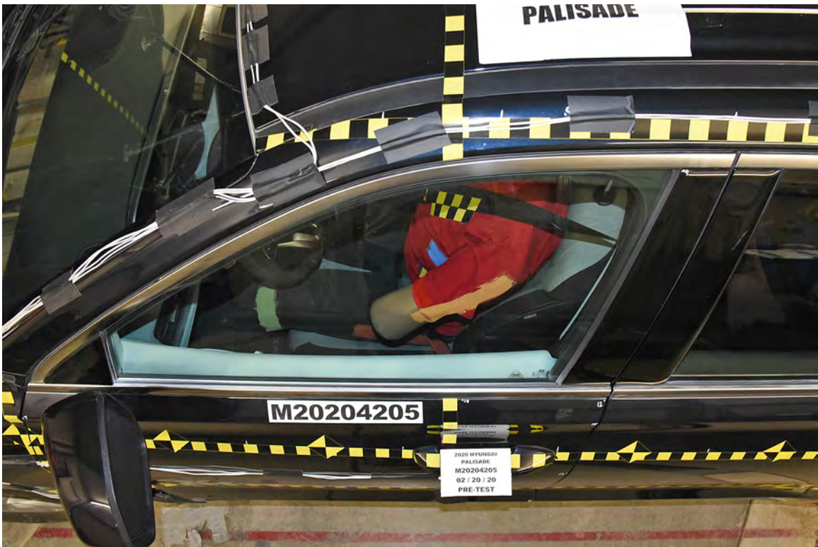
FIGURE 42. Pre-Test Driver Dummy and Door Clearance View
