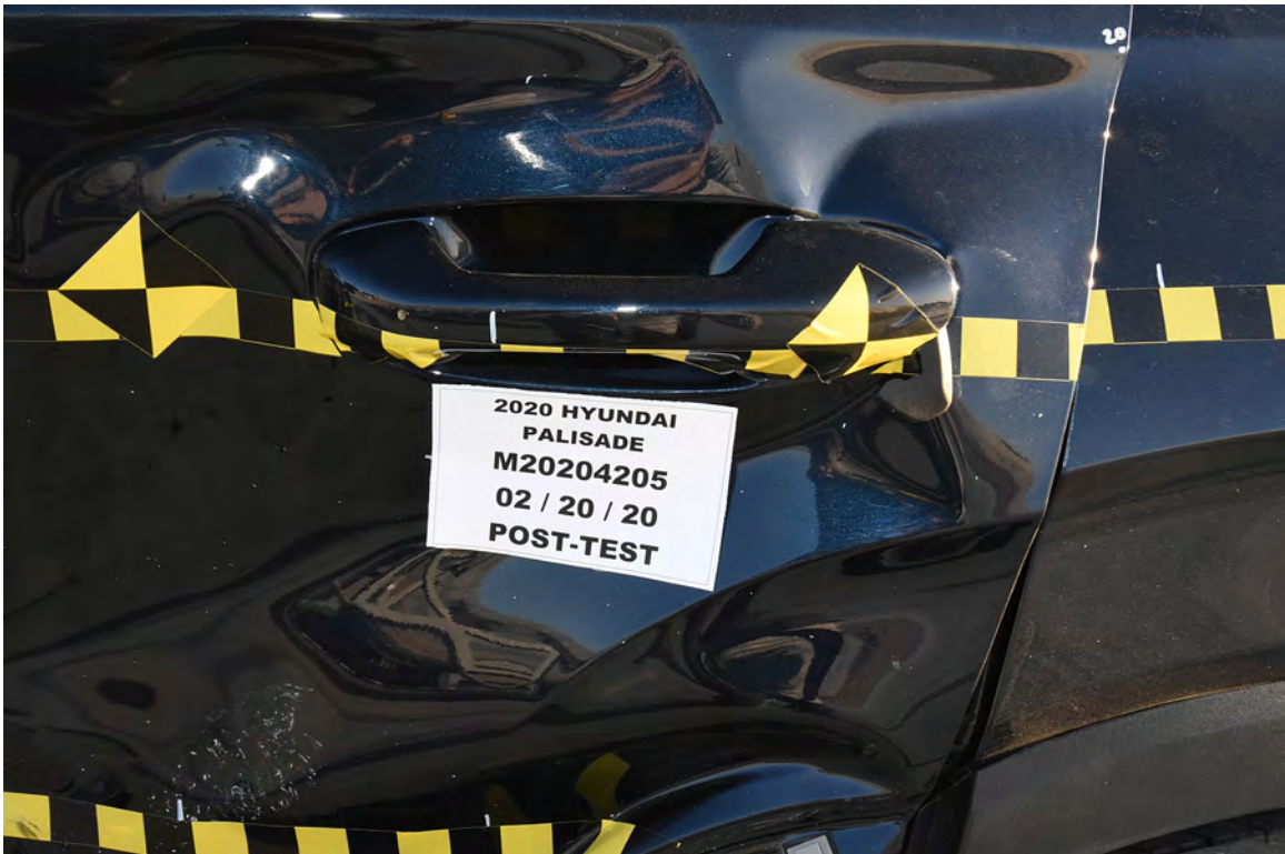
FIGURE 24. Post-Test Left Rear Door Latch Close-Up
