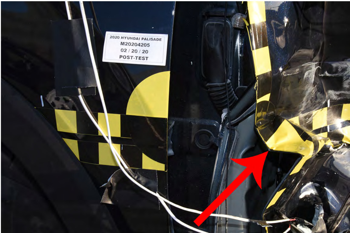
FIGURE 20. Post-Test Close-Up View of Impact Point Target
