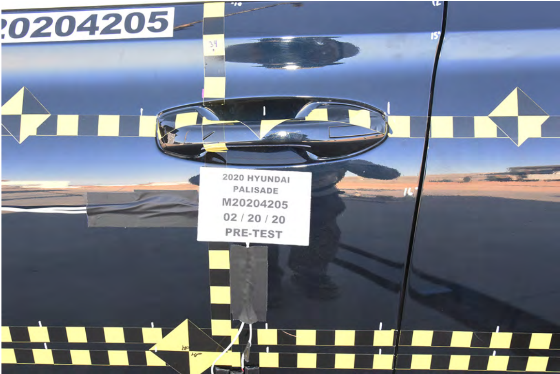
FIGURE 21. Pre-Test Left Front Door Latch Close-Up
