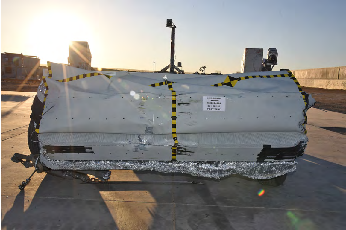
FIGURE 85. Post-Test Front View of MDB Impactor Face
