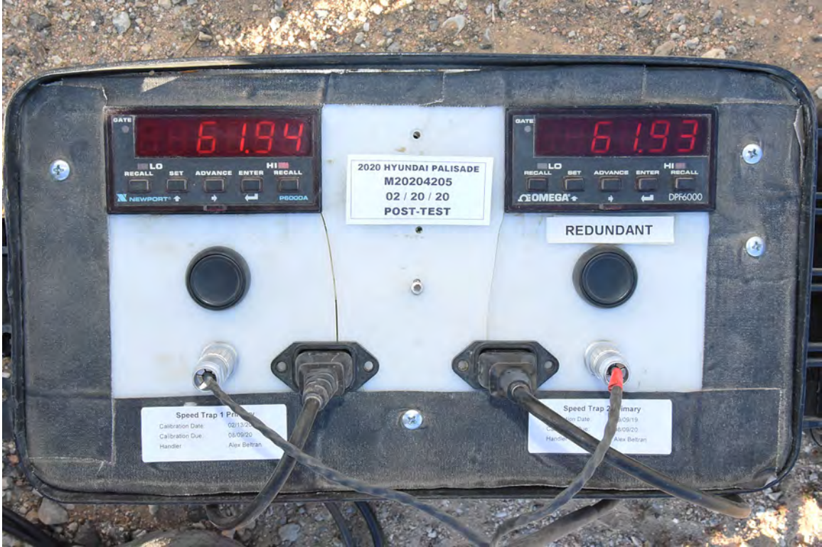
FIGURE 95. Post-Test Primary and Redundant Speed Trap Read-Out
