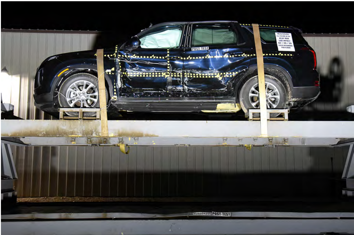
FIGURE 100. FMVSS No. 301 Static Rollover 360 Degrees
