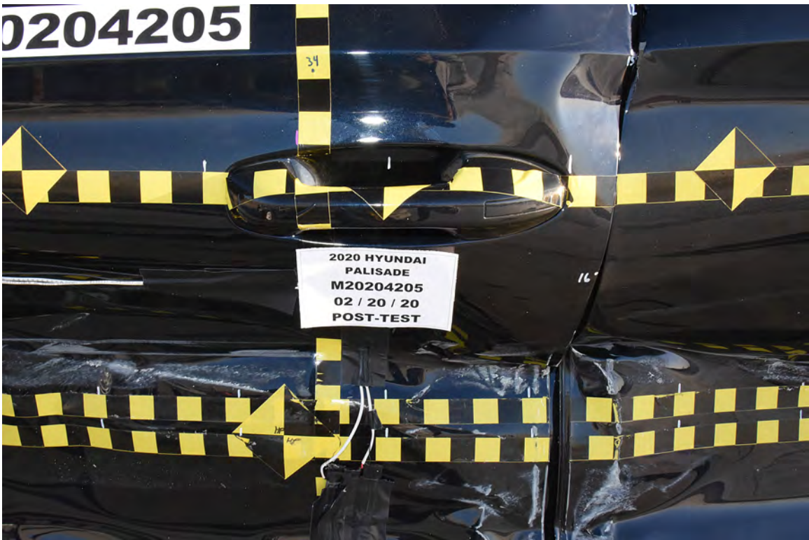
FIGURE 22. Post-Test Left Front Door Latch Close-Up
