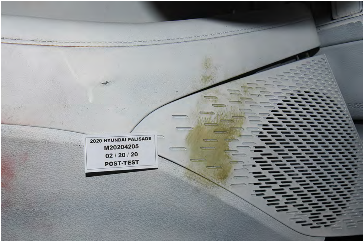
FIGURE 54. Post-Test Driver Dummy Close-Up Knee Contact View
