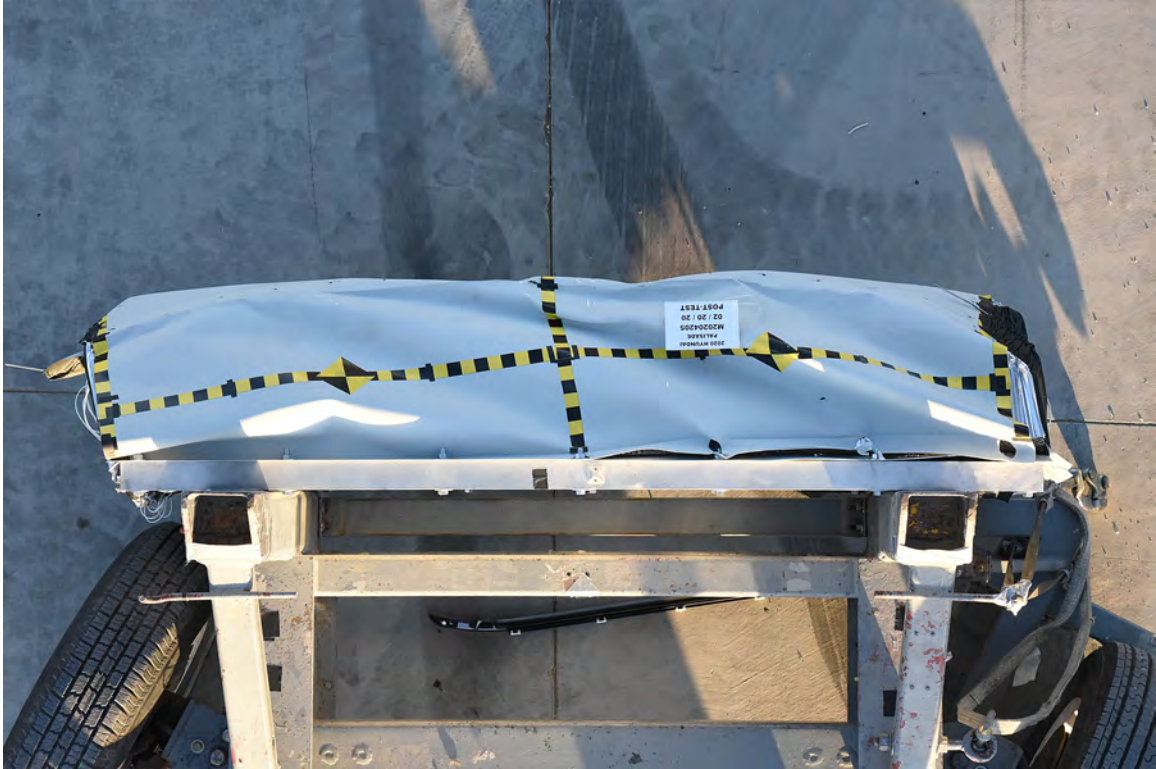
FIGURE 87. Post-Test Top View of MDB Impactor Face
