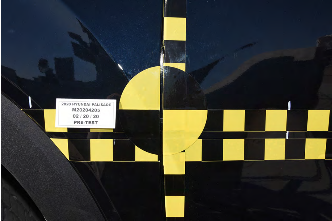
FIGURE 19. Pre-Test Close-Up View of Impact Point Target
