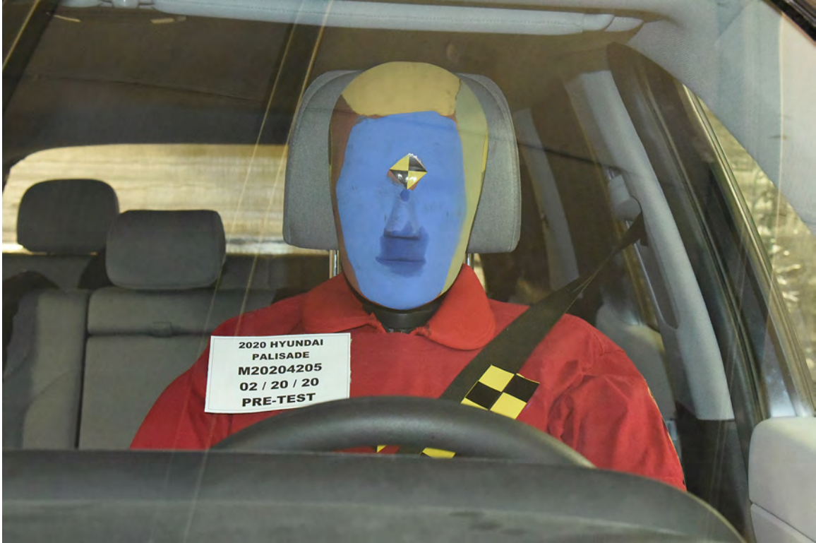
FIGURE 25. Pre-Test Front Close-Up View of Driver Dummy
