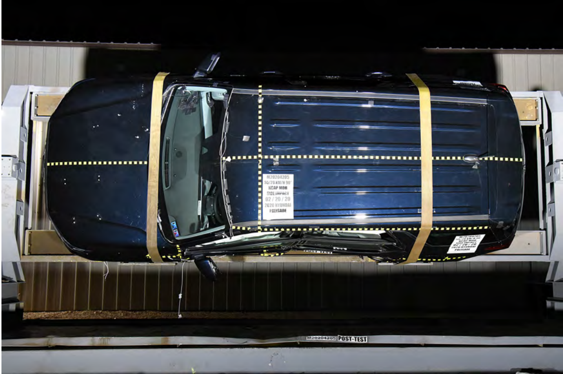
FIGURE 97. FMVSS No. 301 Static Rollover 90 Degrees
