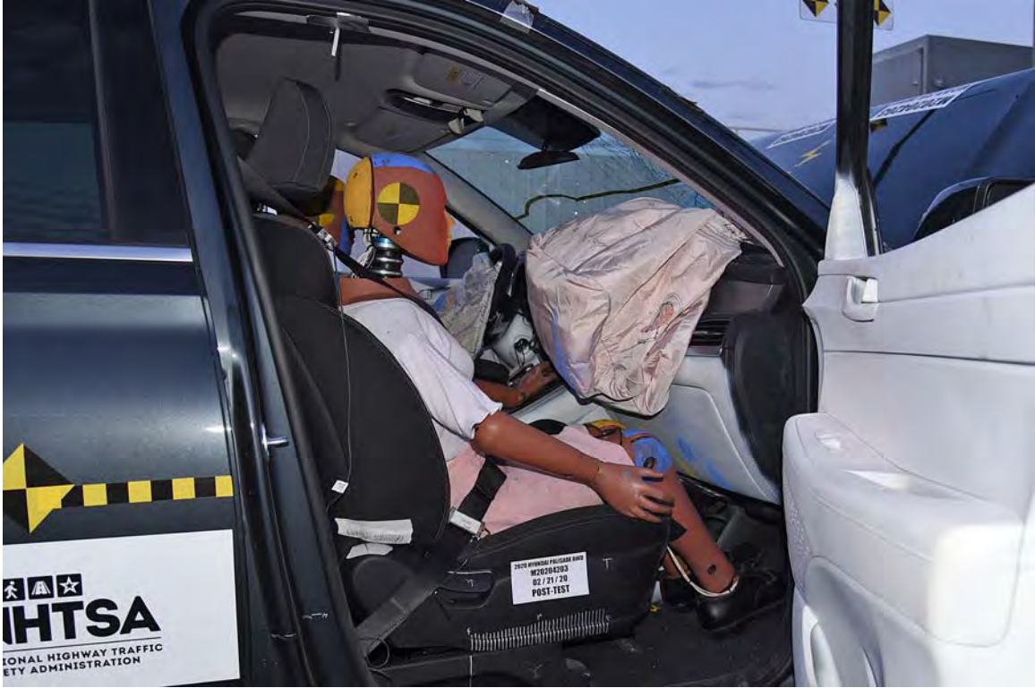
FIGURE 58. Post-Test Passenger Dummy and Vehicle Interior View
