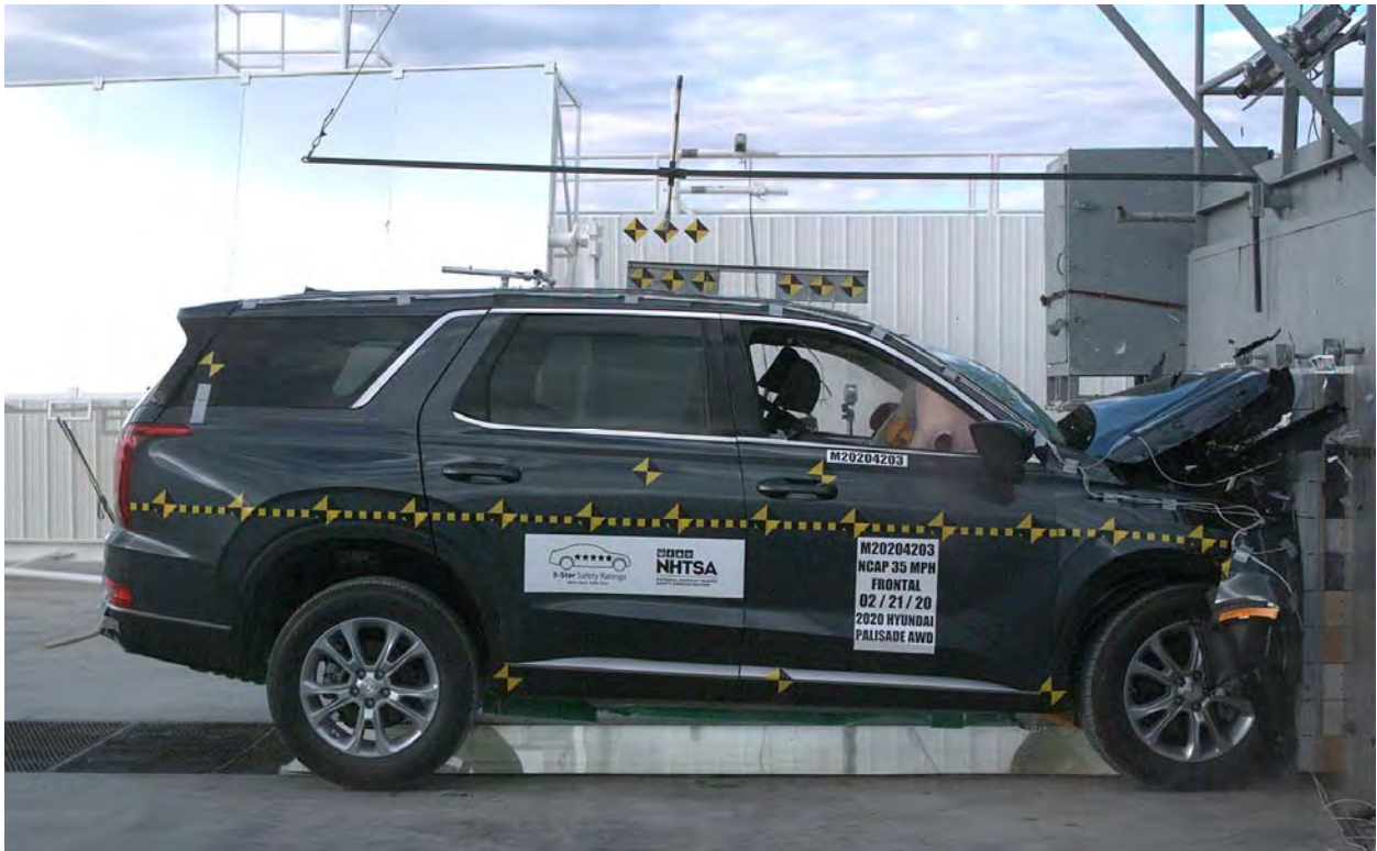
FIGURE 82. 2020 Hyundai Palisade AWD Frontal Impact Event
