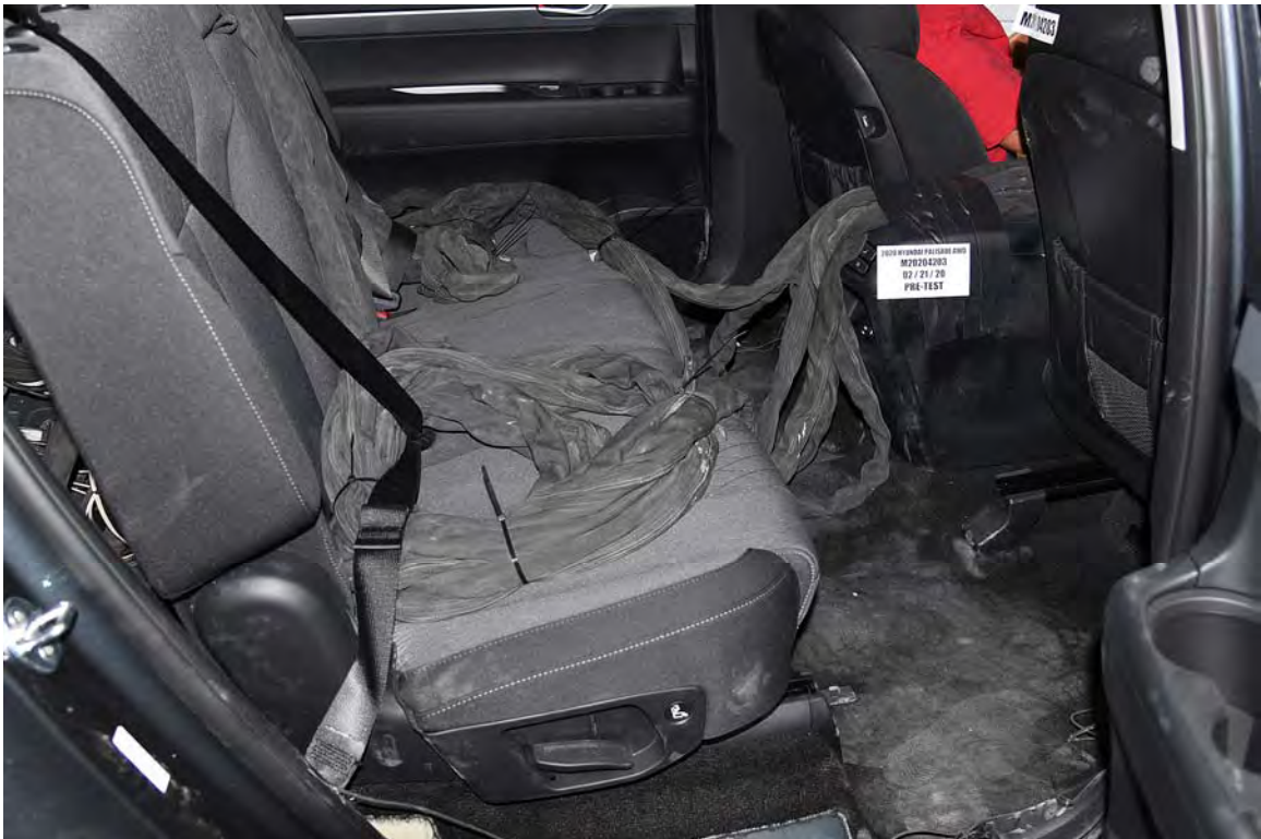
FIGURE 28. Pre-Test Dummy Cable Routing
