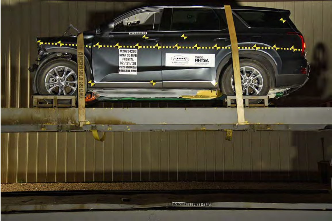
FIGURE 77. Vehicle at 0° on Static Rollover Device
