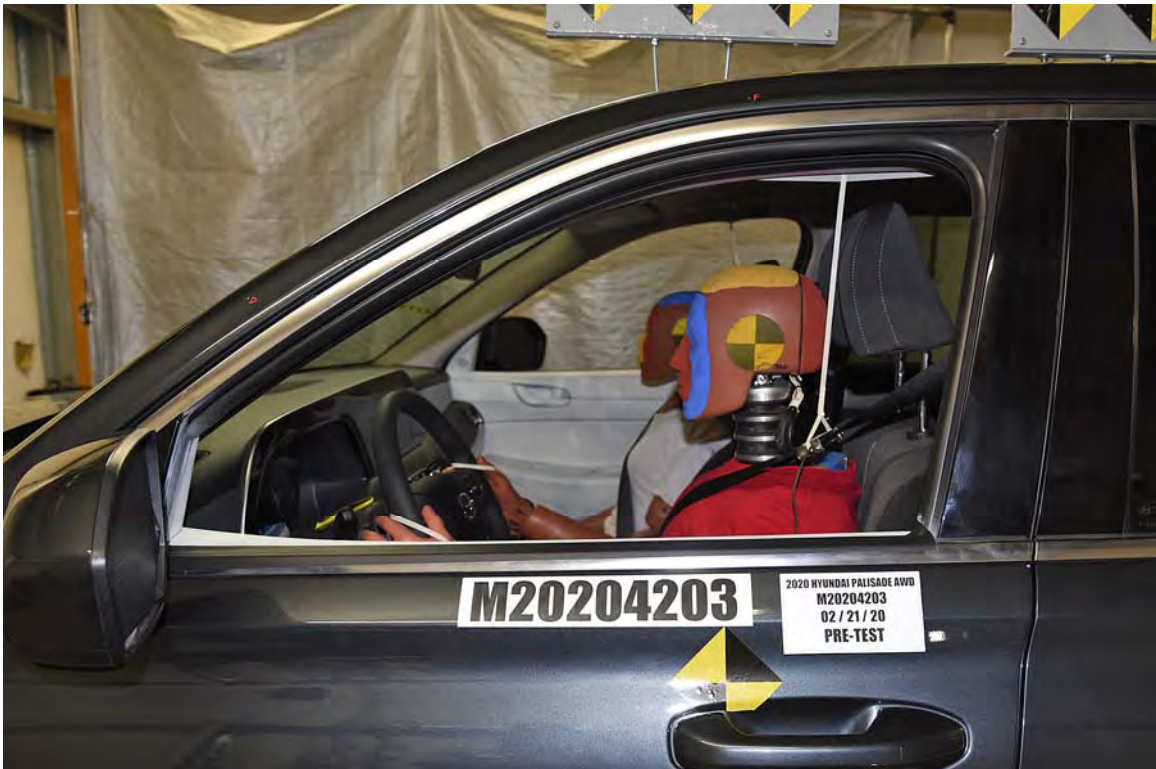
FIGURE 32. Pre-Test Driver Dummy Window View
