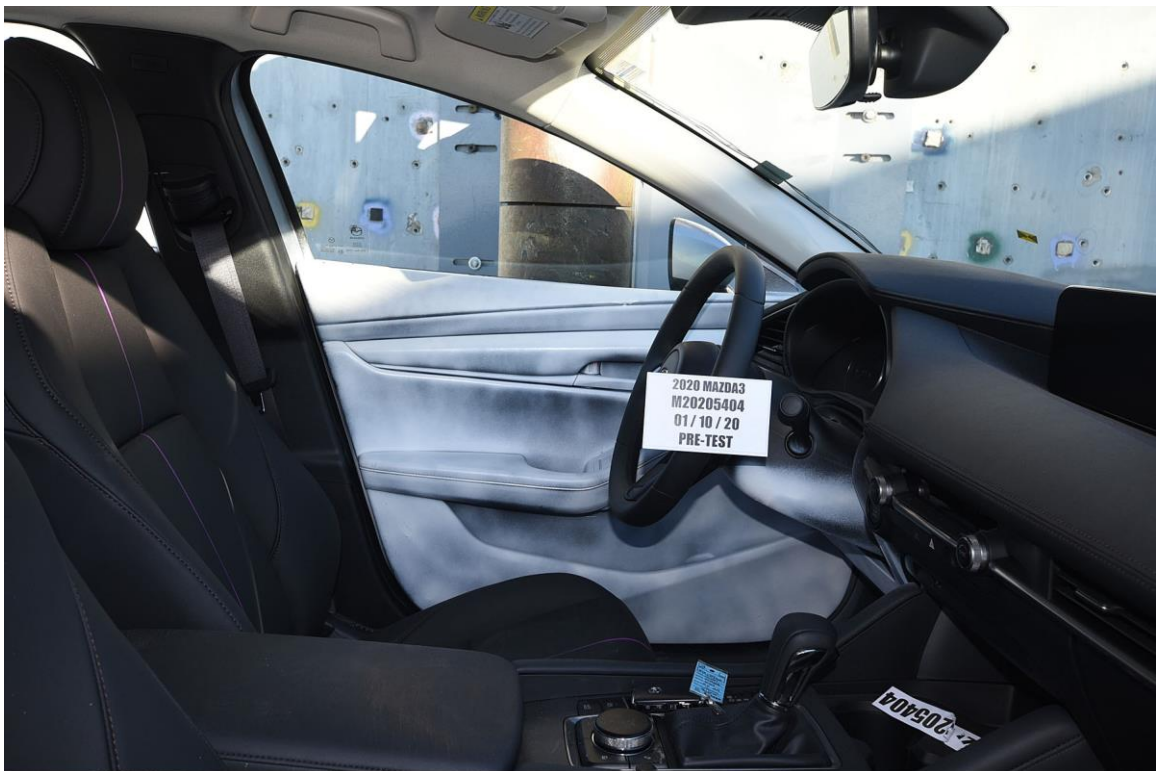
FIGURE 44. Pre-Test Inner Door Panel View
