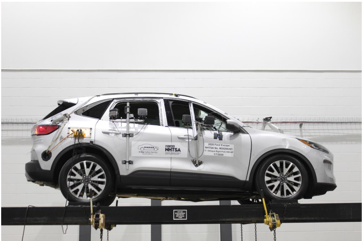
Figure A-67: FMVSS No. 301 Static Rollover 360 Degrees
