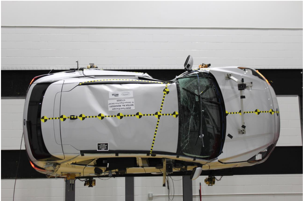
Figure A-66: FMVSS No. 301 Static Rollover 270 Degrees
