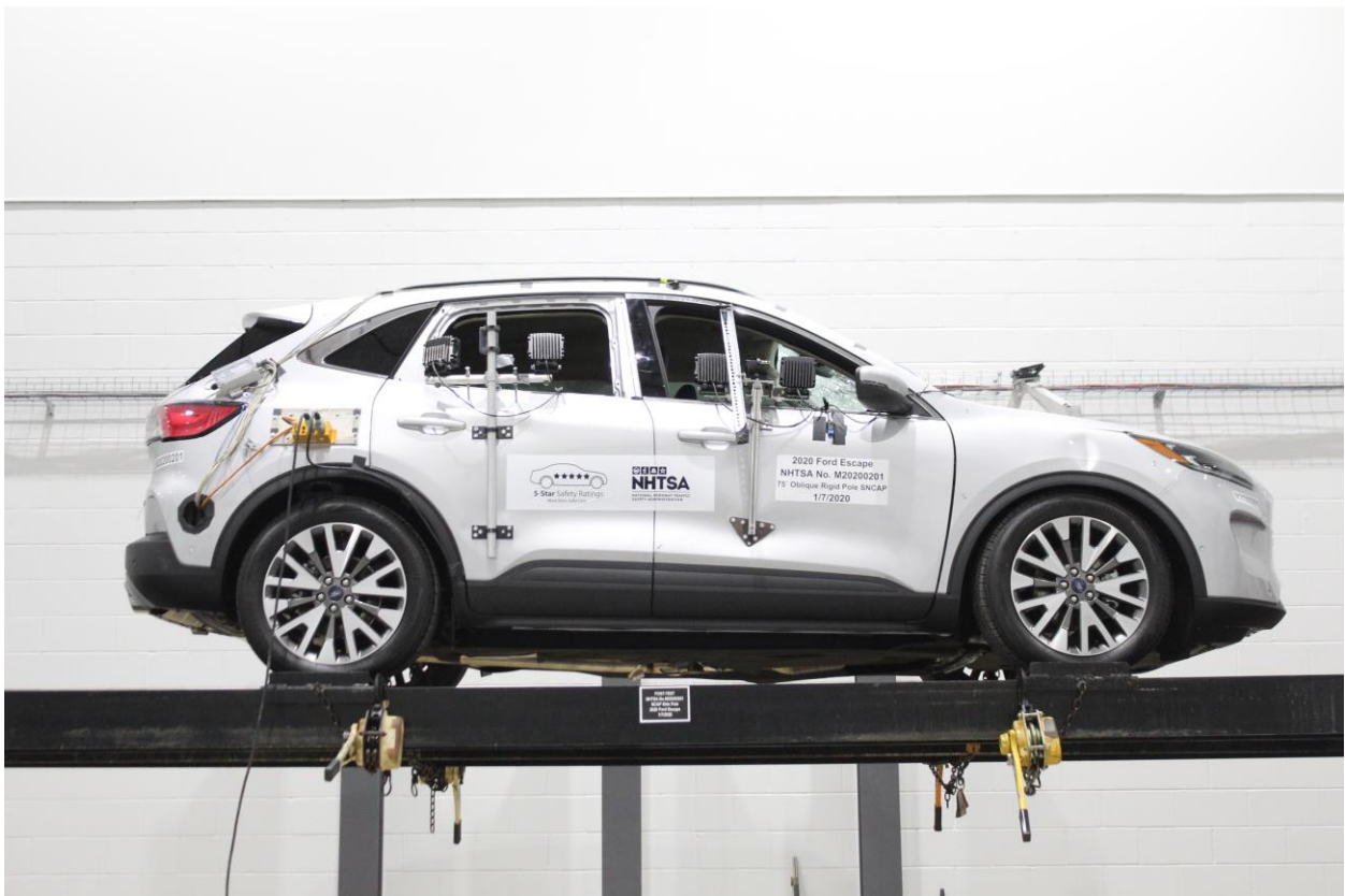
Figure A-63: FMVSS No. 301 Static Rollover 0 Degrees
