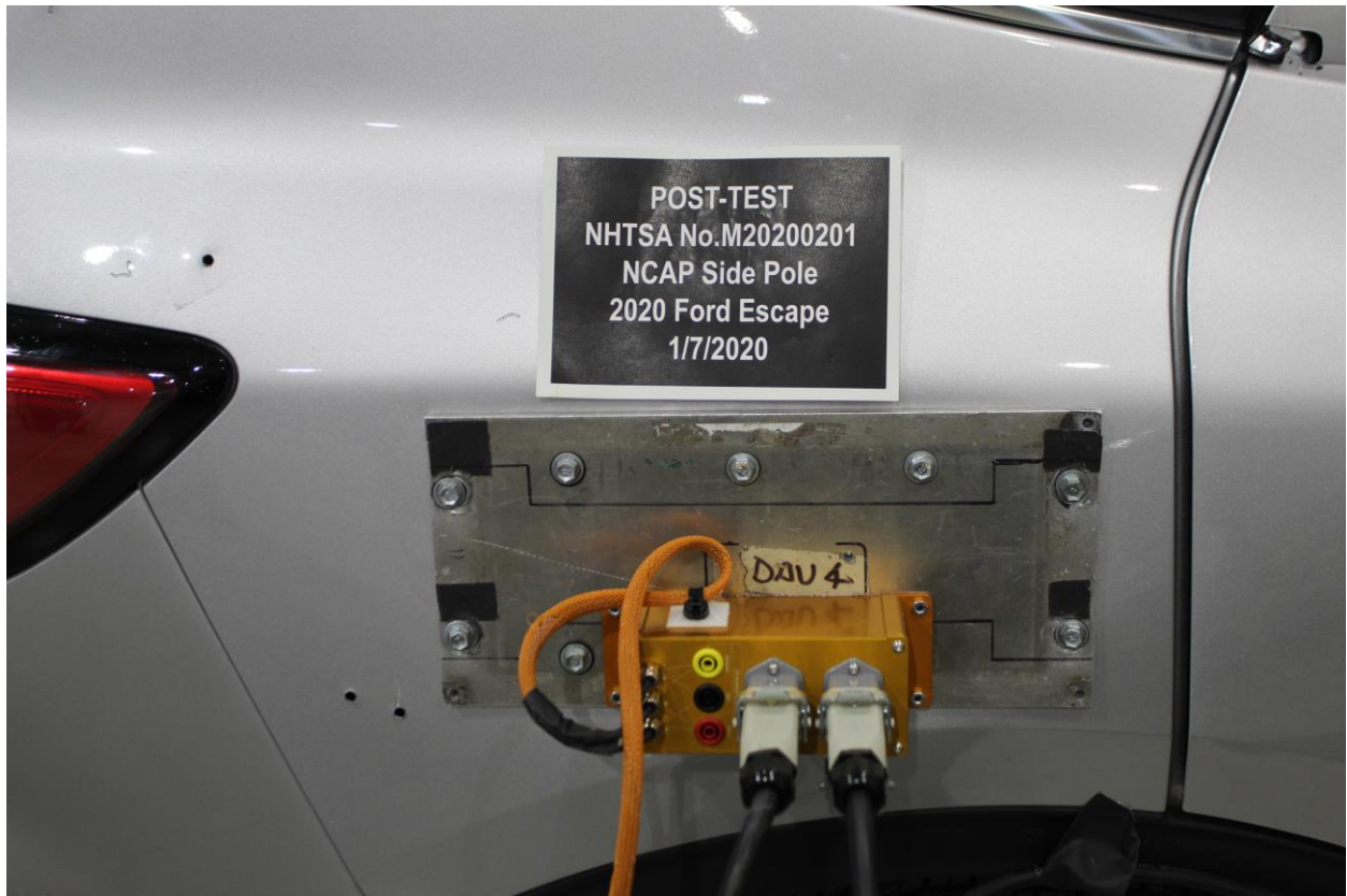
Figure A-21: Post-Impact View of Installed Test Interface Port
