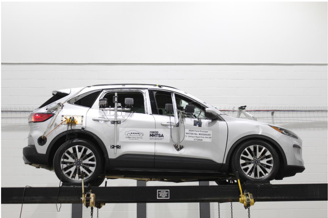
Figure A-26: FMVSS No. 305 Static Rollover 360 Degrees
