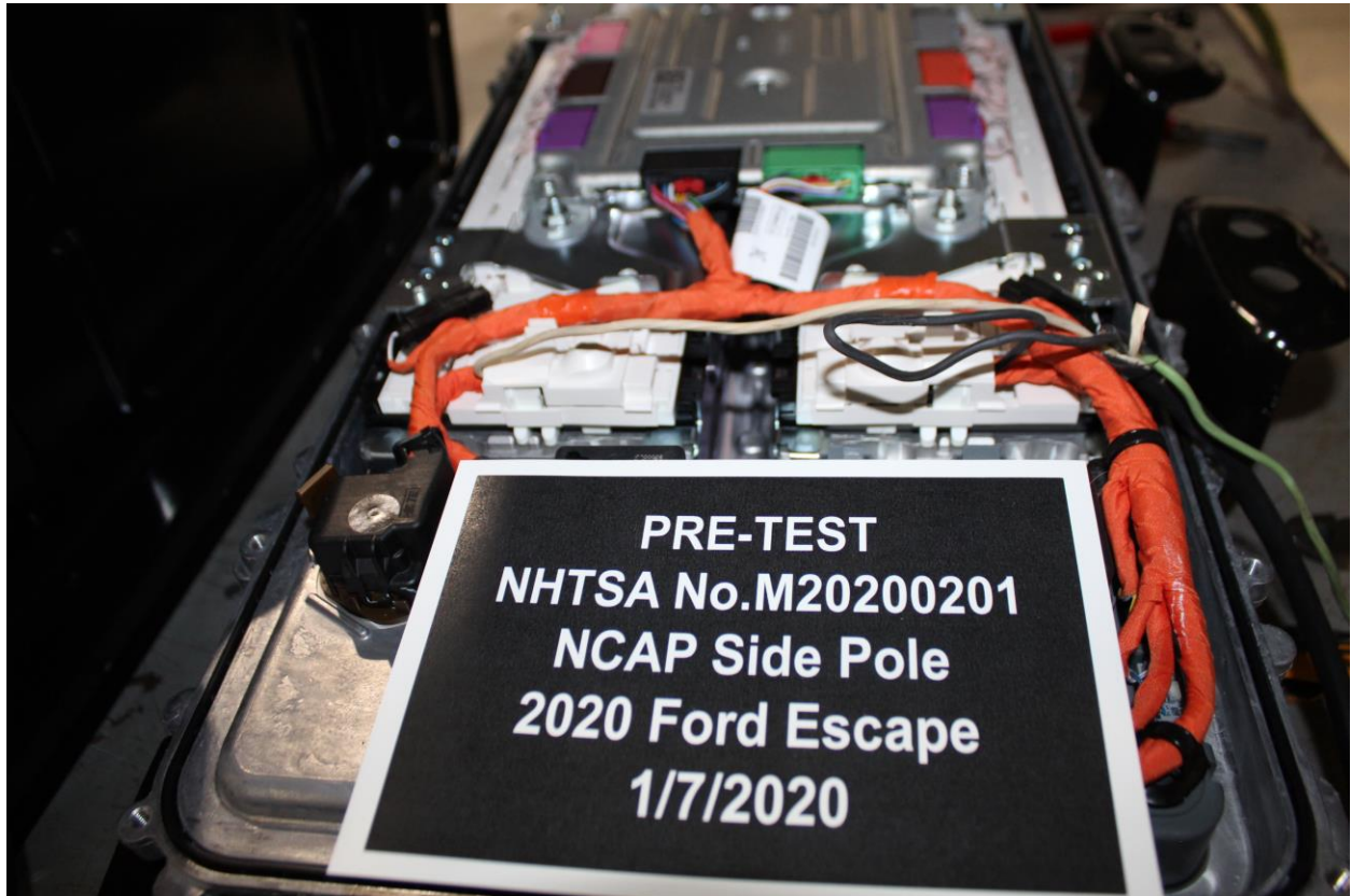
Figure A-17: Pre-Impact View of High Voltage Interconnects
