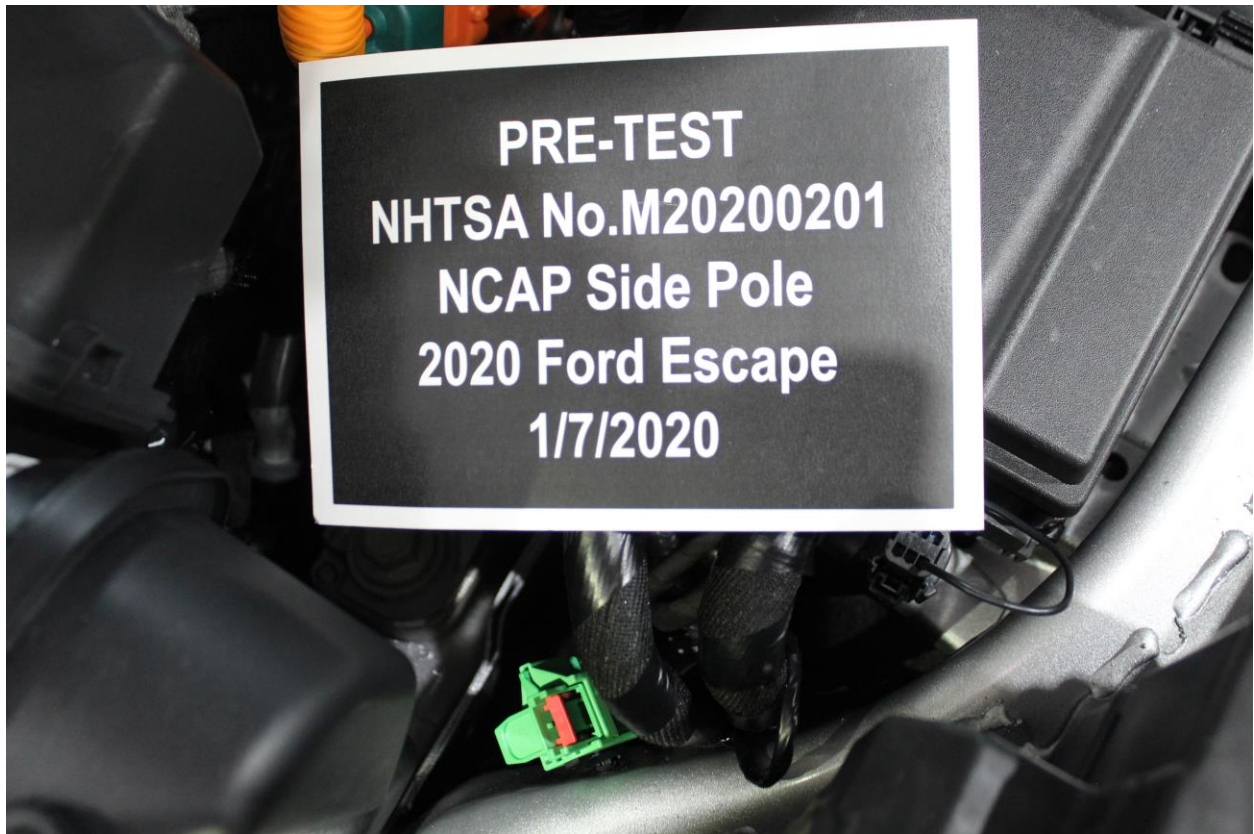
Figure A-5: Manual High Voltage Service Disconnect Location
