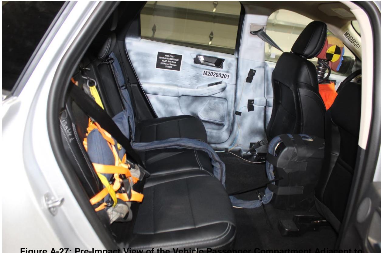
Figure A-27: Pre-Impact View of the Vehicle Passenger Compartment Adjacent to Propulsion Battery
