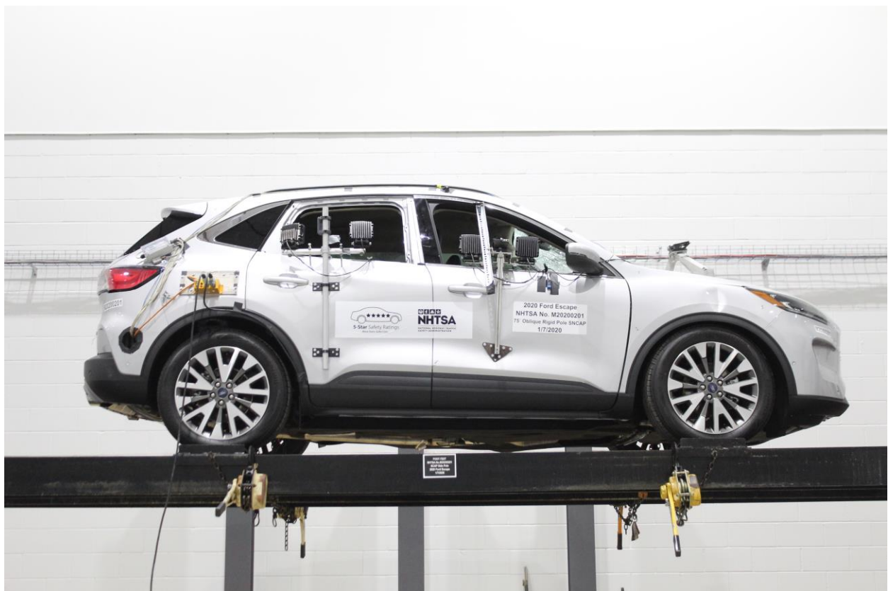
Figure A-22: FMVSS No. 305 Static Rollover 0 Degrees
