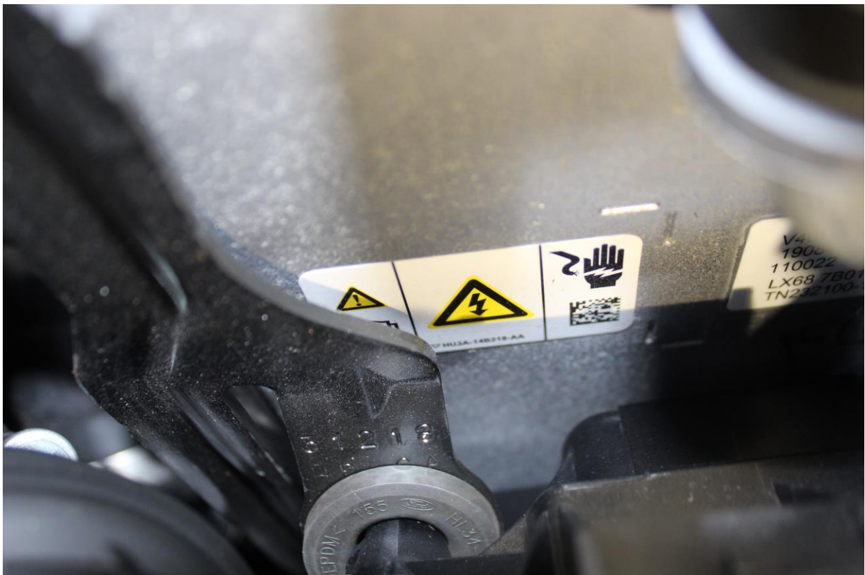
Figure A-2: Power Inverter Warning Label
