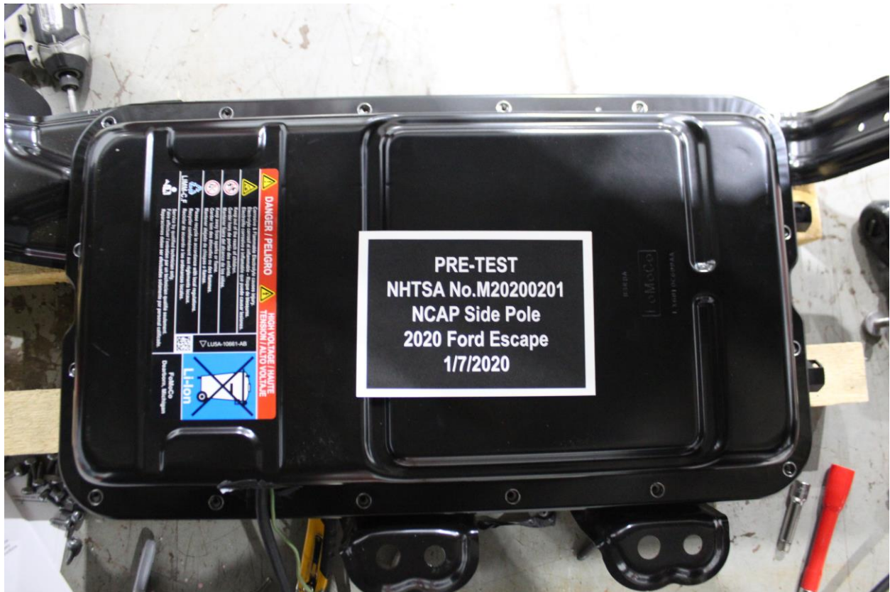
Figure A-11: Pre-Impact View of Battery Box(s) or Container(s) Which Holds Individual Battery Modules
