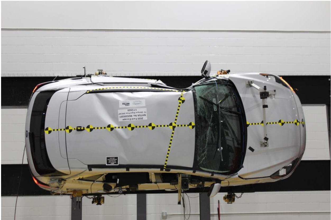
Figure A-25: FMVSS No. 305 Static Rollover 270 Degrees
