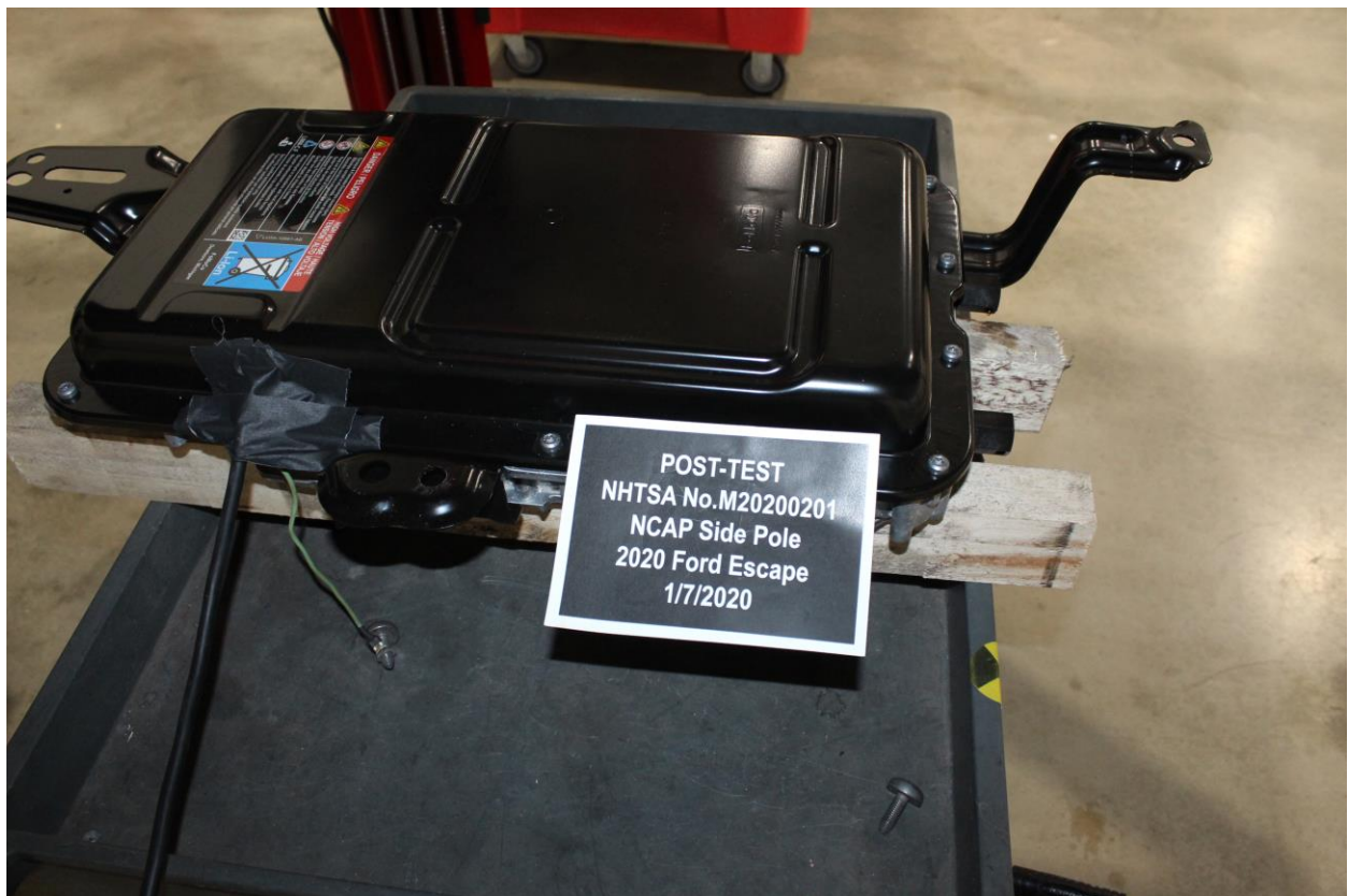
Figure A-12: Post-Impact View of Battery Box(s) or Container(s) Which Holds Individual Battery Modules
