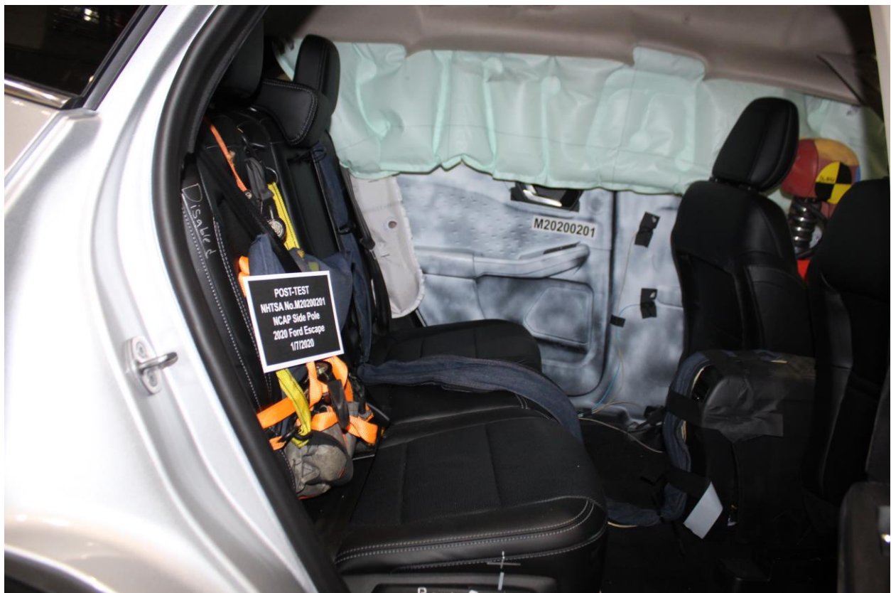
Figure A-28: Post-Impact View of the Vehicle Passenger Compartment Adjacent to Propulsion Battery
