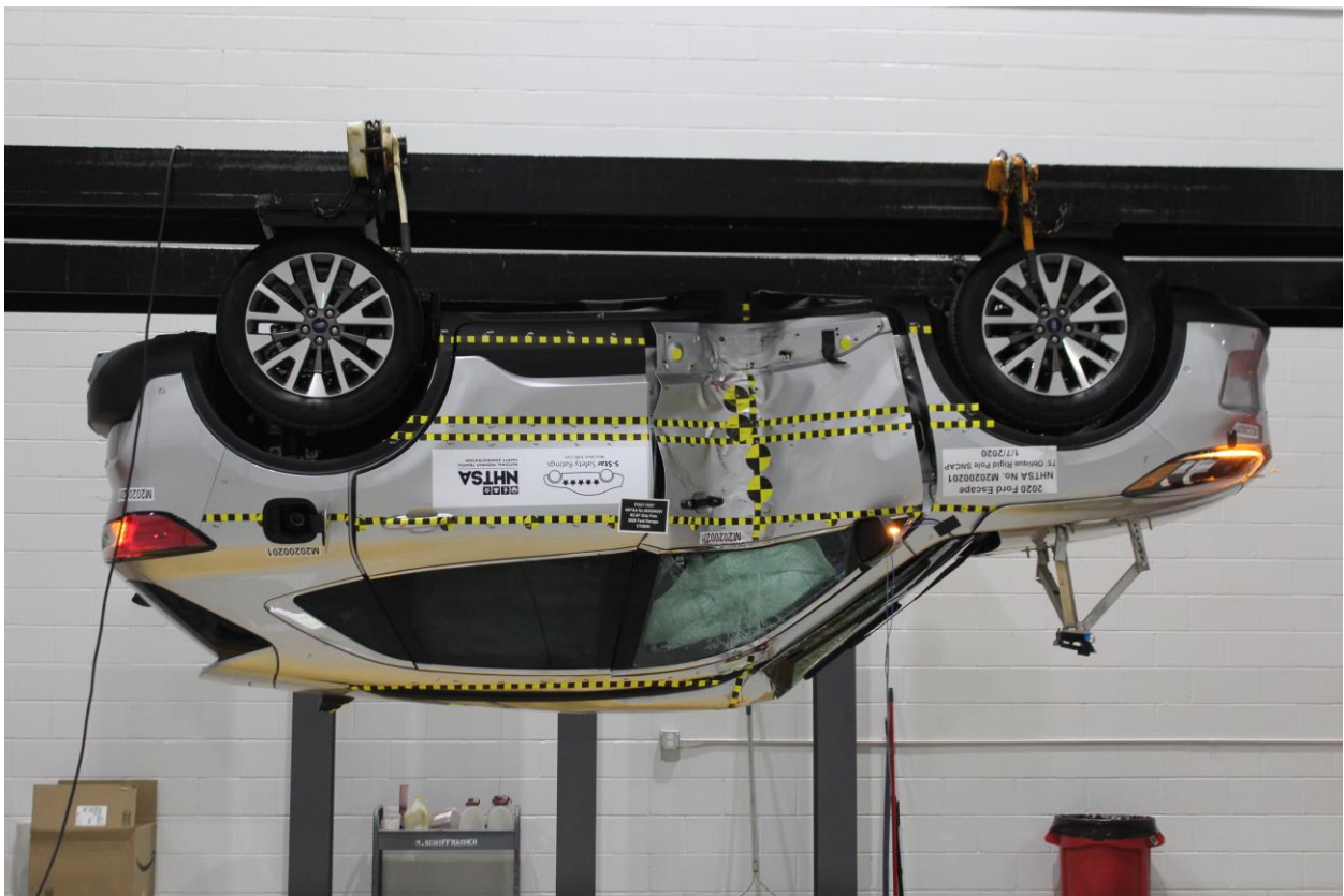
Figure A-24: FMVSS No. 305 Static Rollover 180 Degrees
