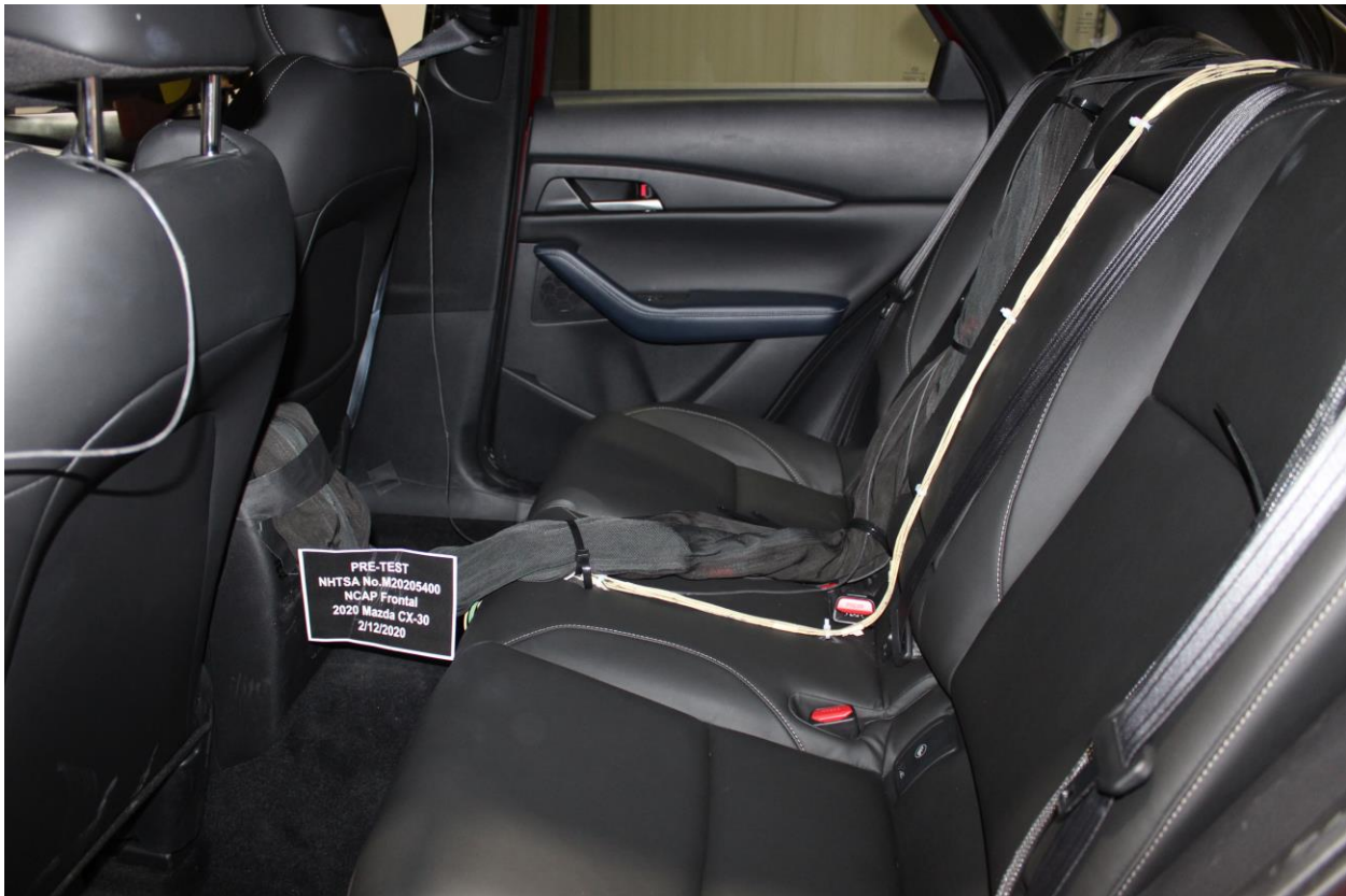
Figure A-28: Pre-Test Dummy Cable Routing
