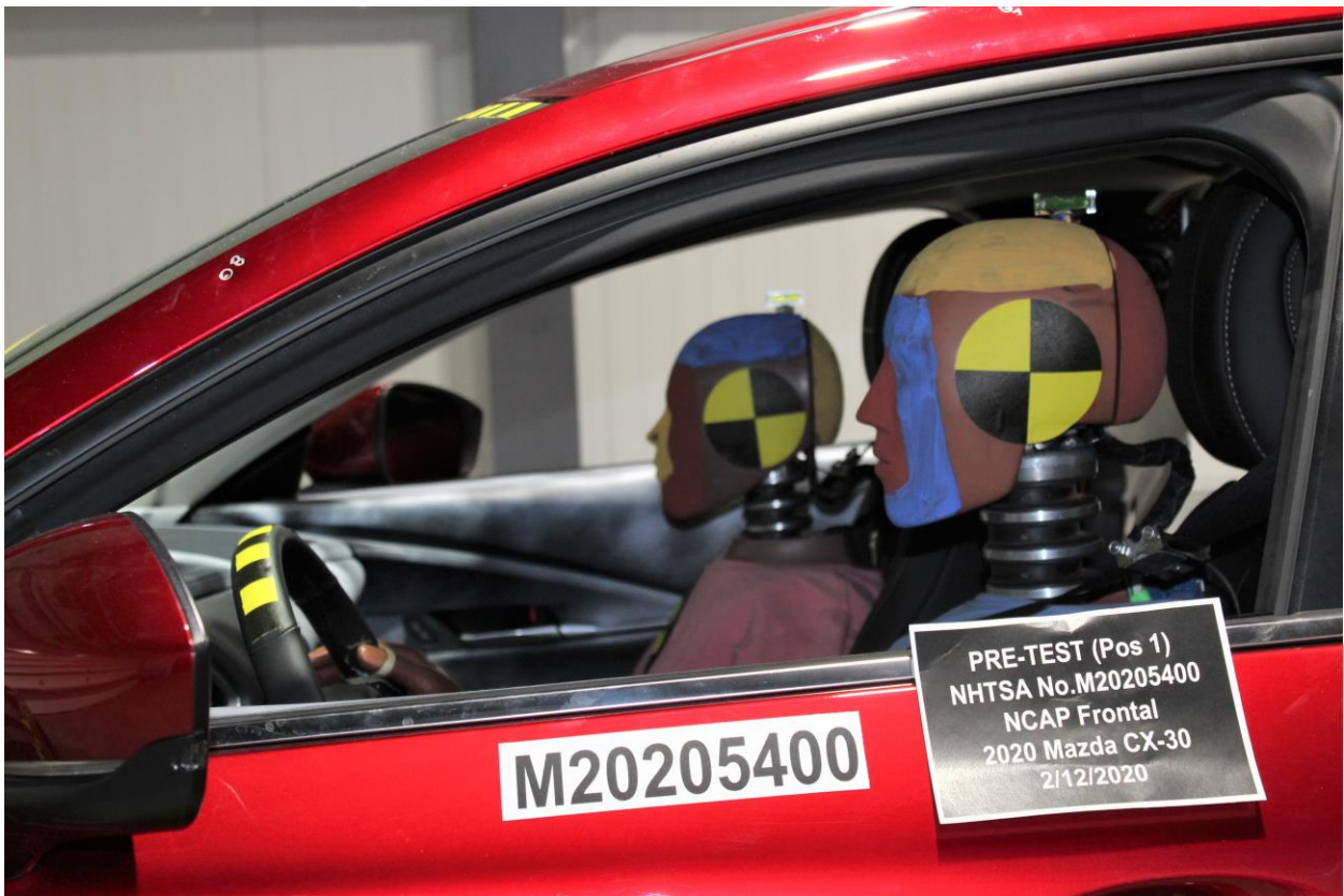
Figure A-32: Pre-Test Driver Dummy Window View
