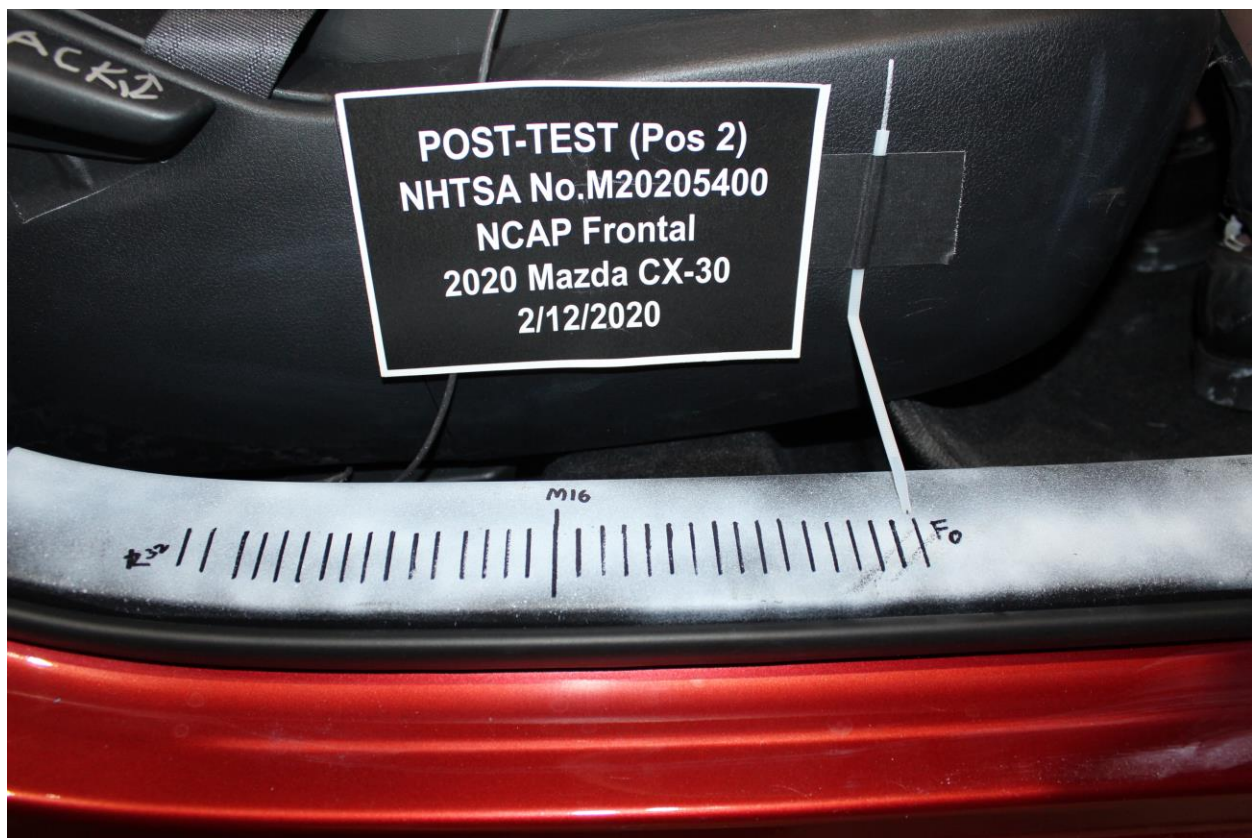
Figure A-60: Post-Test Passenger's Seat Fore-Aft Markings
