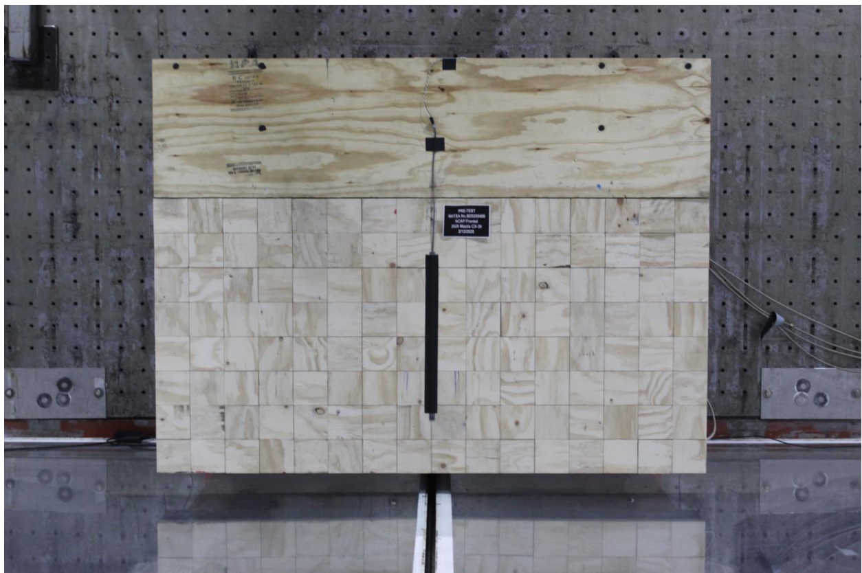
Figure A-2: Pre-Test Load Cell Wall
