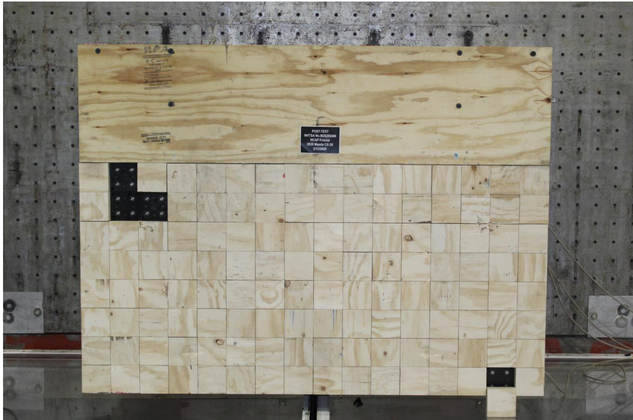
Figure A-3: Post-Test Load Cell Wall
