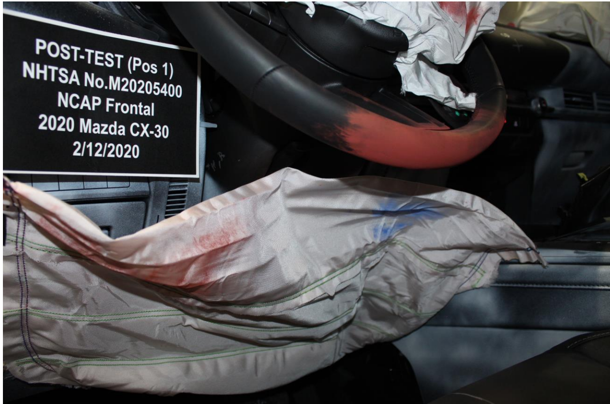
Figure A-45: Post-Test Driver's Side Knee Bolster
