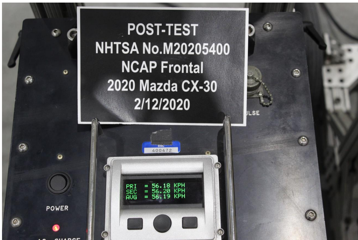
Figure A-76: Post-Test Speed Trap Read-Out
