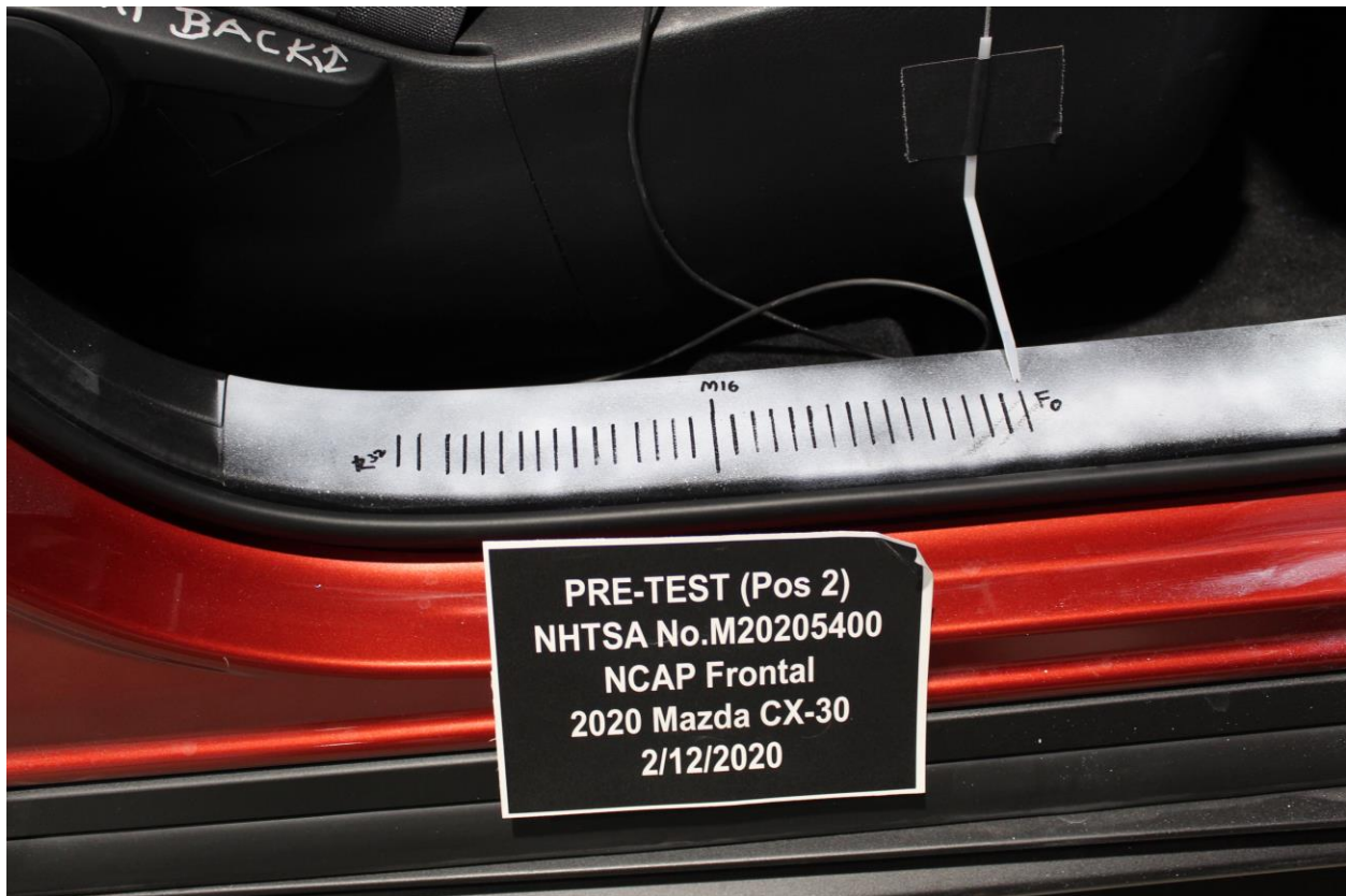
Figure A-59: Pre-Test Passenger's Seat Fore-Aft Markings
