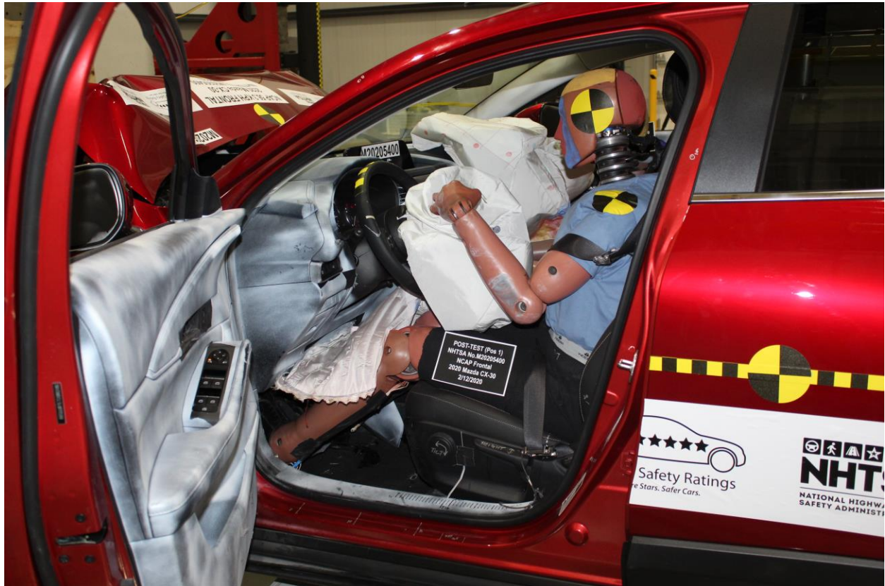
Figure A-35: Post-Test Driver Dummy and Vehicle Interior View
