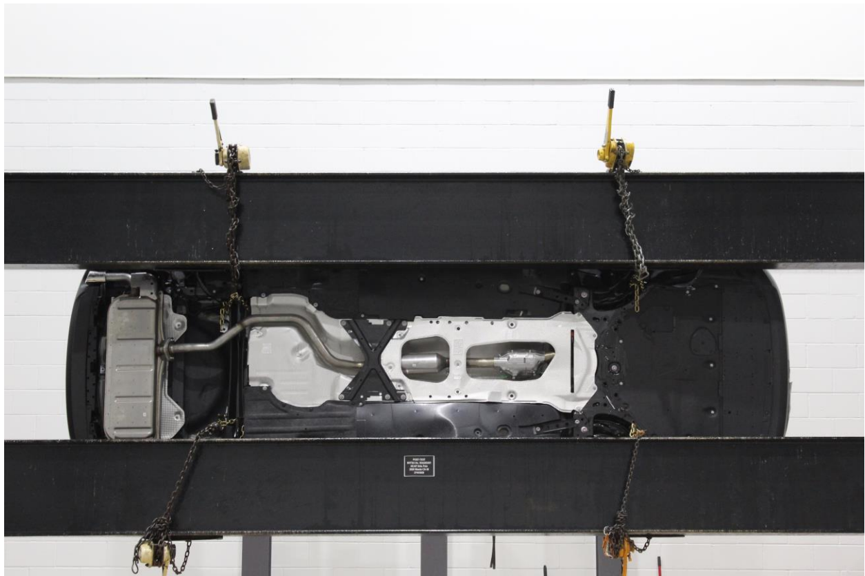
Figure A-64: FMVSS No. 301 Static Rollover 90 Degrees
