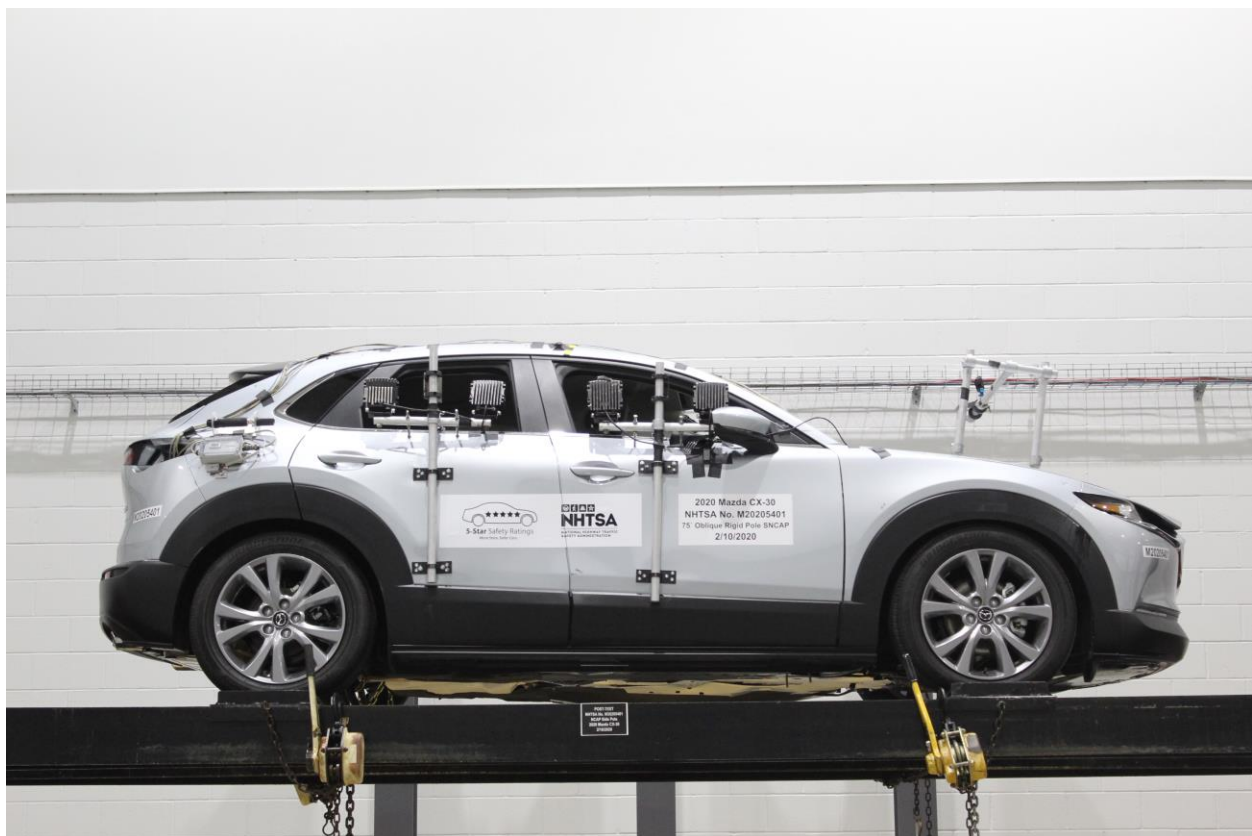
Figure A-67: FMVSS No. 301 Static Rollover 360 Degrees
