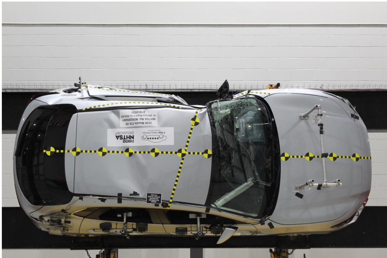
Figure A-66: FMVSS No. 301 Static Rollover 270 Degrees
