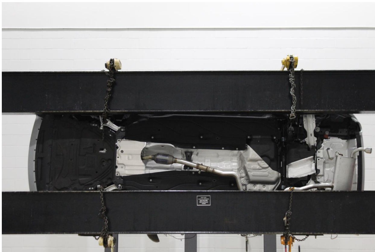
Figure A-97: FMVSS No. 301 Static Rollover 90 Degrees
