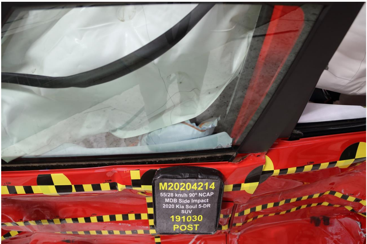
043 Post-Test Driver Dummy and Door Clearance View
