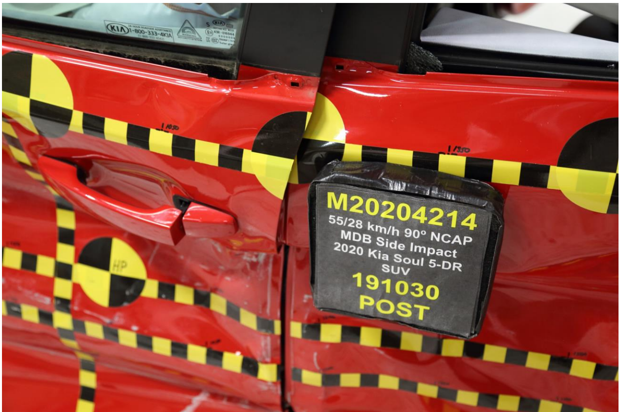
022 Post-Test Left Front Door Latch Close-Up
