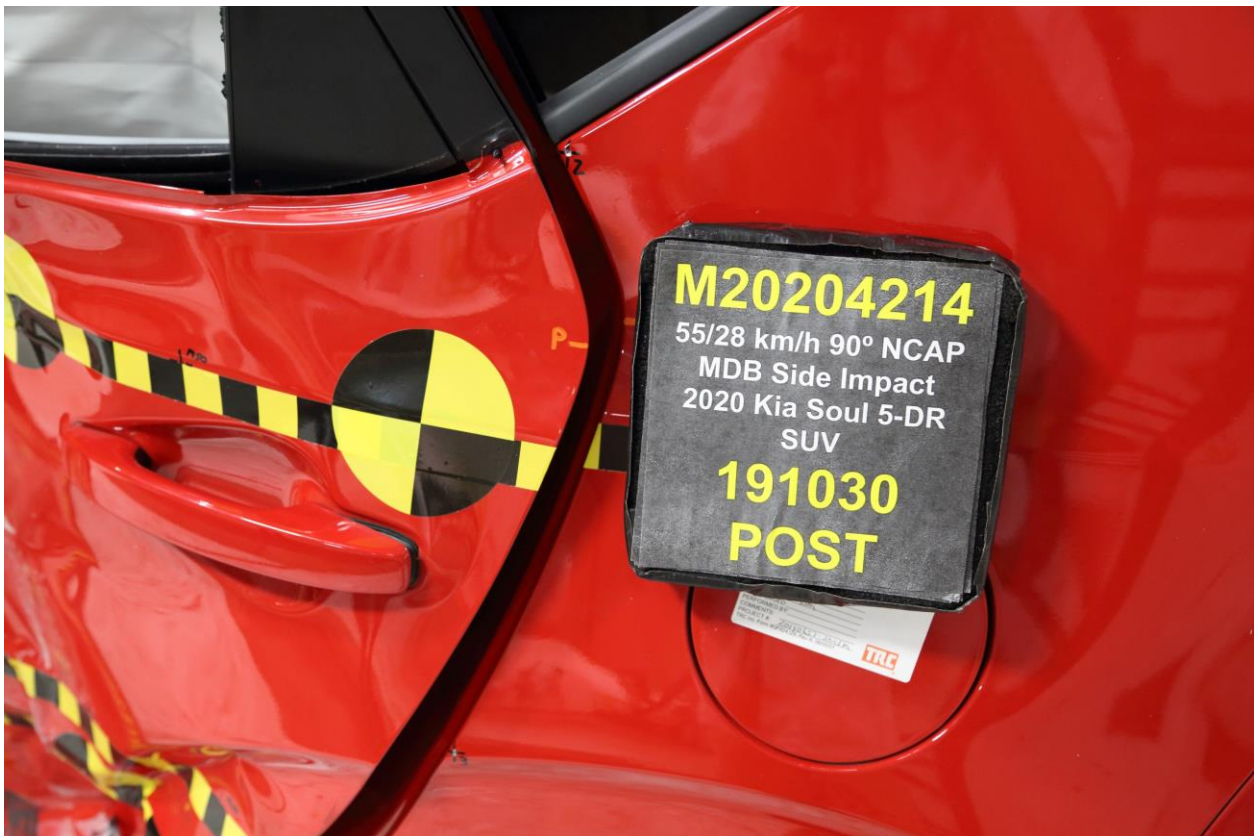
024 Post-Test Left Rear Door Latch Close-Up
