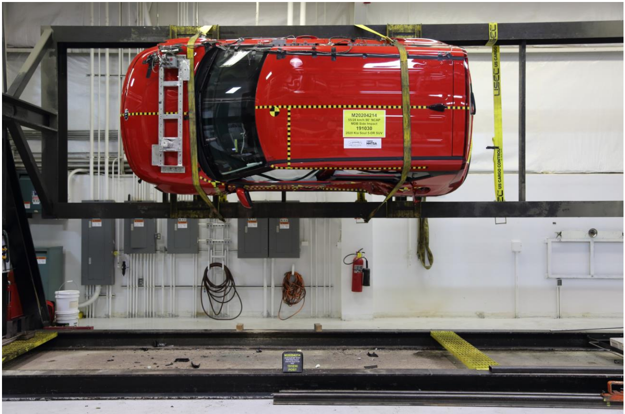
097 FMVSS No. 301 Static Rollover 90 Degrees
