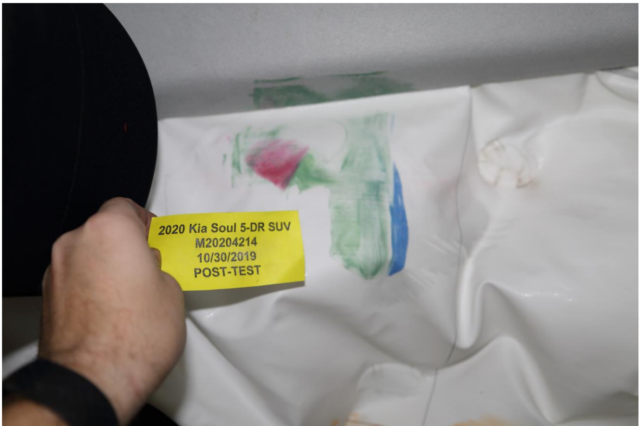
048 Post-Test Driver Dummy Close-Up Head Contact with Vehicle View
