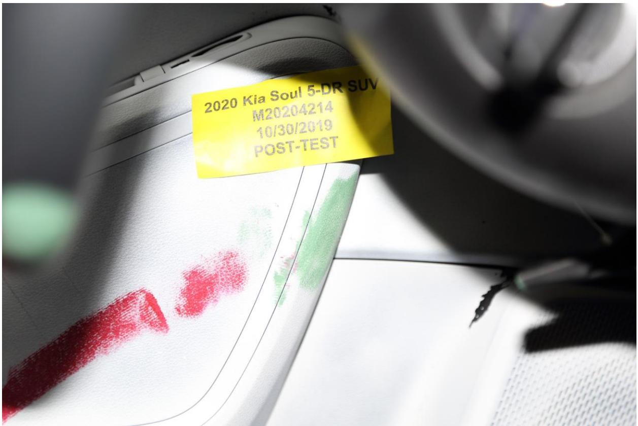
054 Post-Test Driver Dummy Close-Up Knee Contact View
