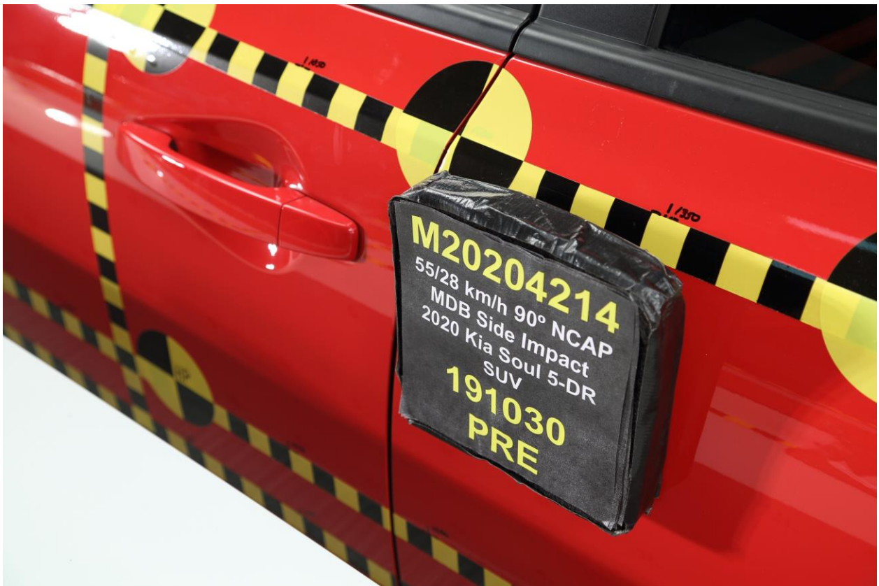
021 Pre-Test Left Front Door Latch Close-Up
