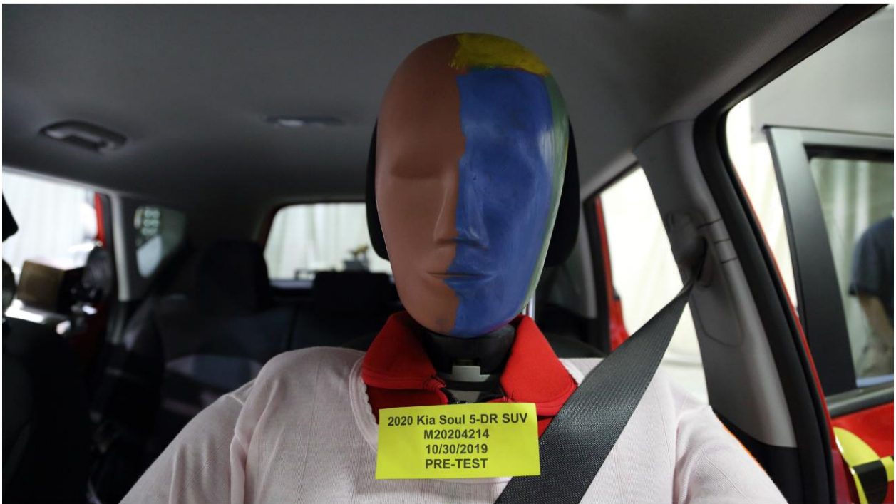
031 Pre-Test Frontal View of Driver Dummy Head and Shoulders in Relation to Head Restraint
