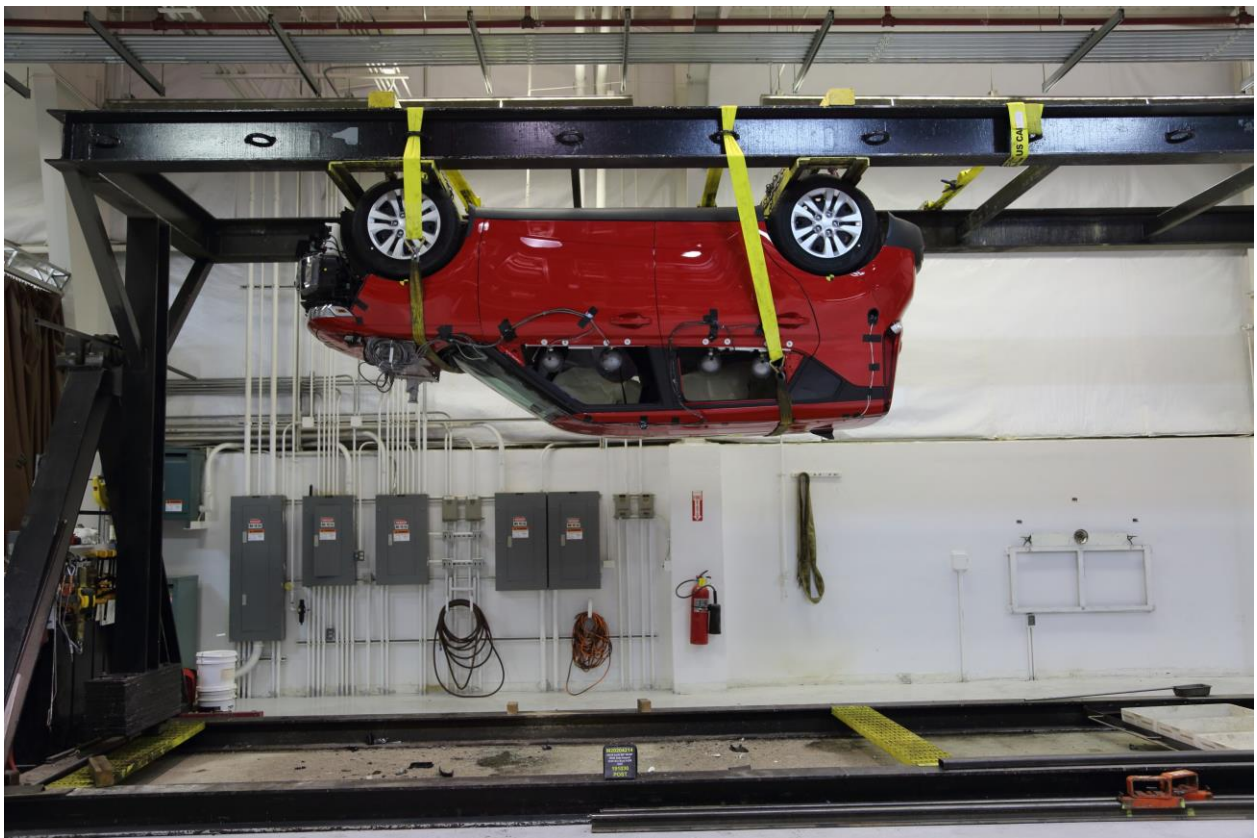
098 FMVSS No. 301 Static Rollover 180 Degrees
