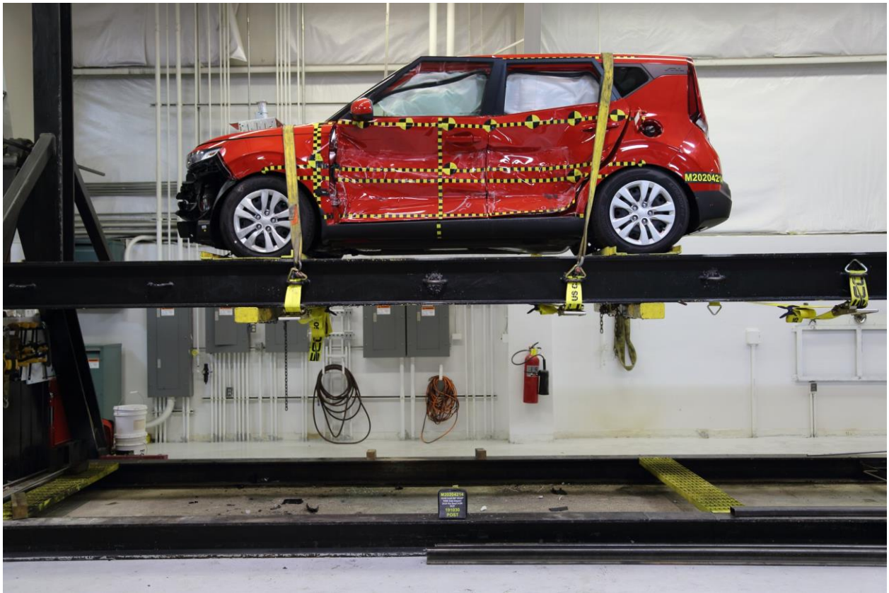
096 FMVSS No. 301 Static Rollover 0 Degrees
