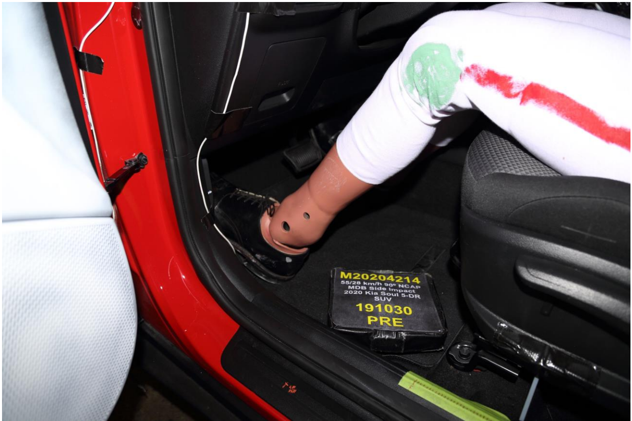
034 Pre-Test Placement of Driver's Dummy Feet
