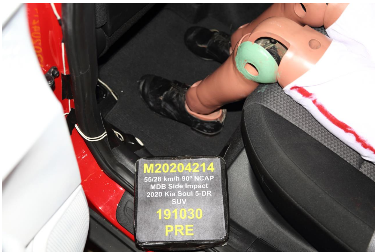
064 Pre-Test Placement of Rear Passenger Dummy's Feet
