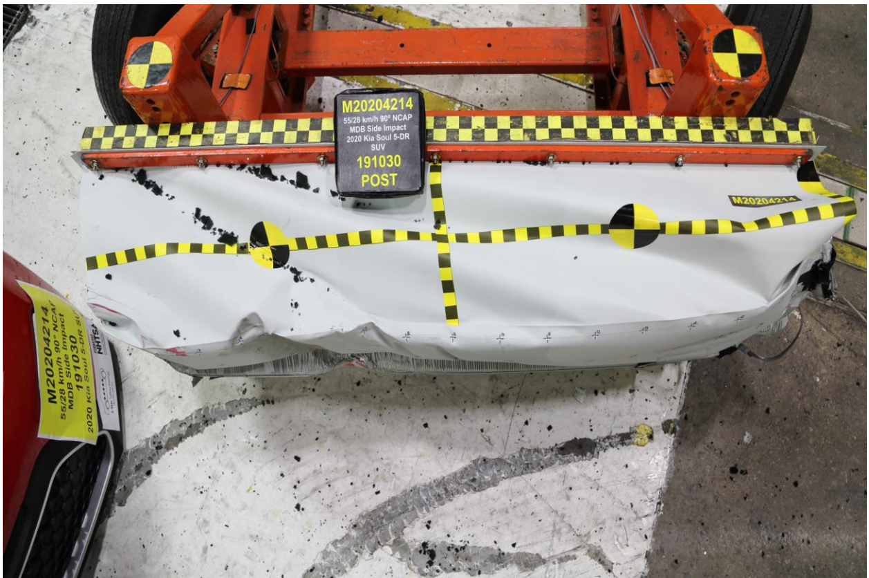
087 Post-Test Top View of MDB Impactor Face
