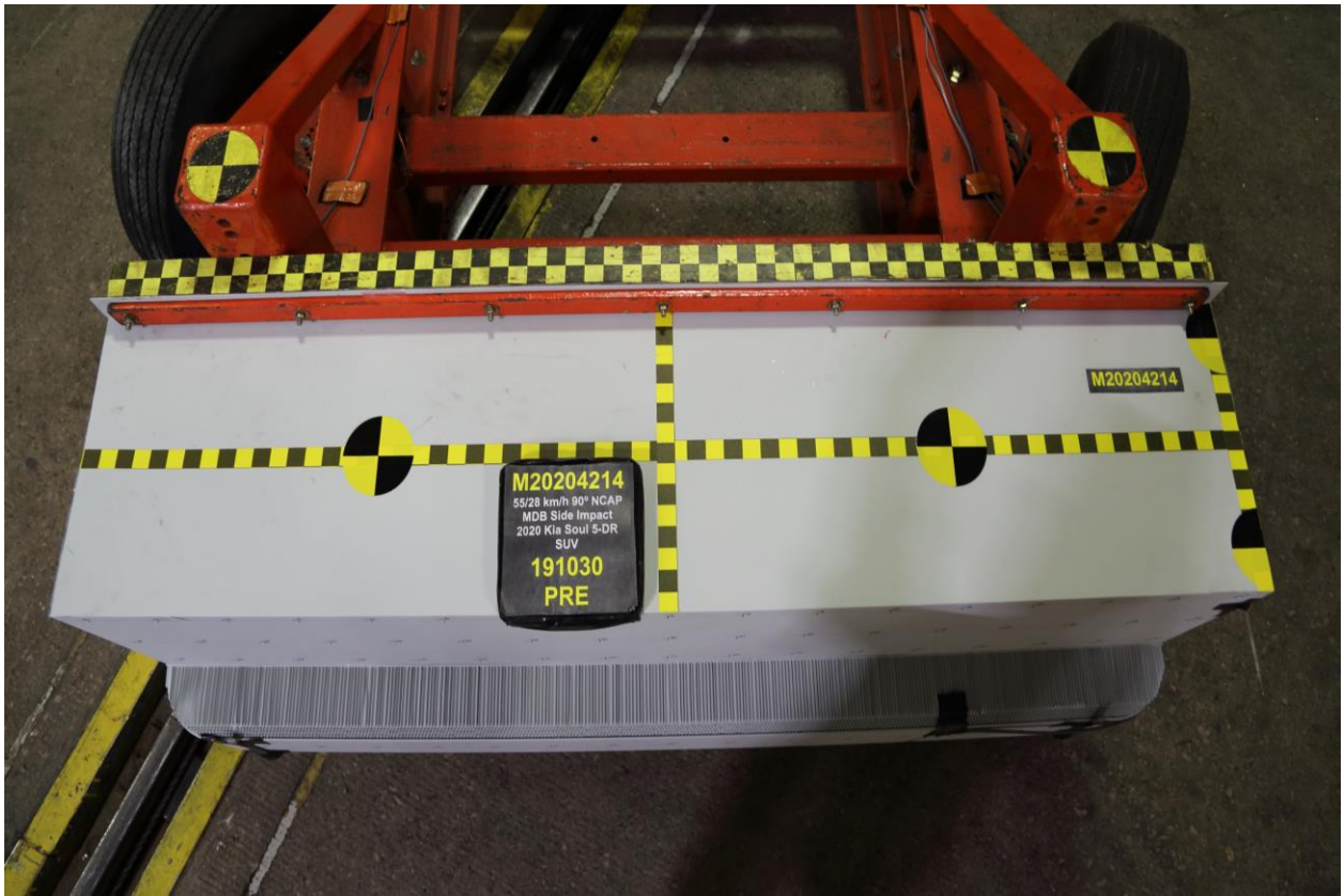
086 Pre-Test Top View of MDB Impactor Face
