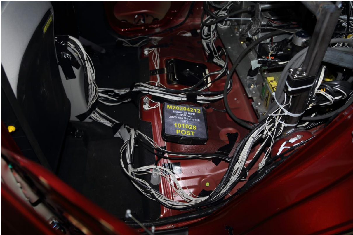
029 Post-Test Dummy Cable Routing
