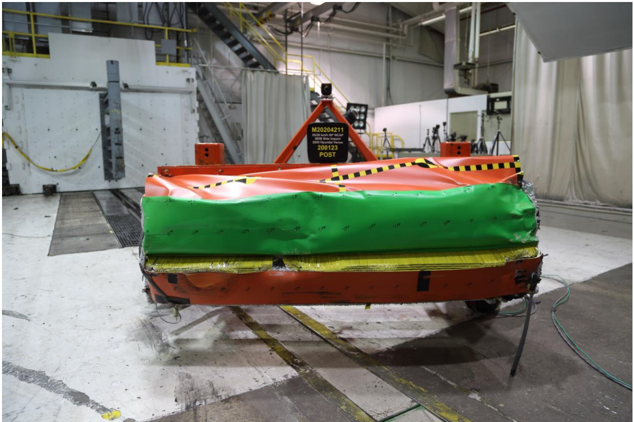
085 Post-Test Front View of MDB Impactor Face
