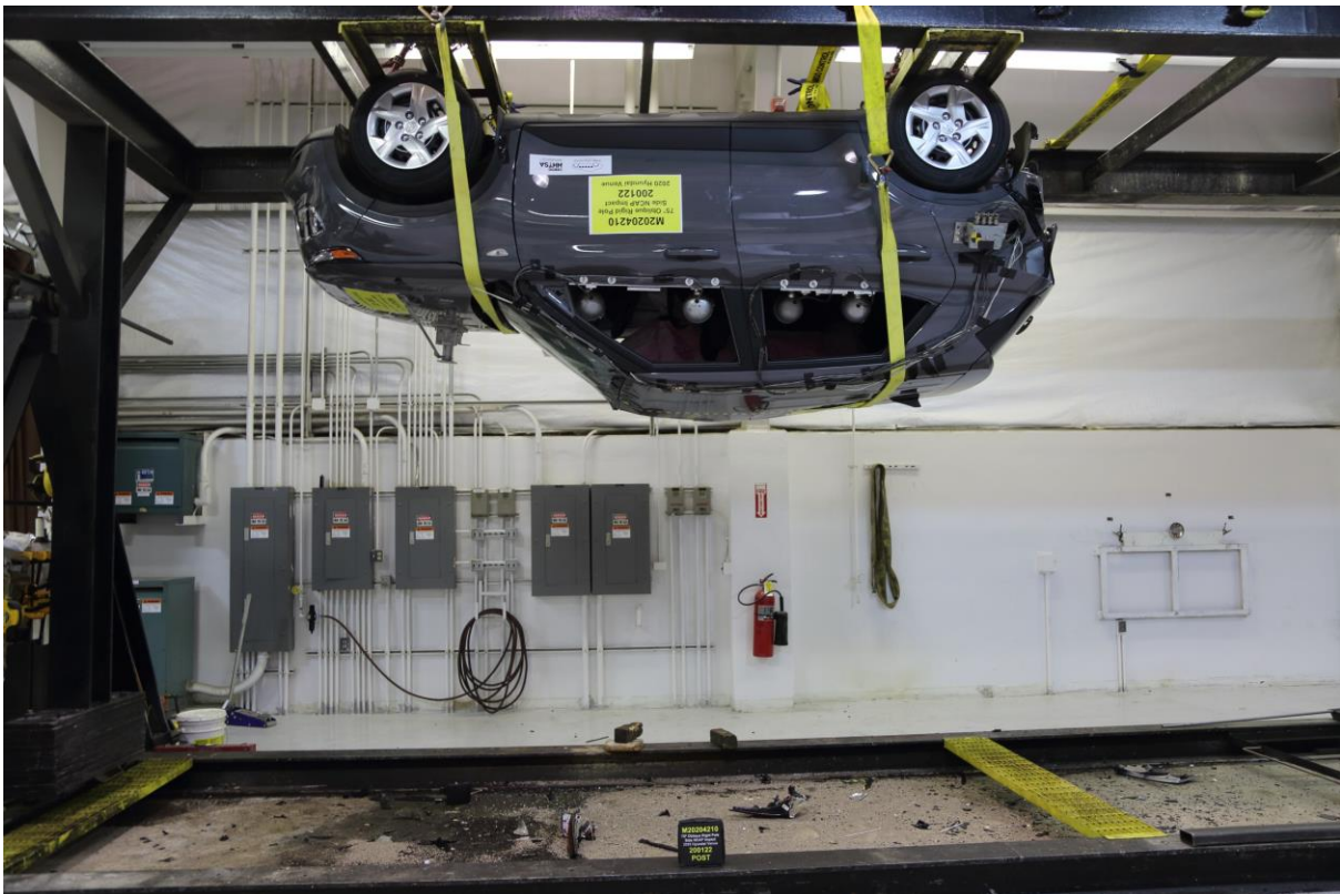
No. 065 FMVSS No. 301 Static Rollover 180 Degrees
