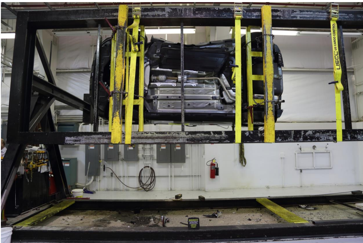
No. 066 FMVSS No. 301 Static Rollover 270 Degrees
