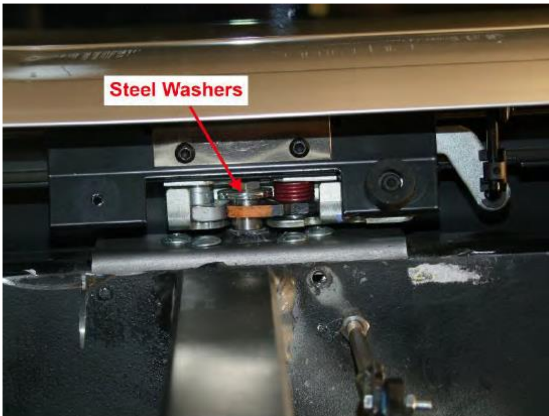
Figure 15 MCI modification A1 with window latched. (The tip of the detent lever is painted orange.) (Fig. 5.21 of reference 1)
