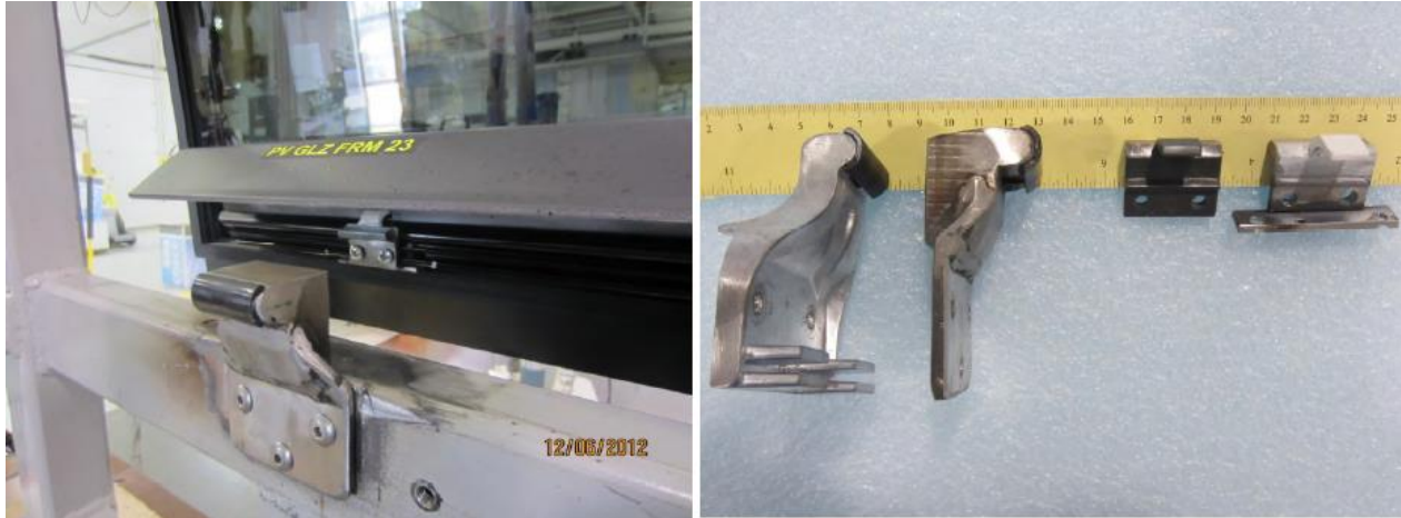
Figure 16 Prevost striker post and locator tab countermeasures (Fig. 8.4 of reference 1)
