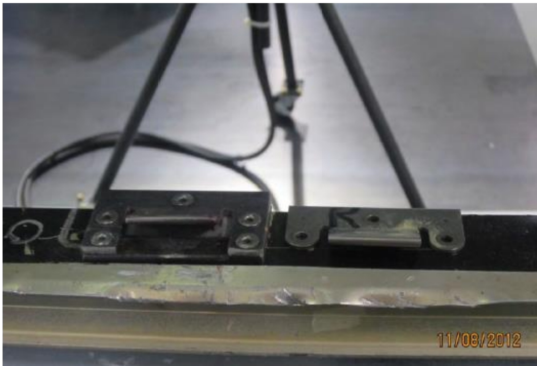
Figure 17 Van Hool modified spring clip (L) versus production spring clip (R) (Fig. 8.1 of reference 1)
