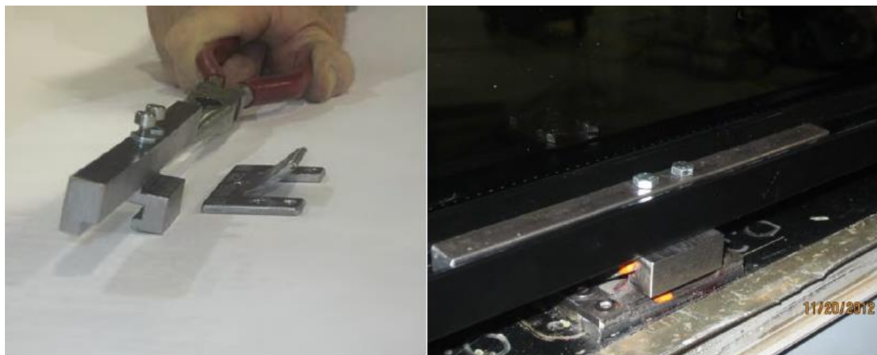
Figure 18 Van Hool latch countermeasure system (Fig. 8.2 of reference 1)
