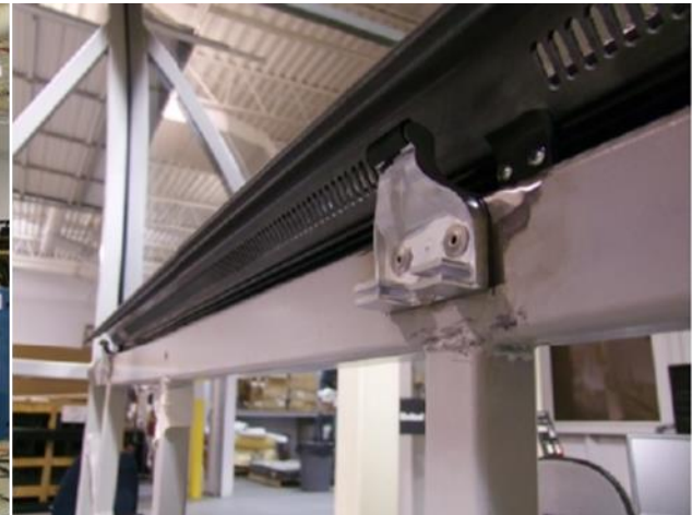
Figure 9 Prevost H3-45 test frame and latching mechanism (Fig. 5.5 and Fig. 5.6 of reference 1)
