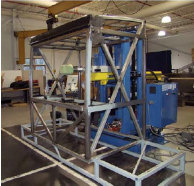
Figure 8 MCI E/J-series test frame and latching mechanism (latch bar not shown) (Fig. 5.1 and Fig. 5.3 of reference 1)
