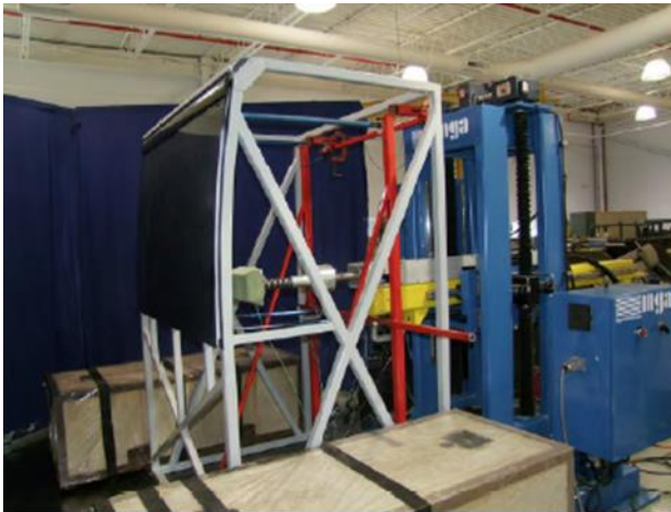
Figure 9 Prevost H3-45 test frame and latching mechanism (Fig. 5.5 and Fig. 5.6 of reference 1)
