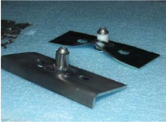
Figure 14 MCI E/J-series latch plate modification “A” shown in foreground (Fig. 5.19 of reference 1)
