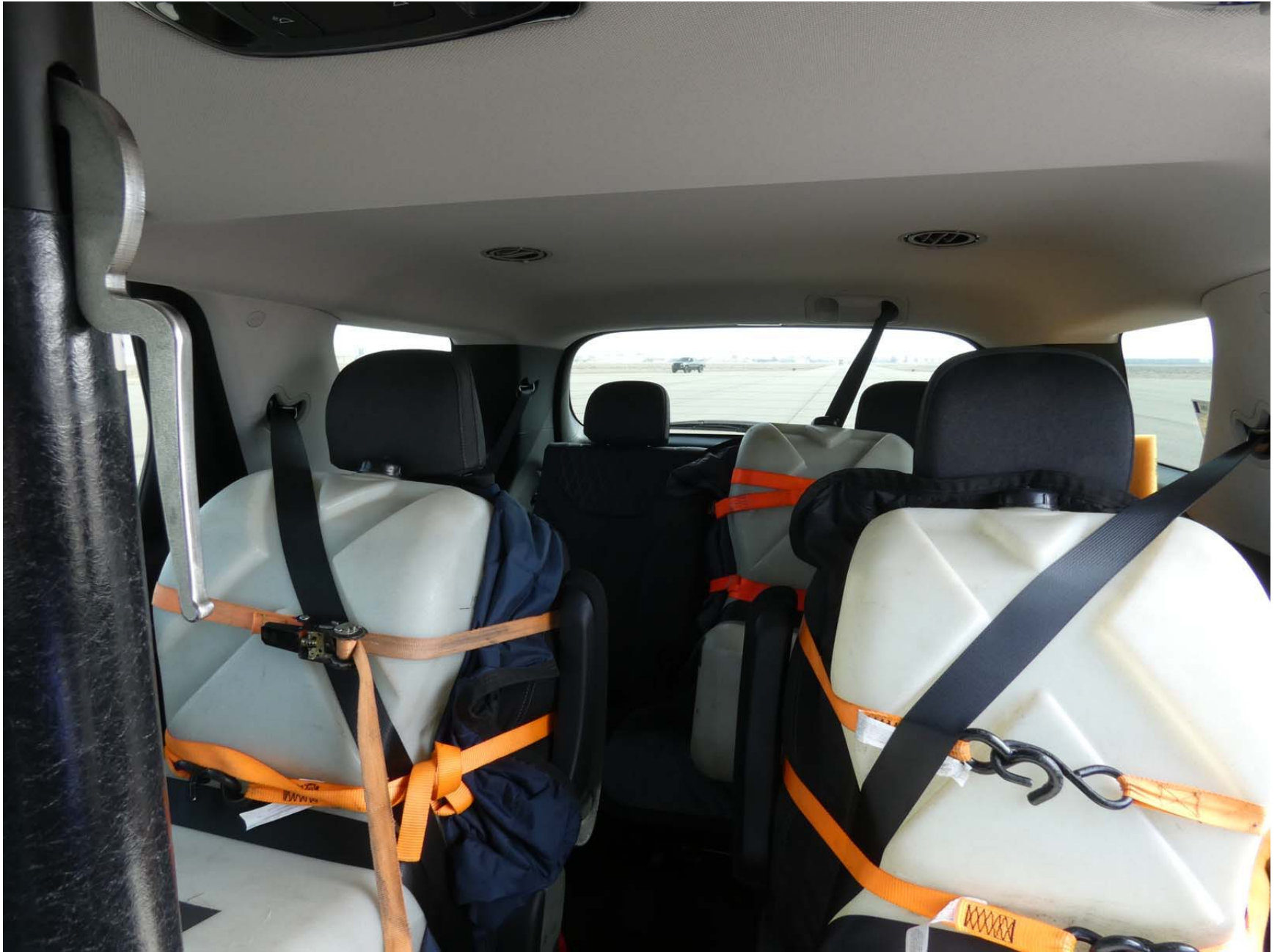
Figure A10. Ballast Condition
