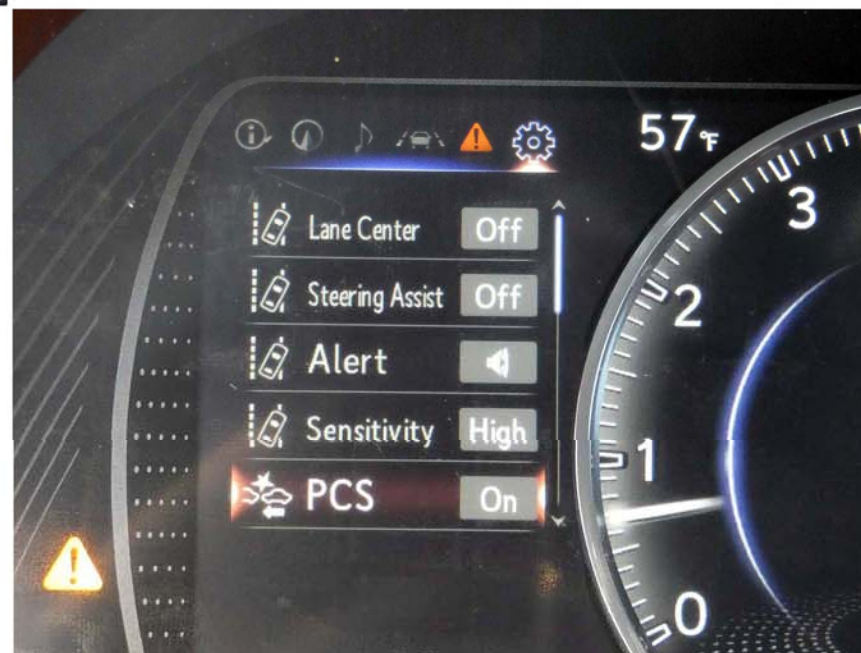
Figure A12. FCW System Setting Menus
