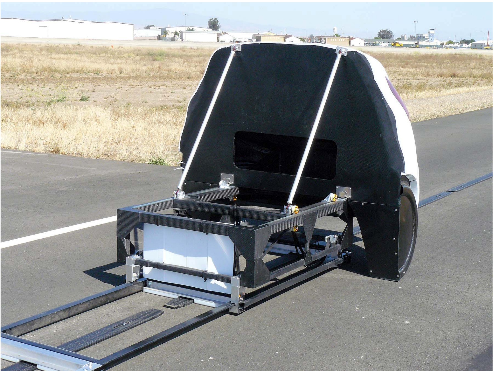
Figure A7. Load Frame/Slider of SSV
