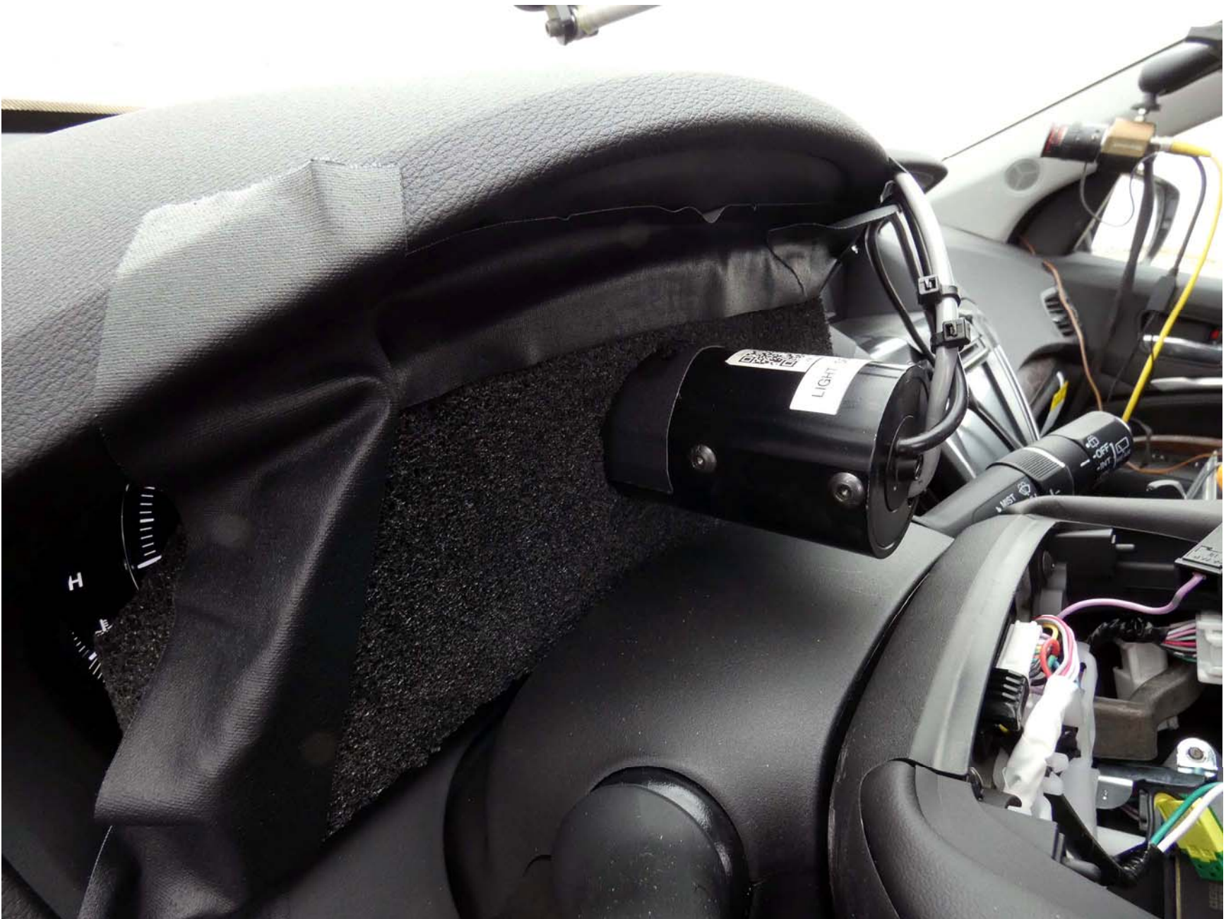
Figure A11. Sensor for Detecting Visual Alerts
