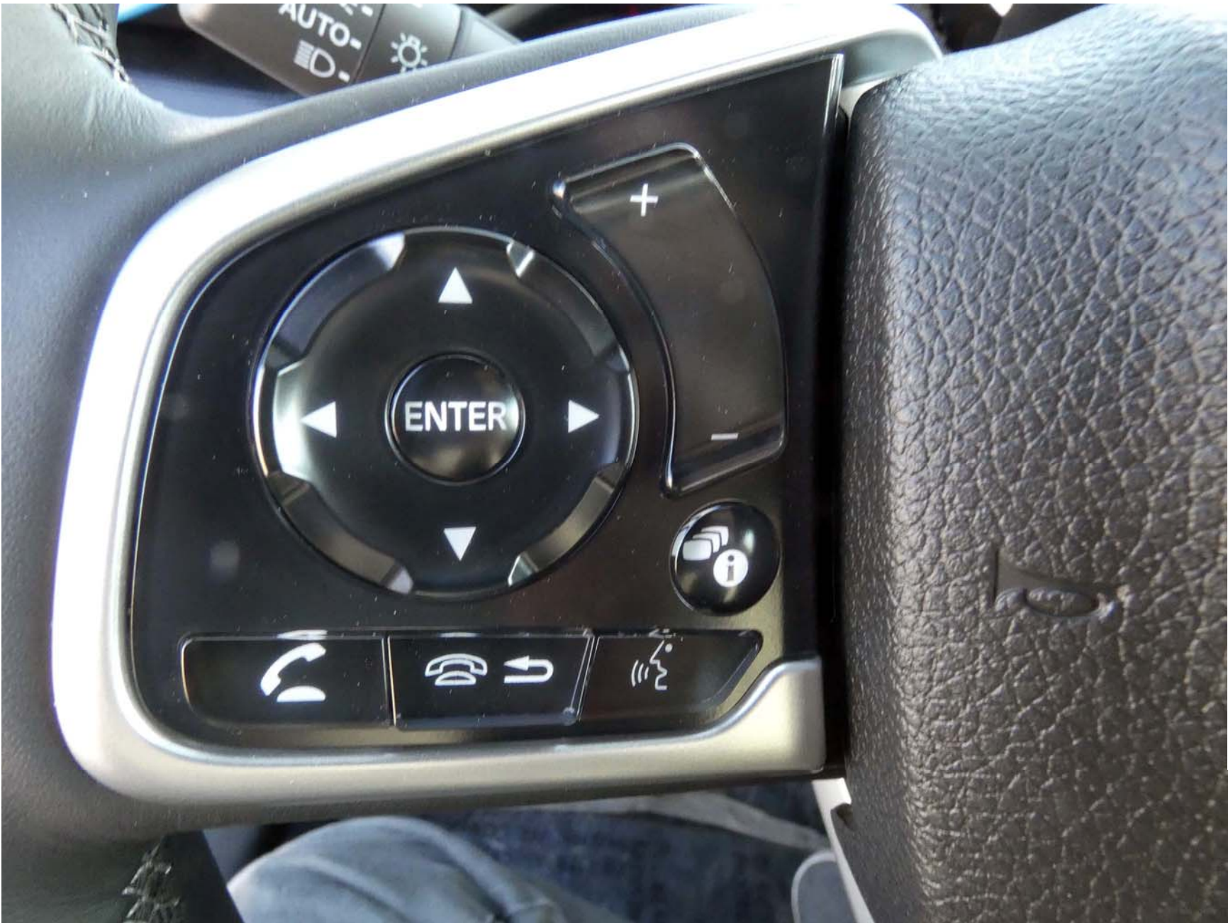
Figure A10. Controls for Interacting with RDM (LDW) Settings
