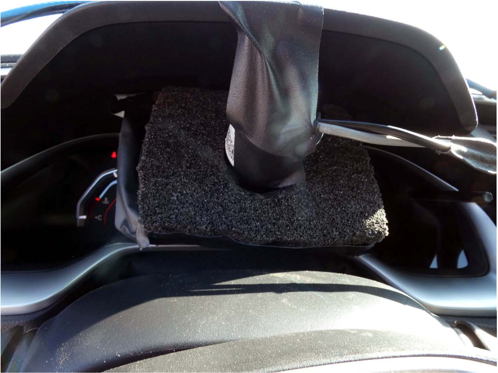
Figure A7. Sensor for Detecting Visual Alerts
