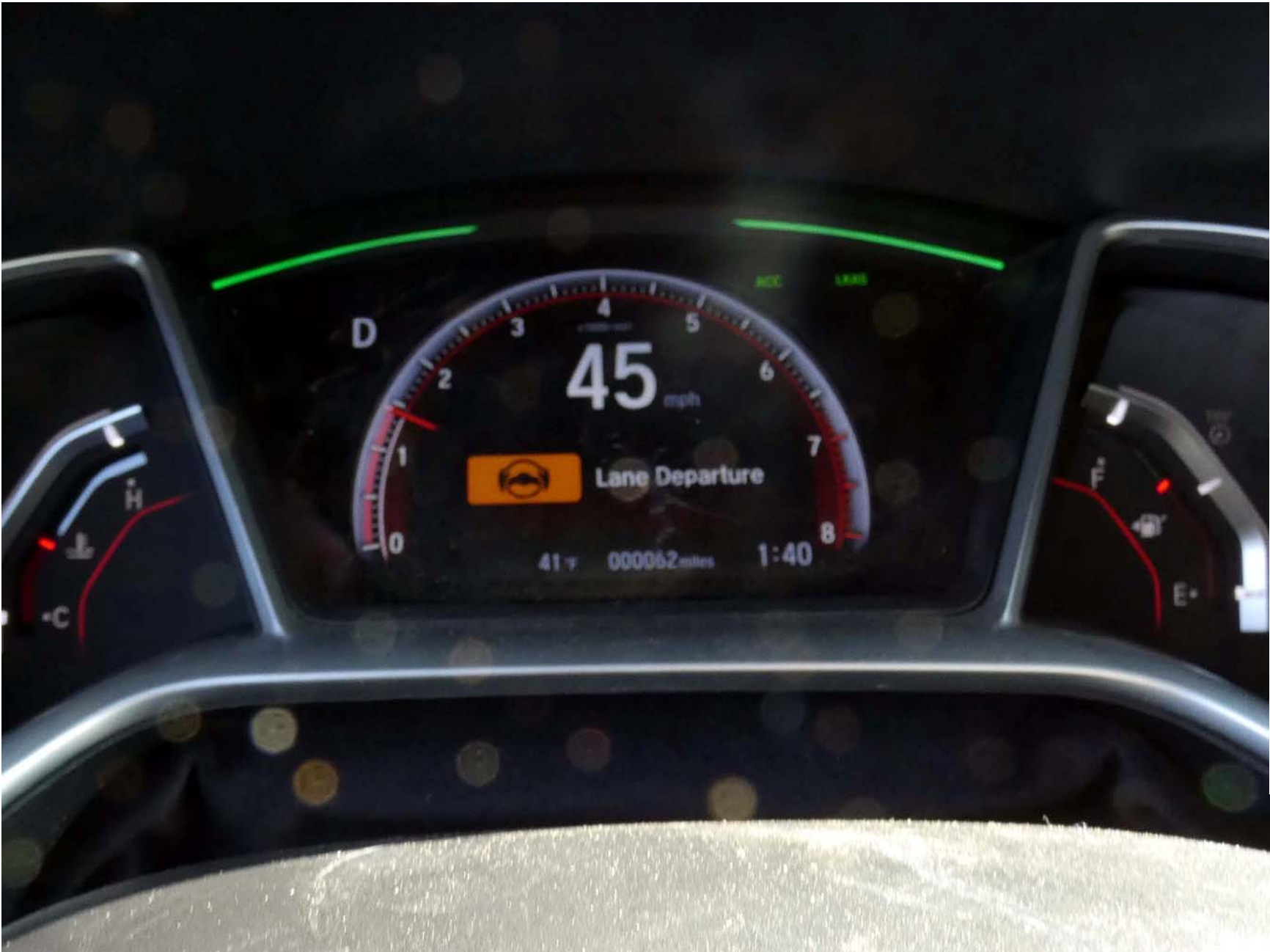
Figure A12. RDM (LDW) Instrument Panel Visual Alert
