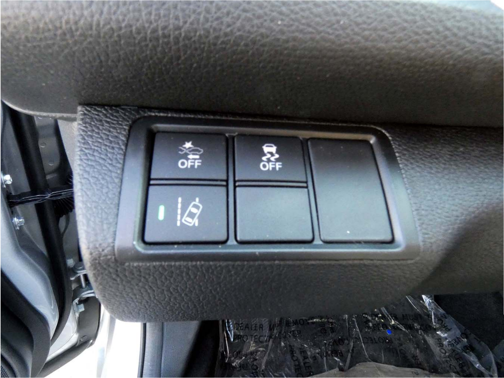
Figure A9. RDM (LDW) On/Off Switch
