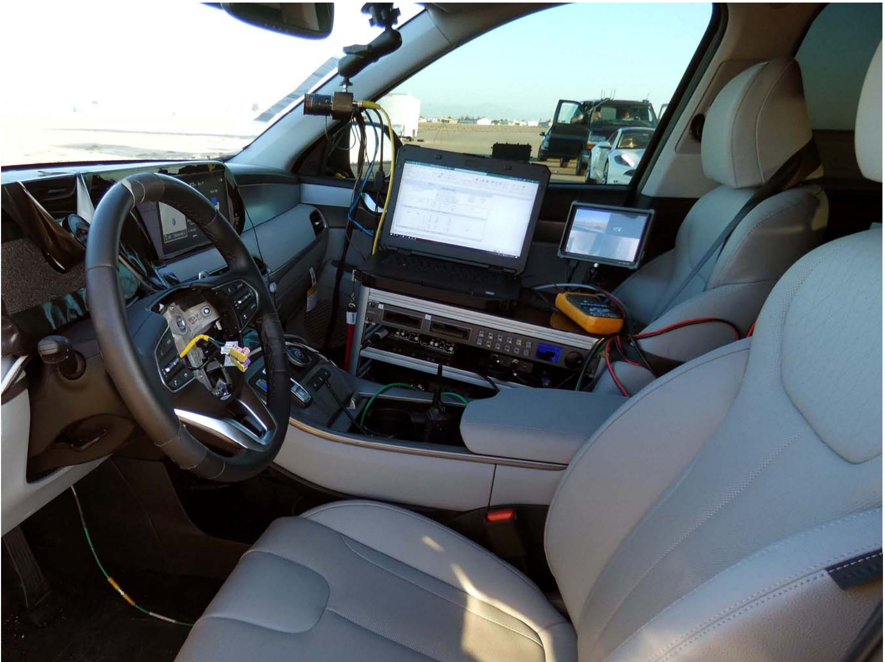
Figure A11. Computer Installed in Subject Vehicle
