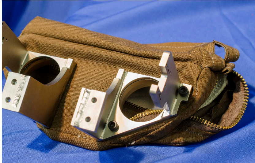
Figure 9-15. Left and right attachment brackets installed on lower abdomen
