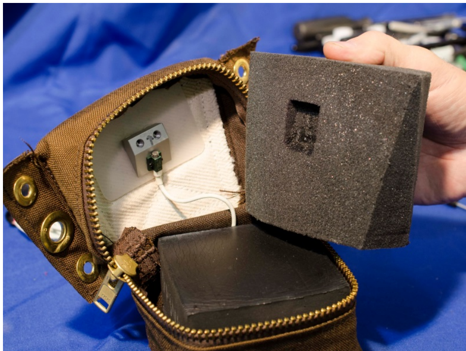
Figure 8-11. Front foam layer inserted into bag after attachment of accelerometer mount
