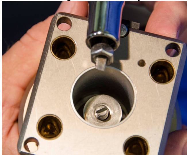
Figure 4-17. Technique for installing center neck cable
