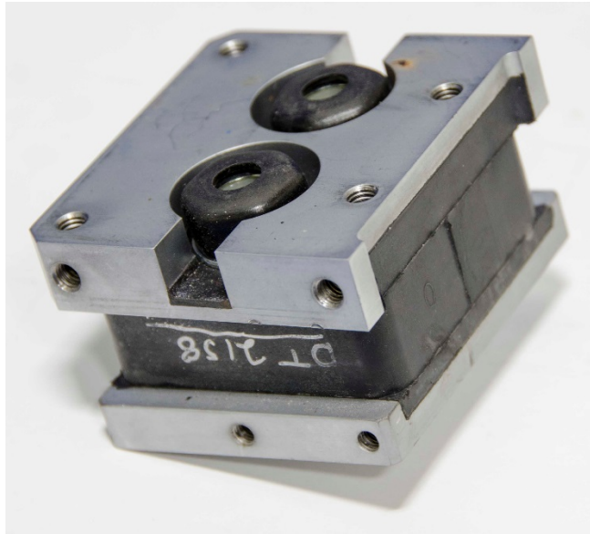
Figure 5-22. Vinyl covers for spine flex joint locknuts
