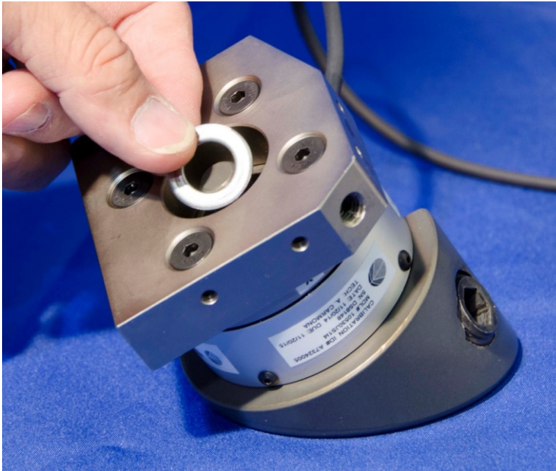
Figure 10-7. Install M12 flat washer
