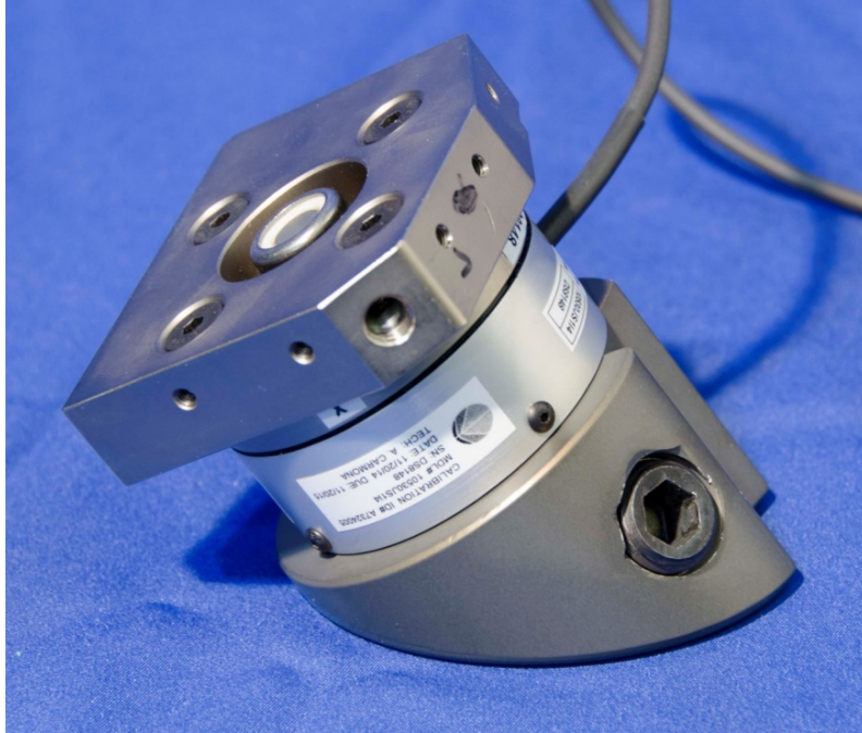
Figure 10-9. Acetabulum load cell installed to pelvic socket adaptor
