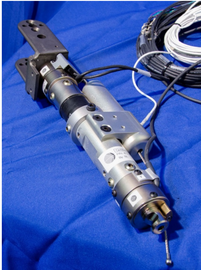
Figure 12-30. Attach Achilles spring tube to lower tibia tube
