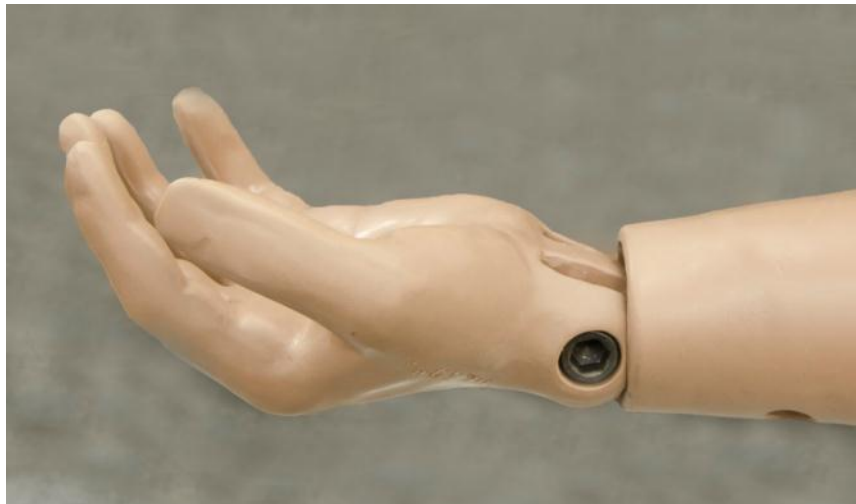
Figure 13-22. Wrist orientation for setting joint torque to 1G
