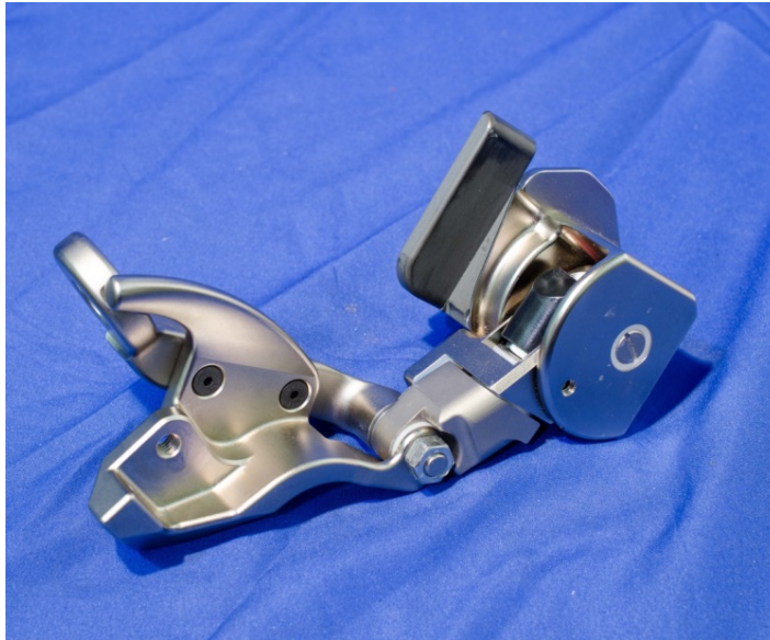
Figure 7-16. Secure scapula to arm link
