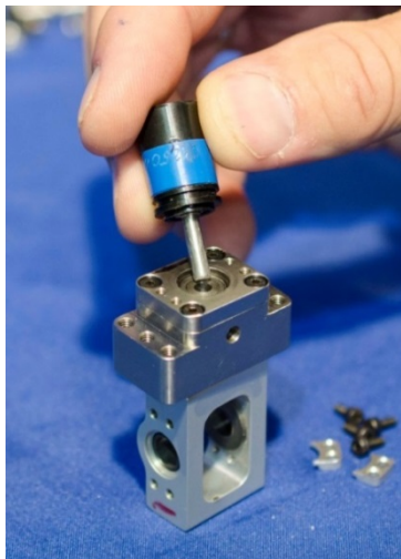
Figure 9-6. Insert Y-axis potentiometer
