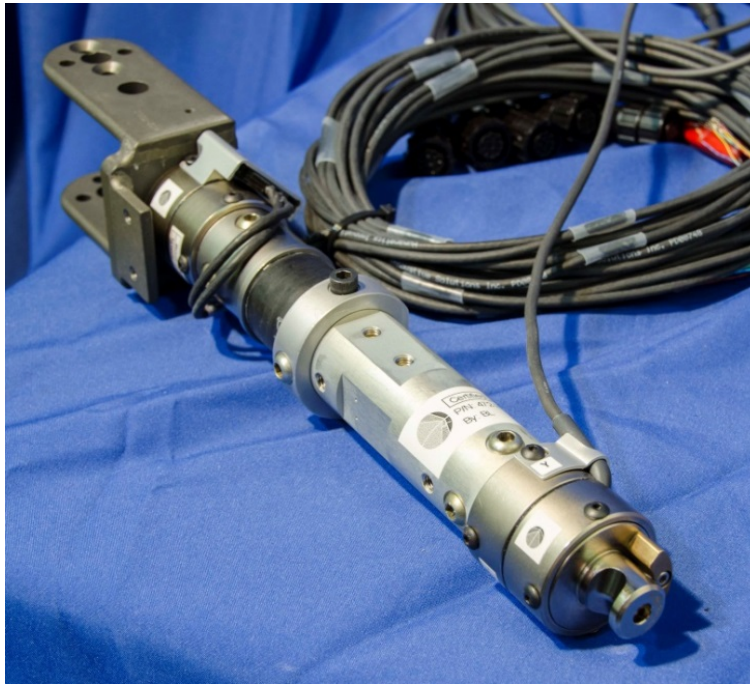
Figure 12-17. Lower leg assembled (without ankle)
