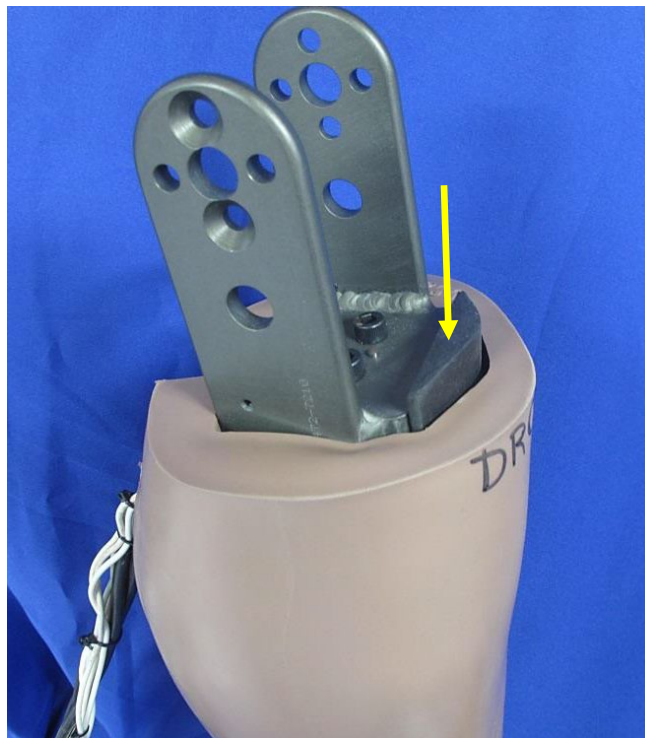
Figure 12-70. Position molded knee bumper into molded pocket on tibia skin
