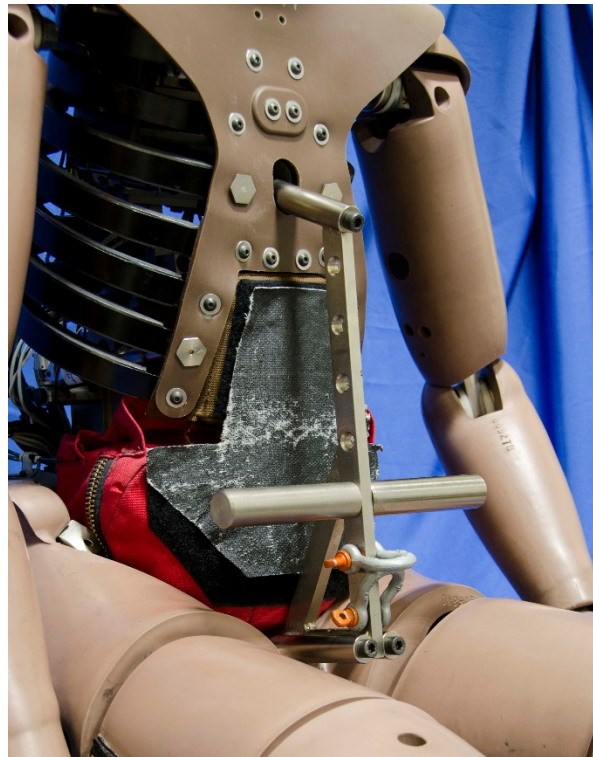
Figure 2-7. Storage bracket assembly secured to THOR-50M
