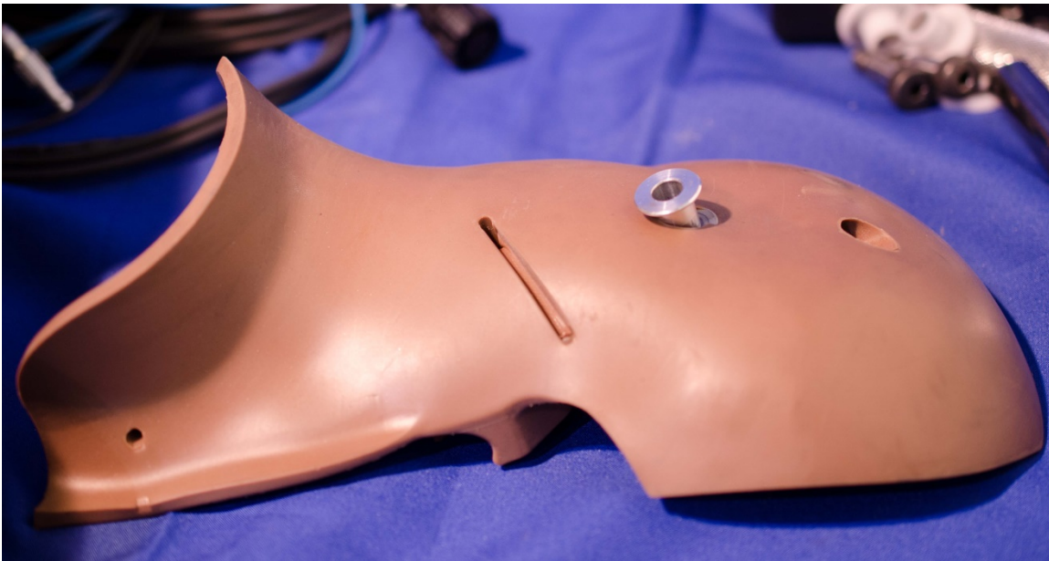
Figure 6-38. Install shoulder cover bushing
