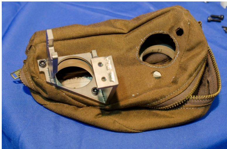
Figure 9-14. Left bracket assembled to internal plate
