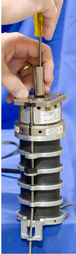
Figure 4-18. Install hardware for neck center cable
