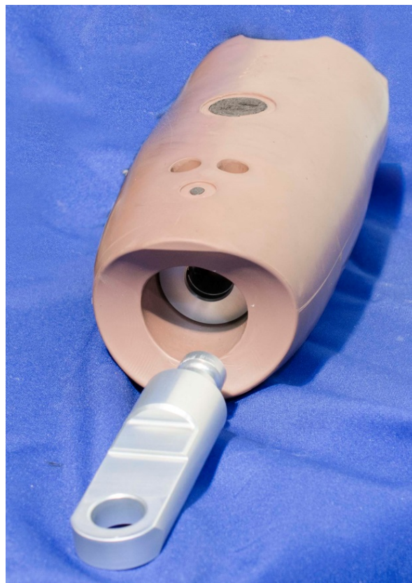
Figure 13-6. Insert upper arm lower section into humerus
