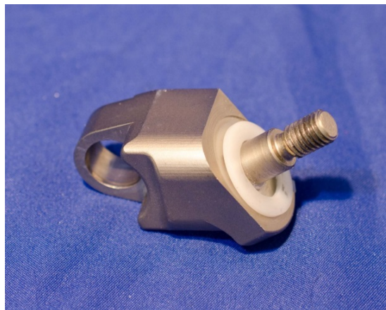
Figure 7-9. Assemble link washer on shoulder support pivot
