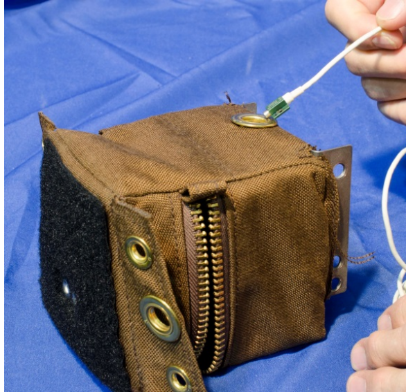
Figure 8-6. Insert accelerometer into upper abdomen bag
