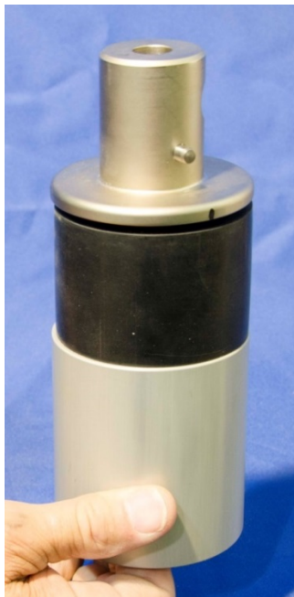
Figure 11-6. Assemble femur ball attachment plate to femur plunger assembly
