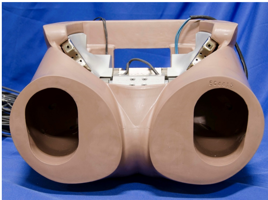
Figure 10-35. Pelvis mechanical assembly seated into pelvis skin
