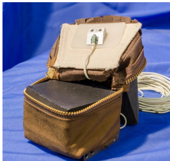
Figure 8-9. Securing upper abdomen accelerometer inside bag
