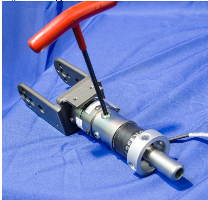
Figure 12-10. Install tibia compliant bushing assembly to upper tibia load cell
