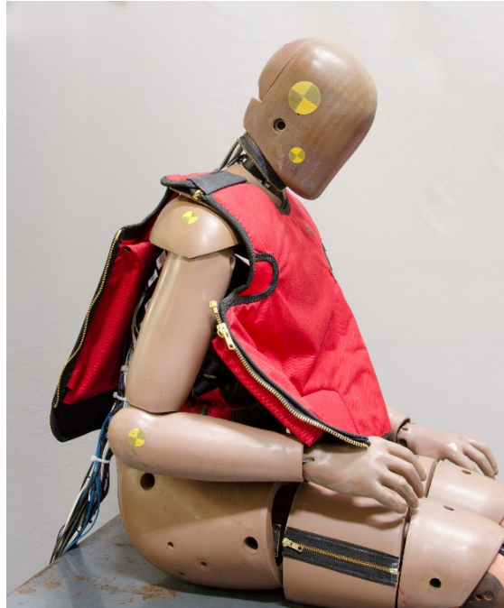
Figure 14-7. Drape front and rear panels over dummy then zipper shoulders
