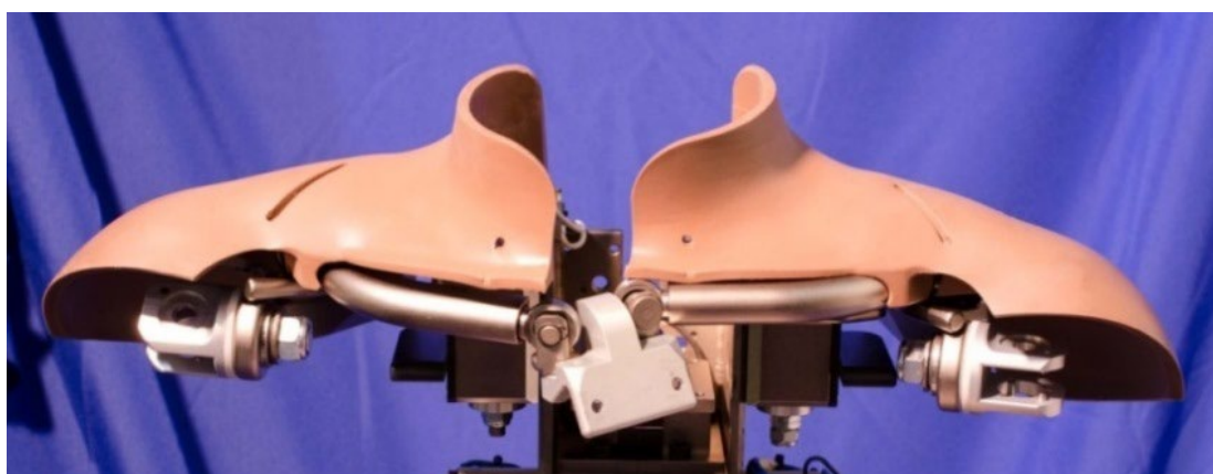
Figure 6-42. Attach shoulder pad assemblies
