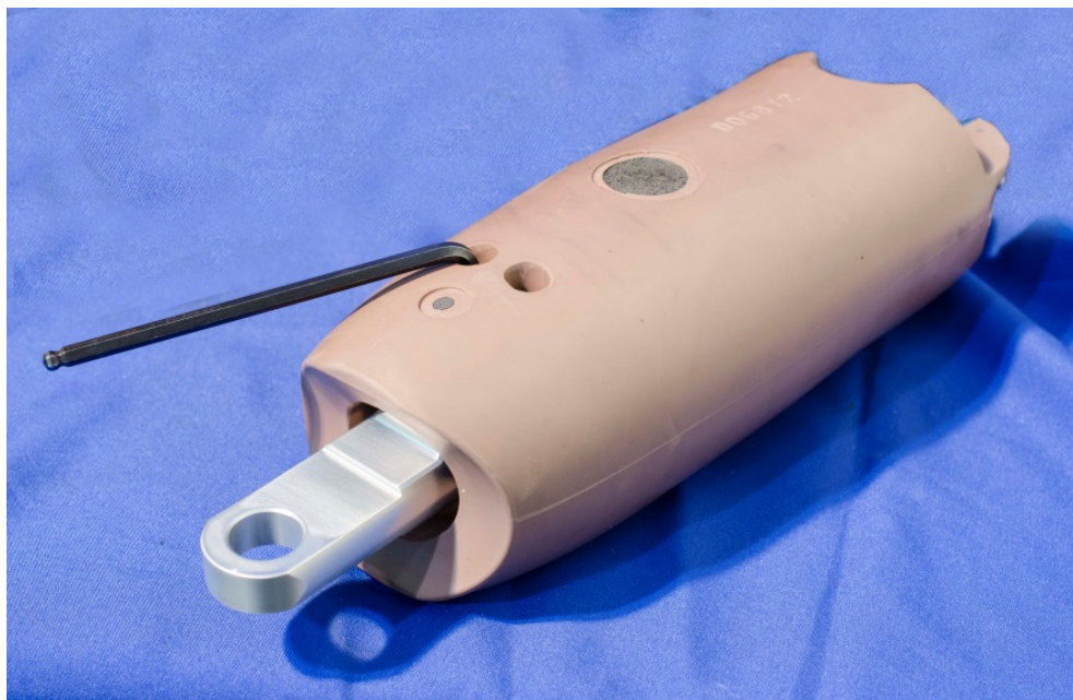
Figure 13-7. Secure upper arm lower section to humerus
