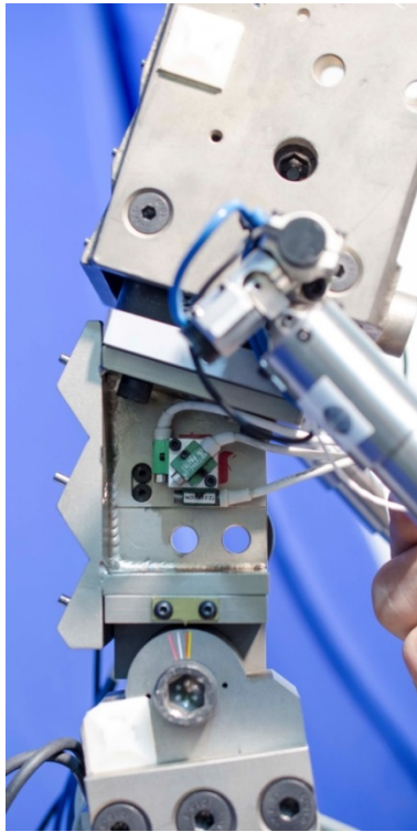
Figure 6-31. Install accelerometer block to right side of spine
