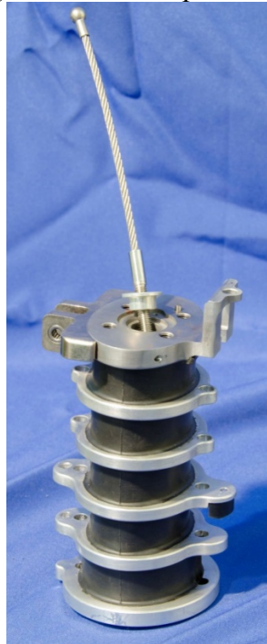
Figure 4-9. Insert neck center cable assembly
