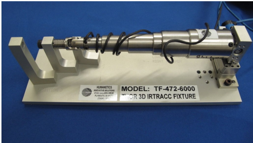
Figure 16-9. THOR-50M 3D IR-TRACC setup fixture
