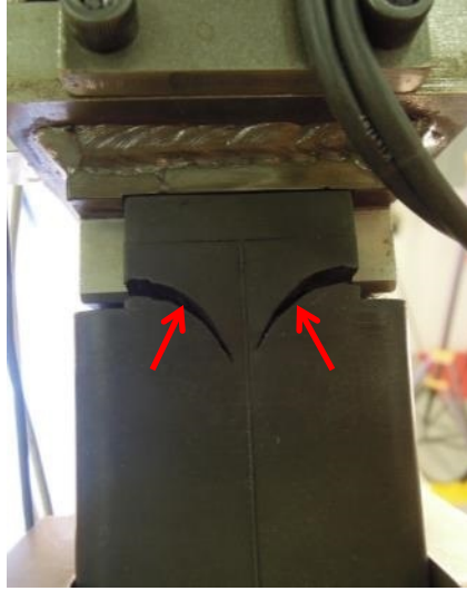
Figure 5-35. Tears in lumbar spine flex joint
