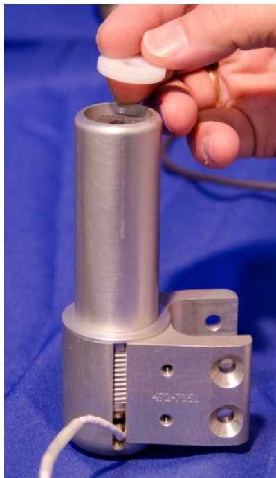
Figure 12-27. Insert Achilles primary washer
