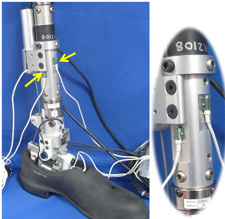
Figure 12-64. Mount accelerometers to lower tibia
