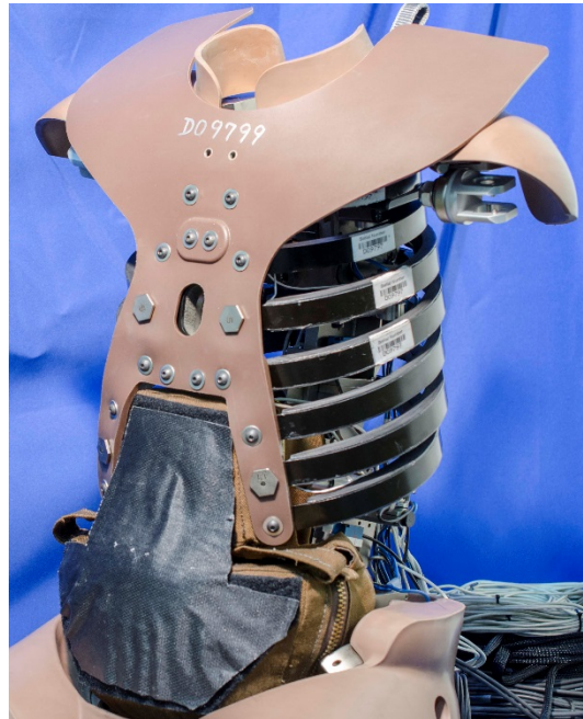
Figure 9-31. Abdomen cover installed
