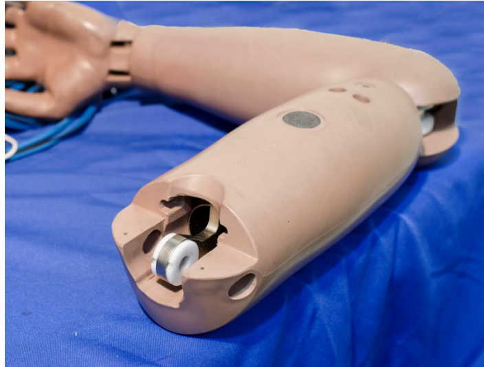
Figure 13-17. Install upper arm washer
