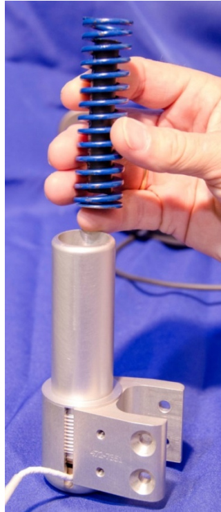
Figure 12-24. Install front compression tube assembly into spring tube
