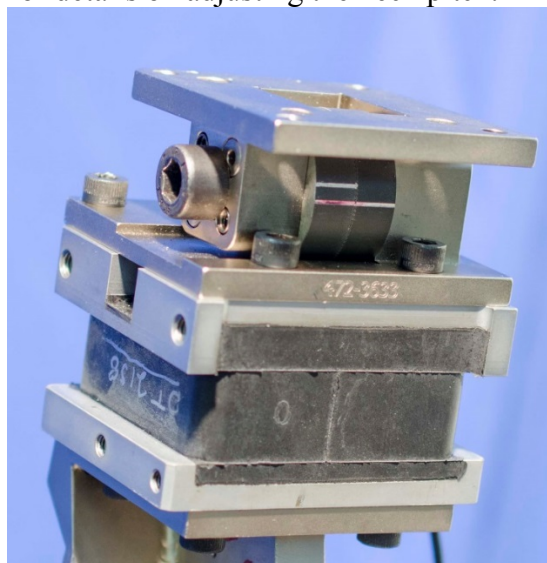
Figure 5-29. Neck pitch mechanism at “neutral” setting
