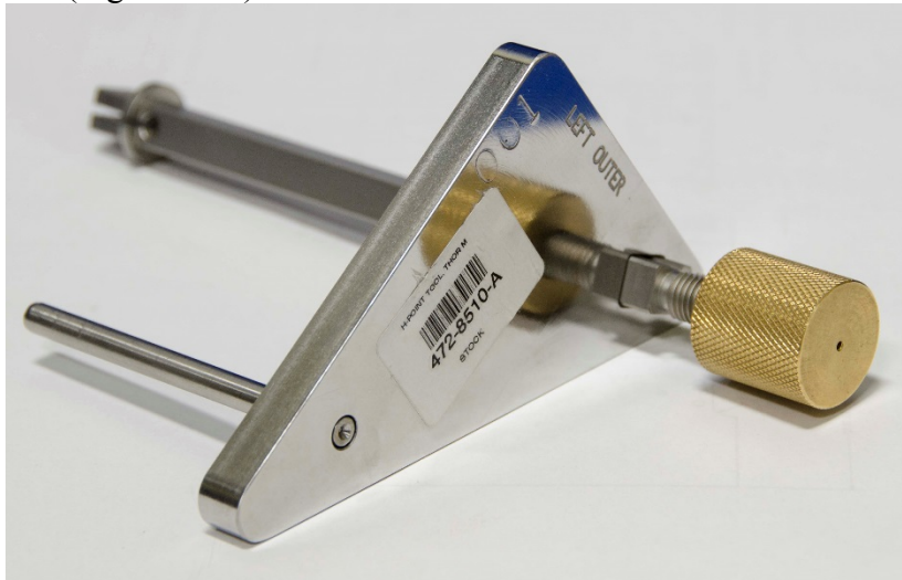
Figure 2-15. THOR-50M H-point tool assembled
