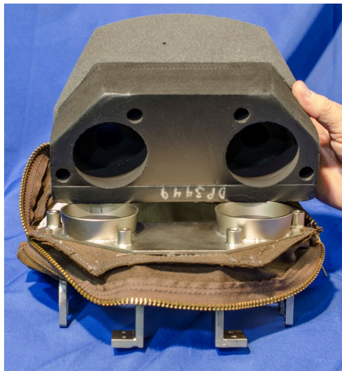
Figure 9-16. Align lower abdomen foams with cones
