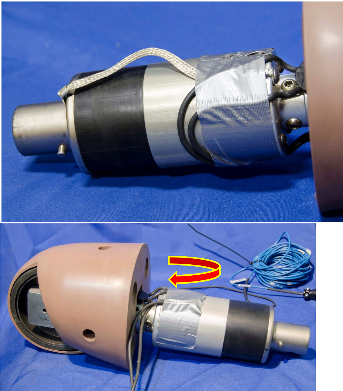
Figure 11-24. Tape femur load cell wiring in a loop for strain-relief
