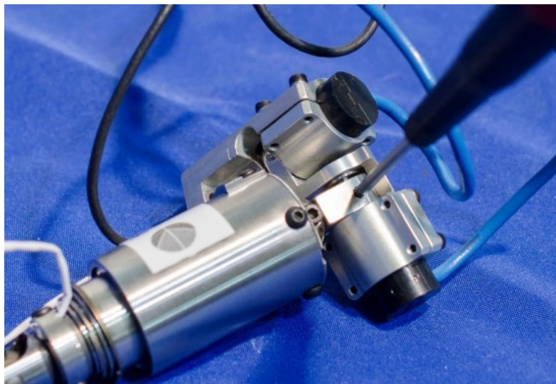
Figure 6-14. Tighten set screw against Z-axis potentiometer
