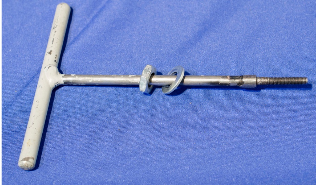
Figure 9-23. Insert washer and nut over threaded tool
