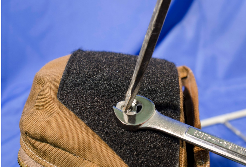
Figure 9-25. Use a screwdriver to prevent IR-TRACC rotation
