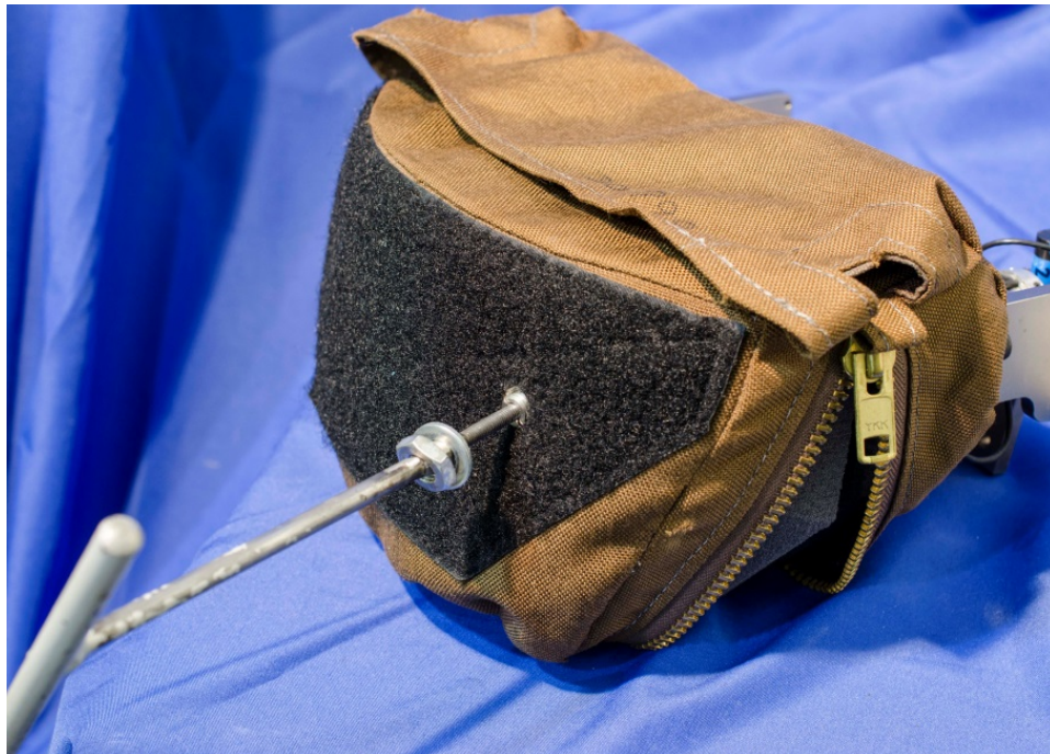
Figure 9-24. Install threaded tool into end of lower abdomen IR-TRACC
