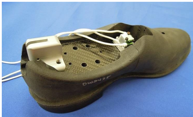
Figure 12-60. Achilles mounting post installed to molded shoe
