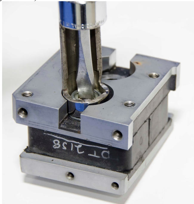
Figure 5-21. Install locknuts to spine flex joint cables
