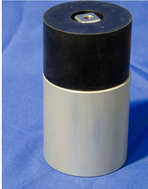
Figure 11-5. Assemble upper leg compression element to femur plunger assembly
