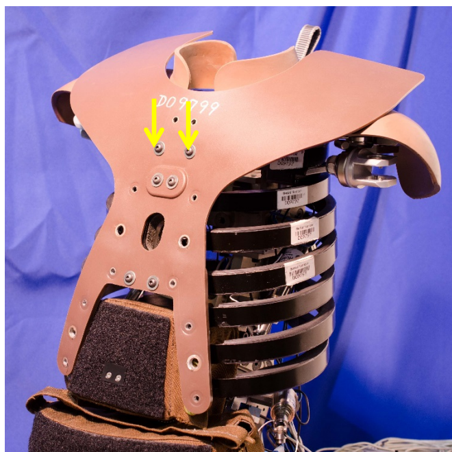
Figure 6-50. Install Rib #1 at sternum
