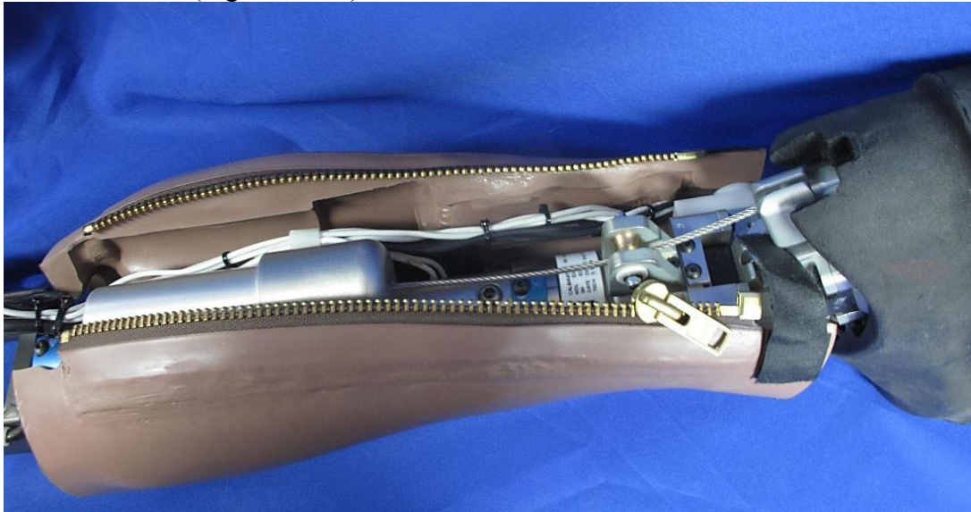
Figure 12-69. Loosely install the lower leg flesh
