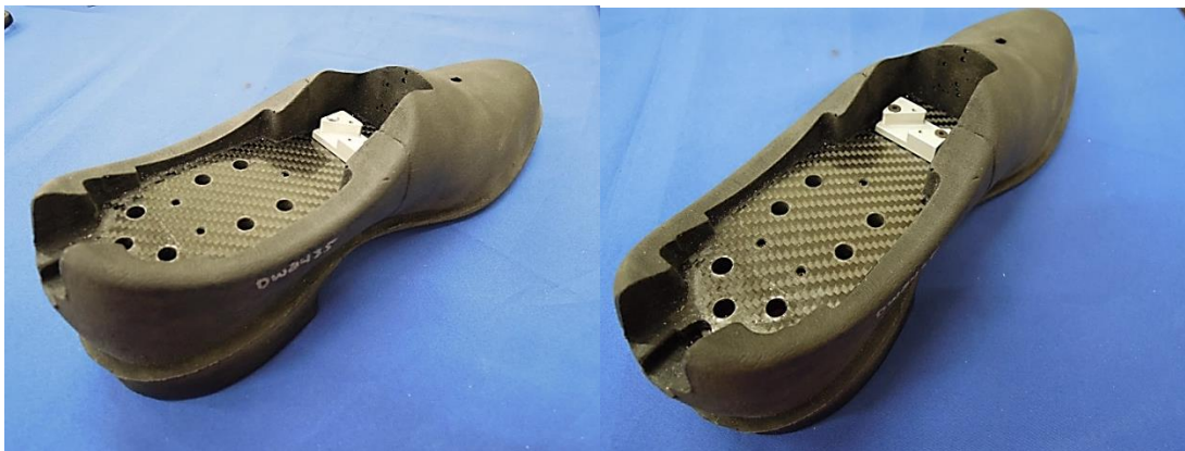
Figure 12-55. Install tri-pack accelerometer mounting plates to molded shoe
