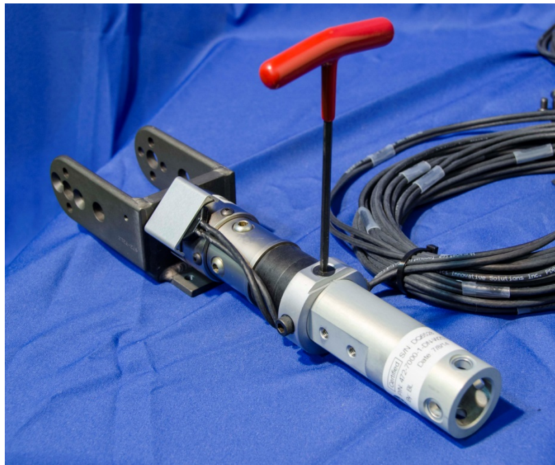
Figure 12-14. Secure lower flange
