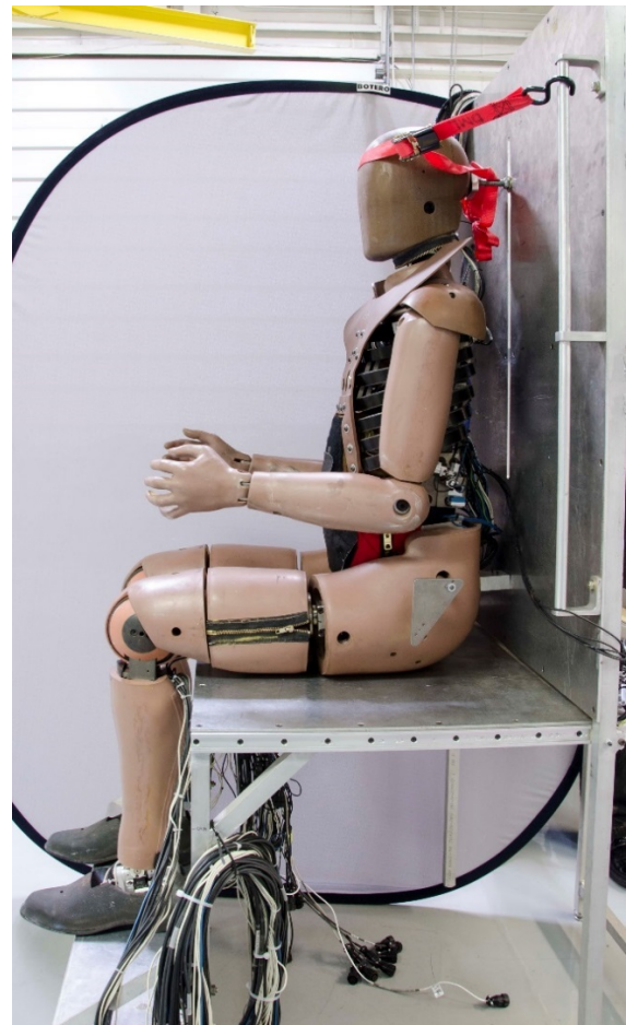
Figure 19-7. Placement of head strap
