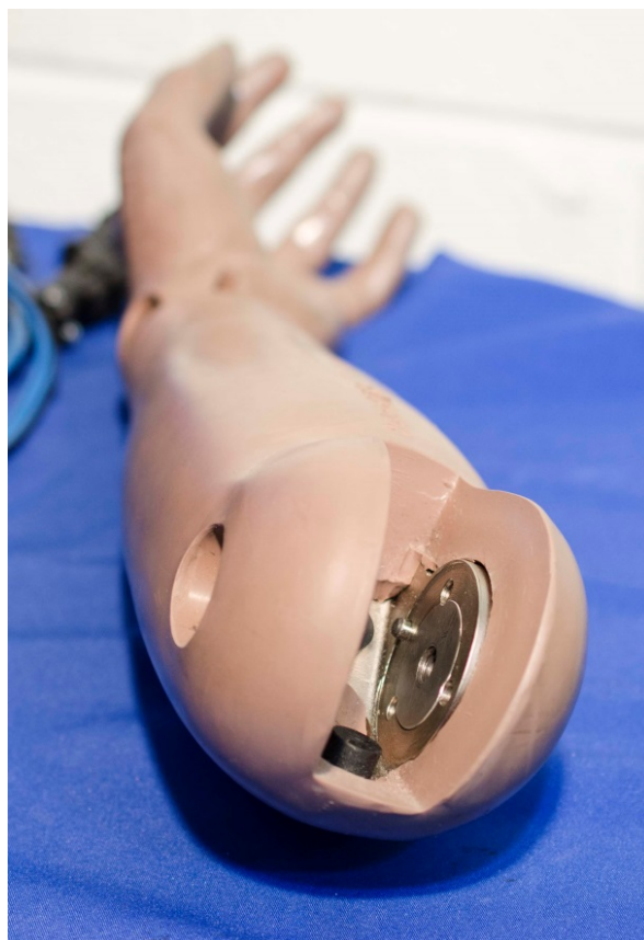
Figure 13-12. Elbow pivot nut installed
