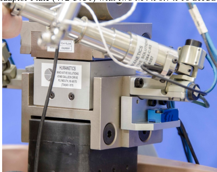
Figure 6-28. Install T12 tilt sensor to spine
