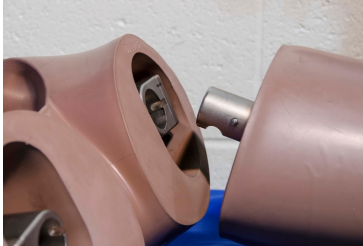
Figure 11-26. Insert upper leg into pelvis for attachment
