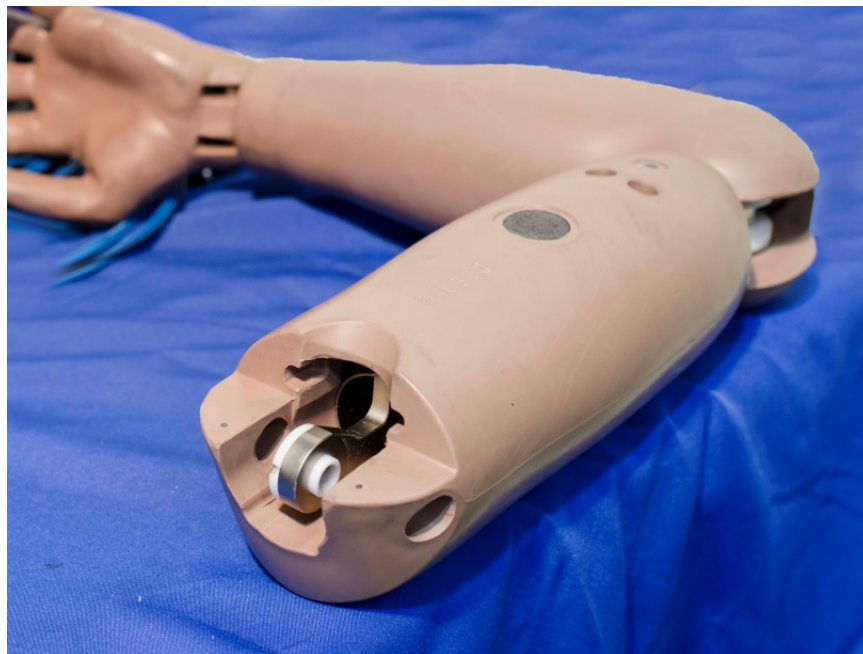
Figure 13-16. Insert upper arm bushing into humerus
