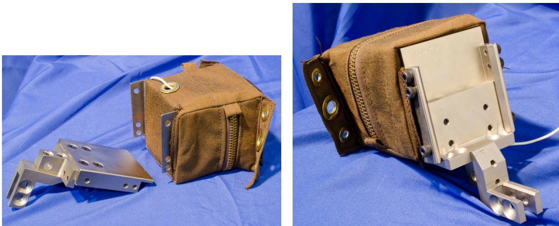
Figure 8-15. Secure Upper Abdomen Bag to Spinal Mount Bracket Assembly
