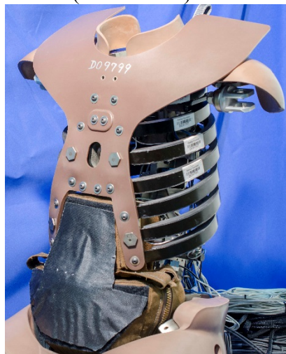
Figure 8-18. Abdomen cover installed
