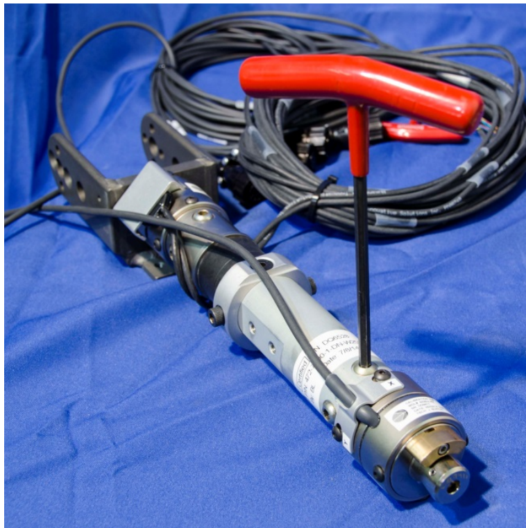
Figure 12-16. Connect lower tibia load cell to lower tibia tube assembly
