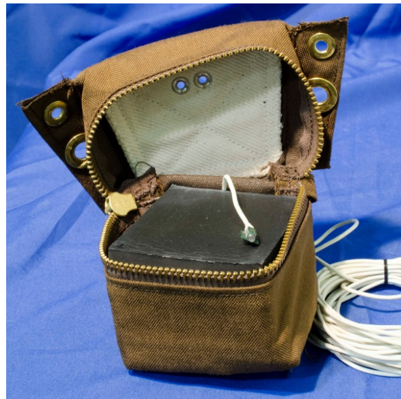
Figure 8-7. Route accelerometer along inside top of upper abdomen bag
