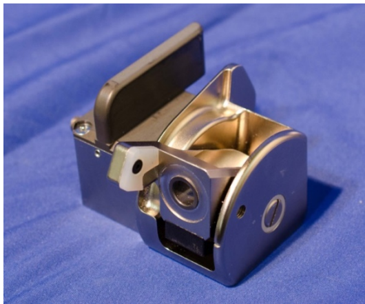
Figure 7-8. Install lower left buffer
