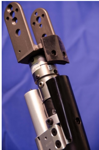
Figure 12-66. Secure molded knee bumper
