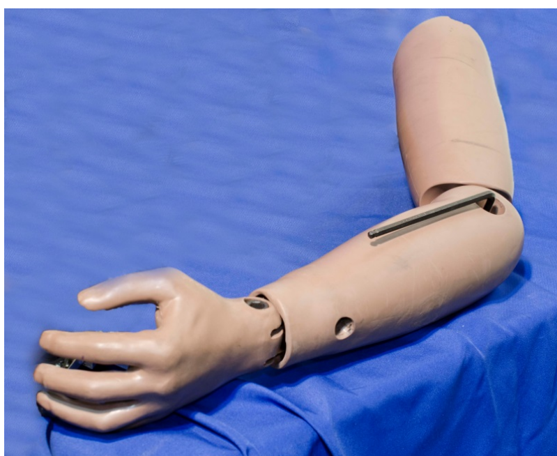
Figure 13-14. Secure upper arm and humerus at elbow
