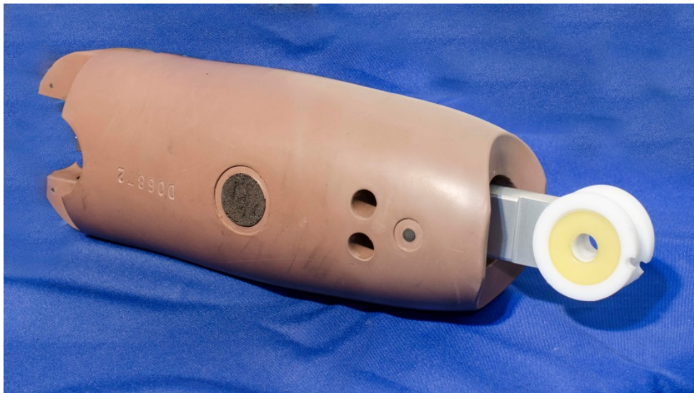
Figure 13-10. Place shoulder joint spring washer into upper arm and elbow pivot bushing
