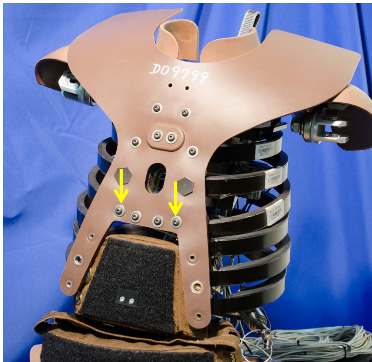
Figure 6-55. Install Rib #4 at sternum
