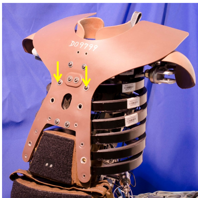
Figure 6-51. Install Rib #2 at sternum
