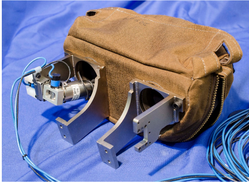
Figure 9-20. Cable strain relief for the lower abdomen IR-TRACCs
