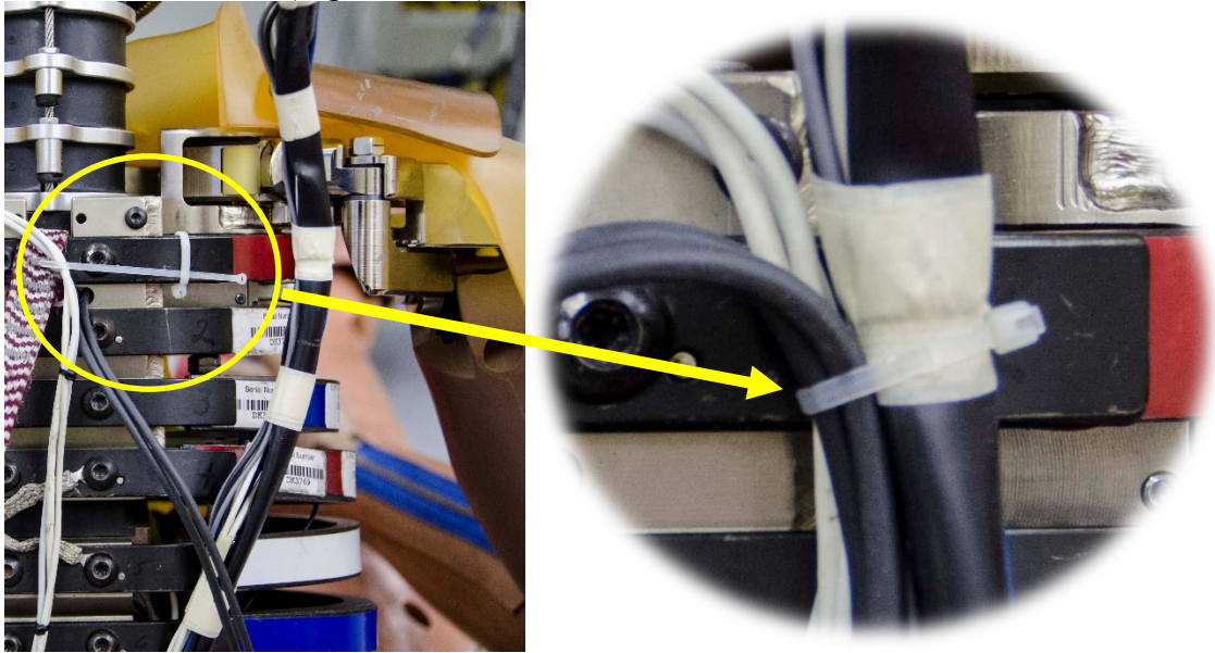
Figure 15-21. Create an anchor on rib #1 for the neck cable bundle
