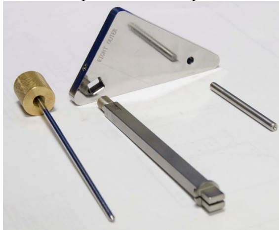
Figure 2-12. H-point tool components
