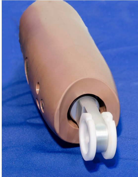
Figure 13-9. Install upper arm and elbow pivot washer into upper arm
