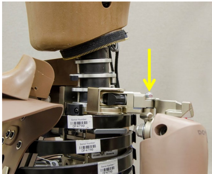
Figure 7-22. Locknut on joint connecting shoulder support assembly to arm link.
