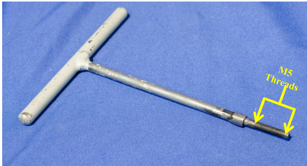
Figure 9-22. Example of threaded tool for aiding lower abdomen IR-TRACC installation
