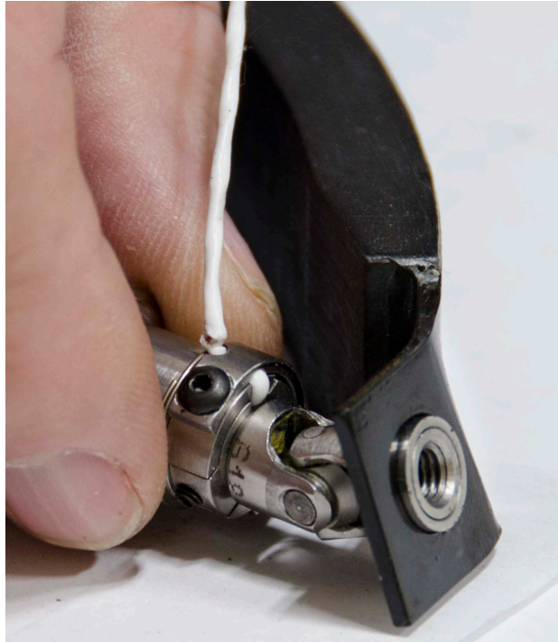
Figure 6-54. Rib attachment for IR-TRACC
