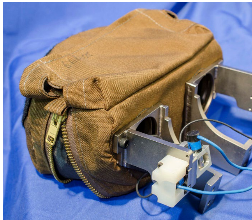
Figure 9-19. Install potentiometer cover to bracket weld assembly
