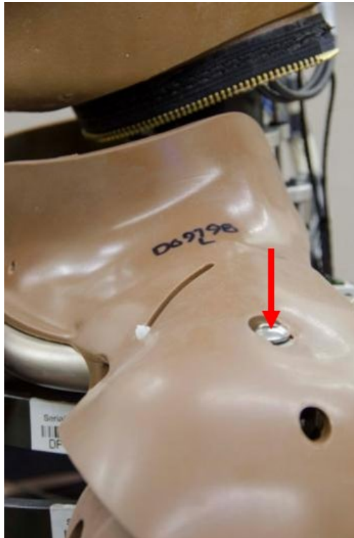
Figure 7-20. Disconnect clavicles at shoulders (shoulder pad cable ties may be left intact)
