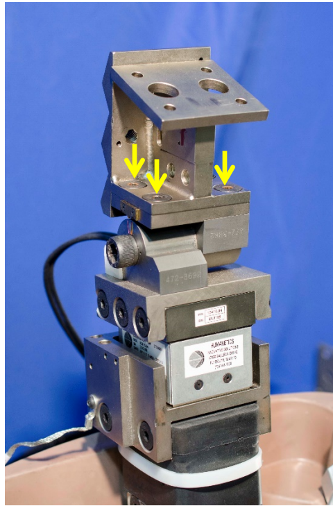
Figure 5-18. Install lower thoracic spine assembly to lumbar spine pitch change assembly
