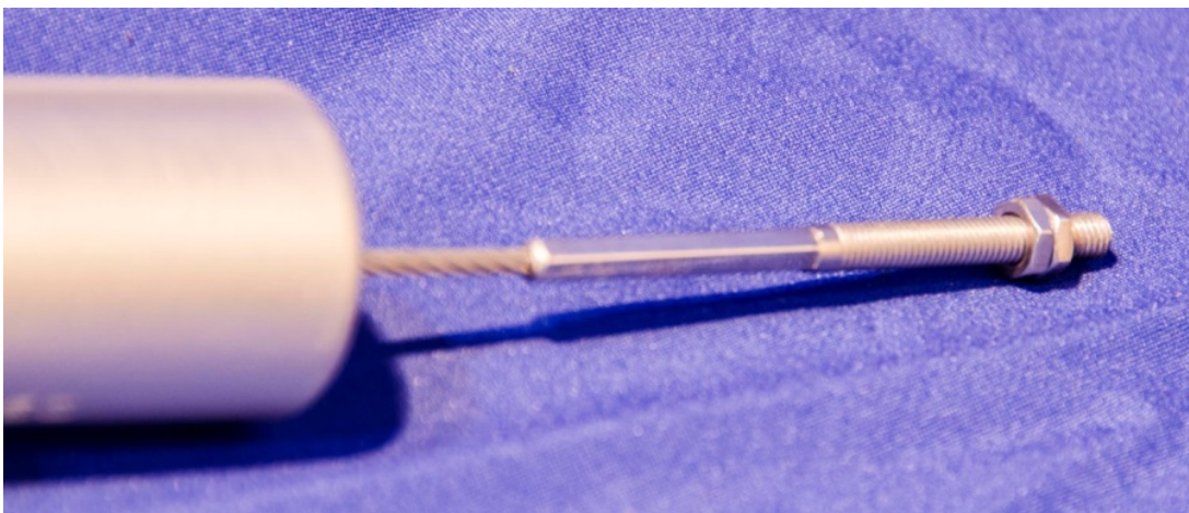
Figure 12-29. Secure Achilles cable with hex jam nuts
