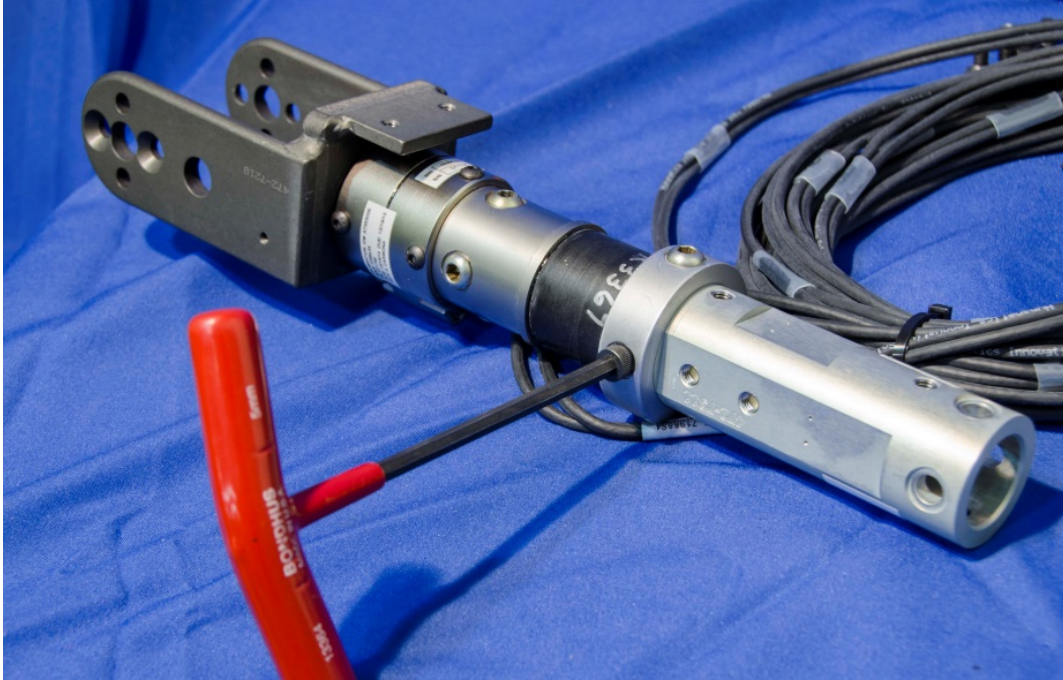
Figure 12-13. Mount plunger retaining bolts
