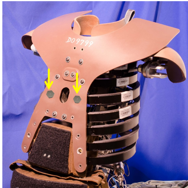
Figure 6-52. Install Rib #3 at sternum
