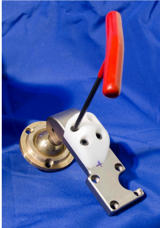
Figure 10-36. Install trochanter to hip arm
