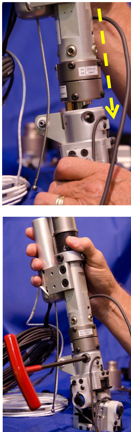
Figure 12-53. Attach lower tibia load cell to ankle top torque base
