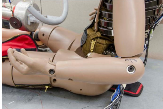
Figure 13-23. Elbow orientation for setting joint torque to 1G
