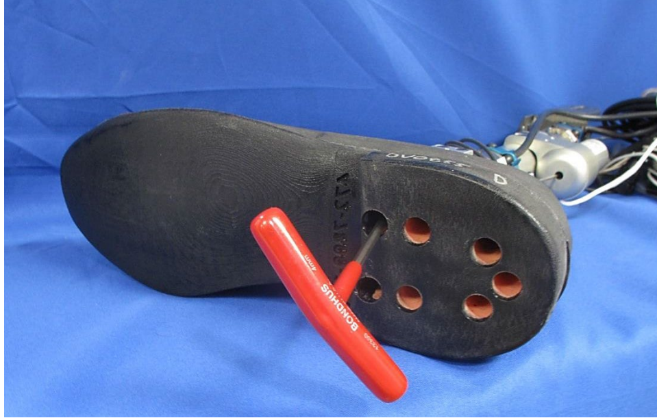
Figure 12-61. Mount molded shoe assembly to ankle
