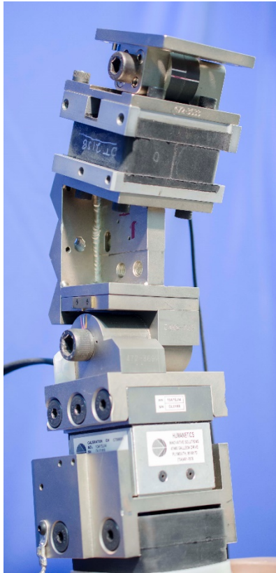
Figure 5-28. Neck pitch change mechanism assembled to upper spine flex joint
