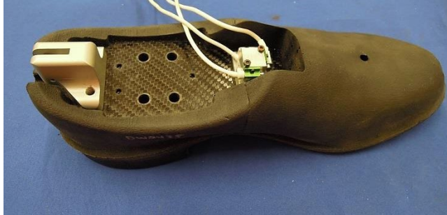
Figure 12-58. Achilles mounting post and molded shoe
