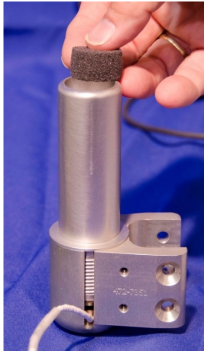
Figure 12-26. Assemble foam compression element into Achilles
