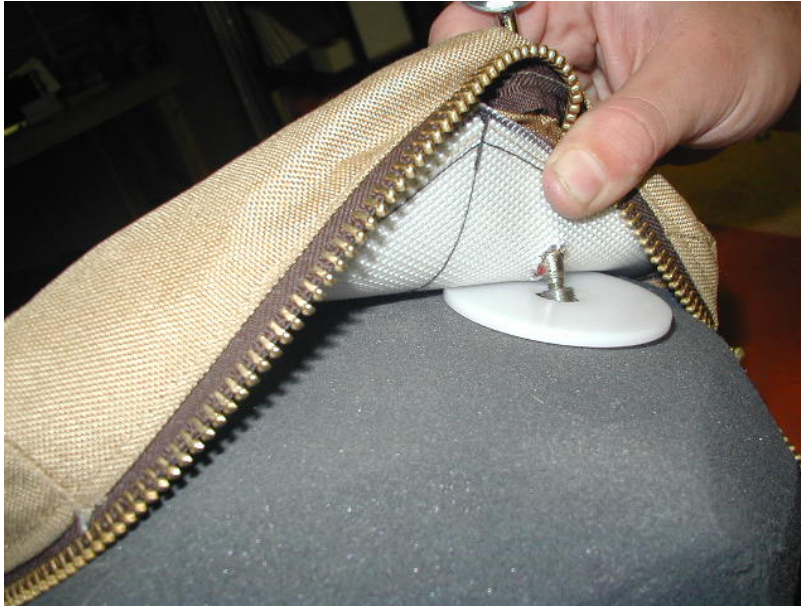
Figure 9-21. Install load distribution plate
