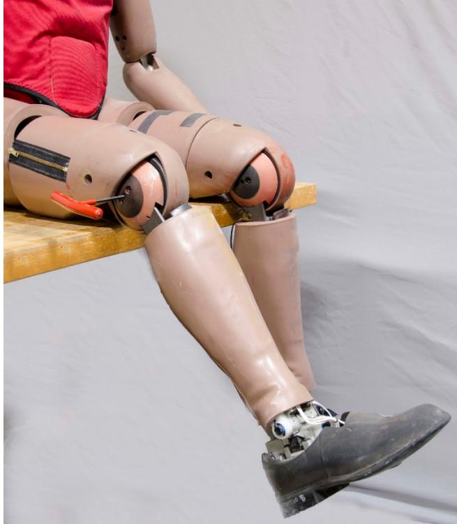
Figure 12-76. Setting the knee to 1G
