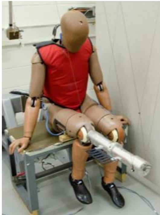
**Figure 3-36. Upper leg impact test for knee skin and compliant bushing**
