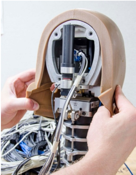
Figure 5-1. Separation of head skin from grooves at posterior of skull assembly.
