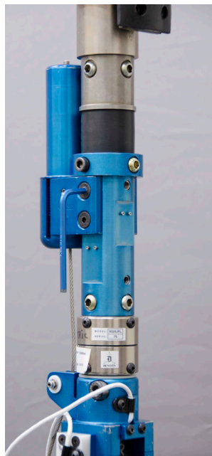
Figure 12-13. Remove Achilles spring tube assembly.
