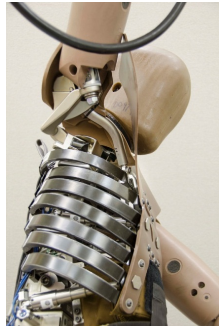
Figure 6-16. Rib #1 can be moved to access wiring for neck removal.
