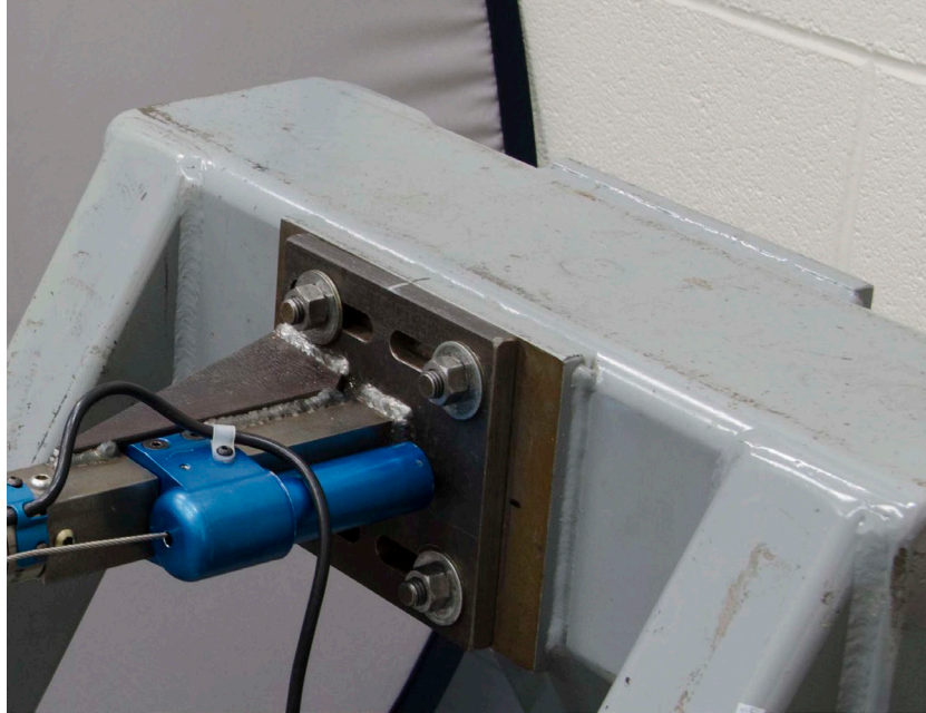
Figure 12-4. Orientation of lower leg mounting bracket for eversion tests.
