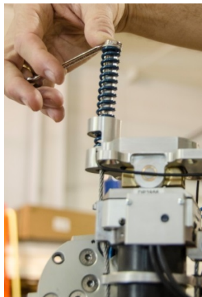
Figure 6-7. Install jam nut on front and rear springs after achieving desired plate angle setting.
