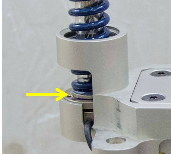
Figure 6-5. Front spring properly seated against spring load cell.
