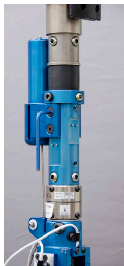
Figure 14-2. Remove Achilles spring tube assembly.
