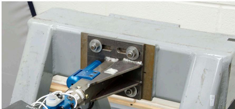
Figure 12-3. Orientation of lower leg mounting bracket for inversion tests.
