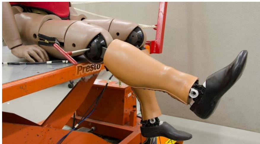
Figure 10-1. Knee orientation for setting joint torque to 1G.
