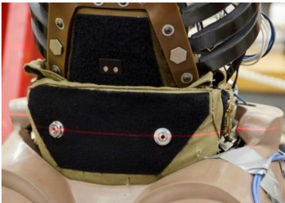
Figure 9-4. Horizontal alignment of IR-TRACC attachment nuts.
