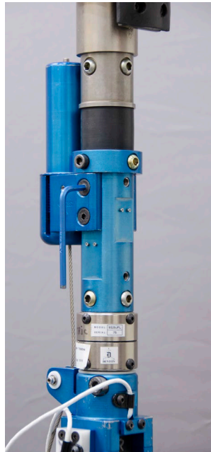
Figure 3-17. Remove Achilles spring tube assembly.
