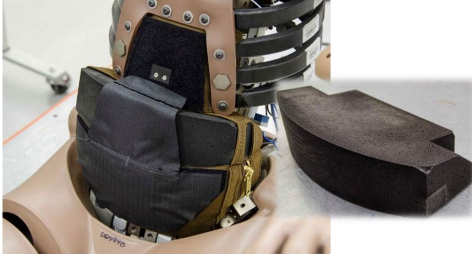
Figure 5-5. Erect posture foam (right) as inserted into the lower abdomen bag (left).
