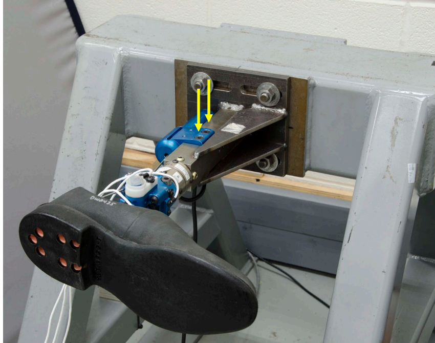
Figure 12-6. Install Achilles tube assembly to mounting bracket.
