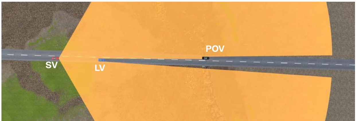
Figure 1: Simulation for Field of view of a state-of-the-art fusion sensor system (camera/radar)
