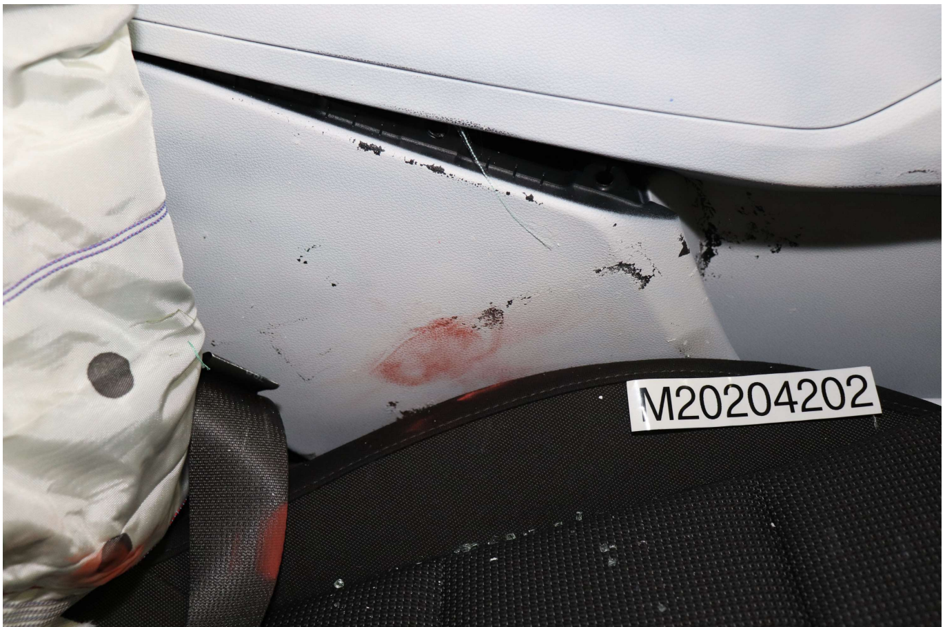
Photo No. 052 - Post-Test Driver Dummy Close-up Pelvis Contact with Vehicle Interior View
