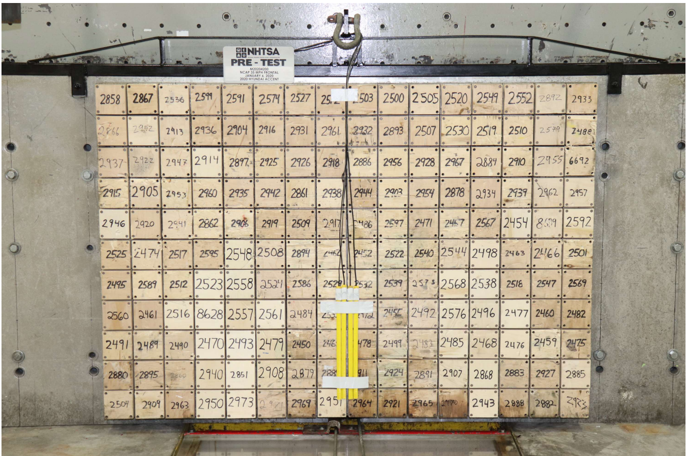
Photo No. 002 - Pre-Test Load Cell Wall
