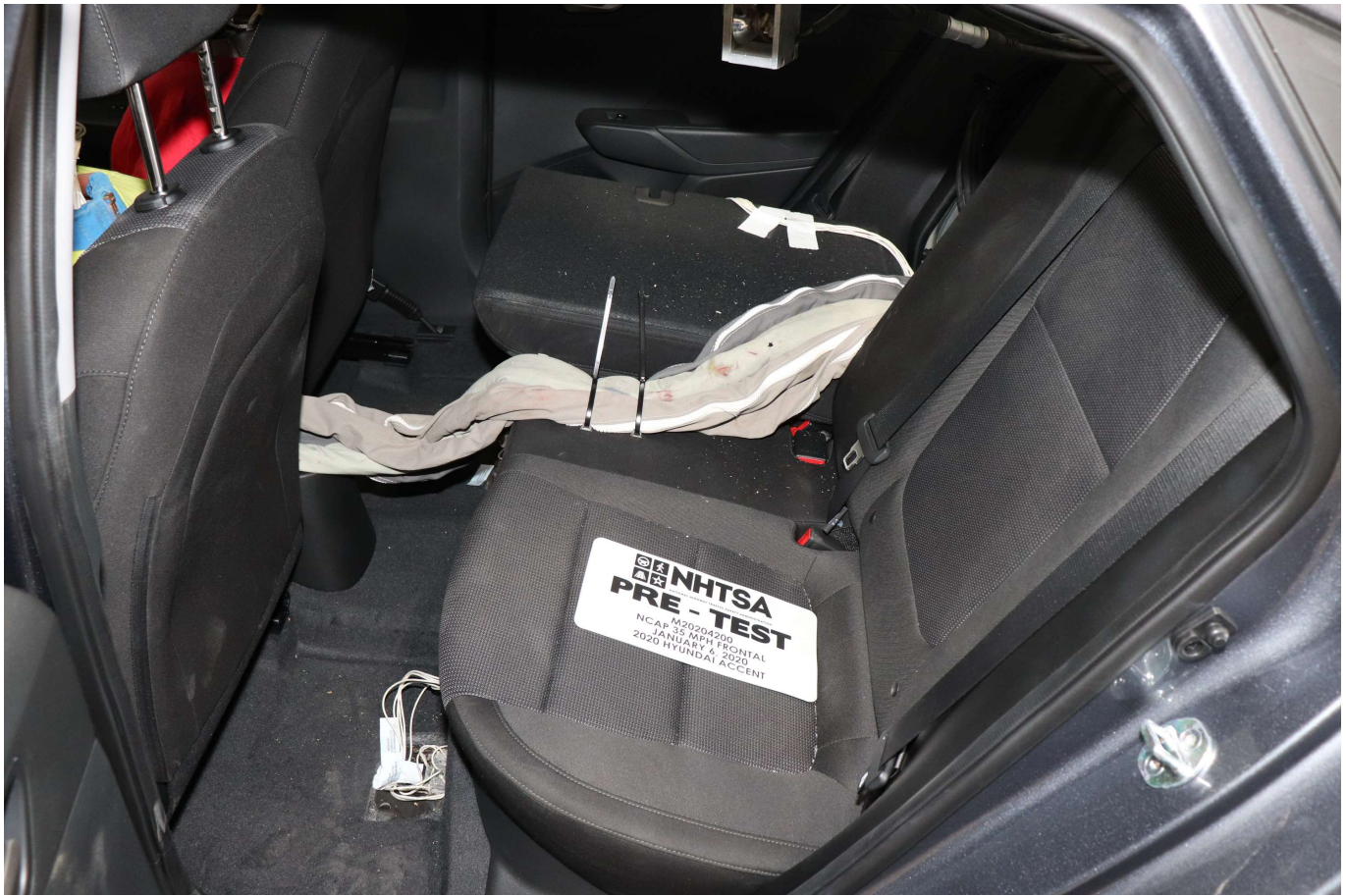
Photo No. 028 - Pre-Test Dummy Cable Routing
