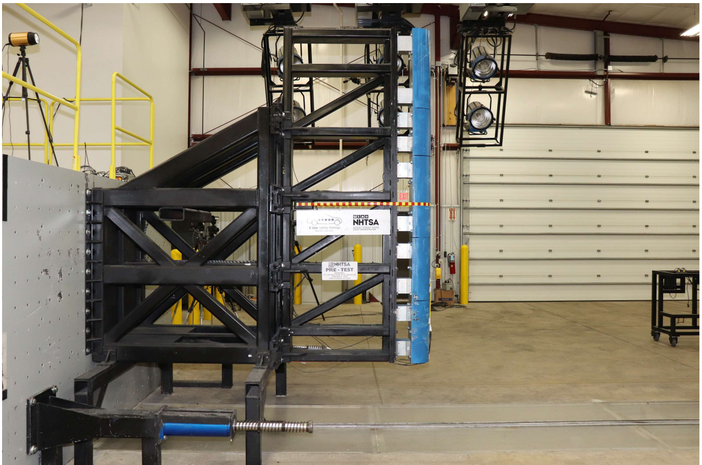
Photo No. 059 - Pre-Test Pole Barrier Side View
