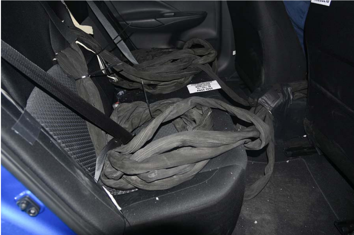
FIGURE 29. Post-Test Dummy Cable Routing
