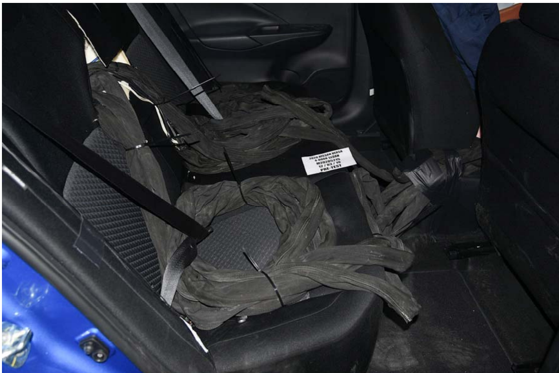
FIGURE 28. Pre-Test Dummy Cable Routing
