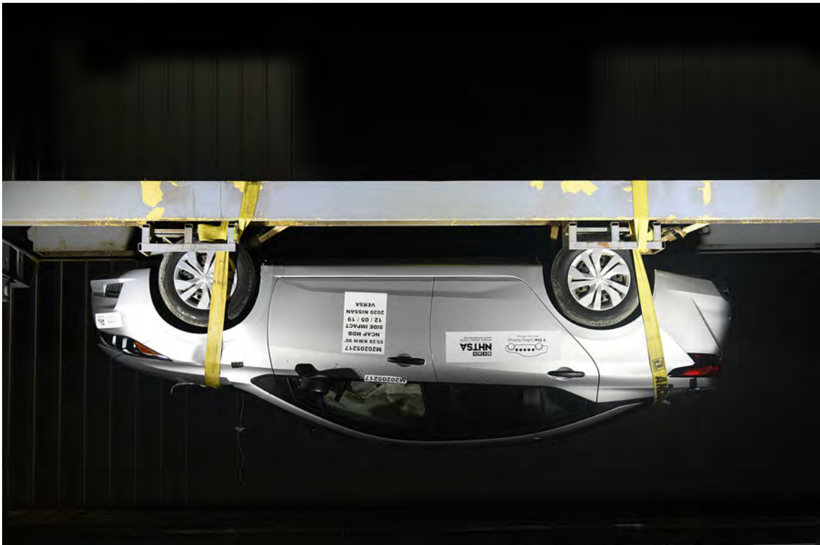
FIGURE 98. FMVSS No. 301 Static Rollover 180 Degrees
