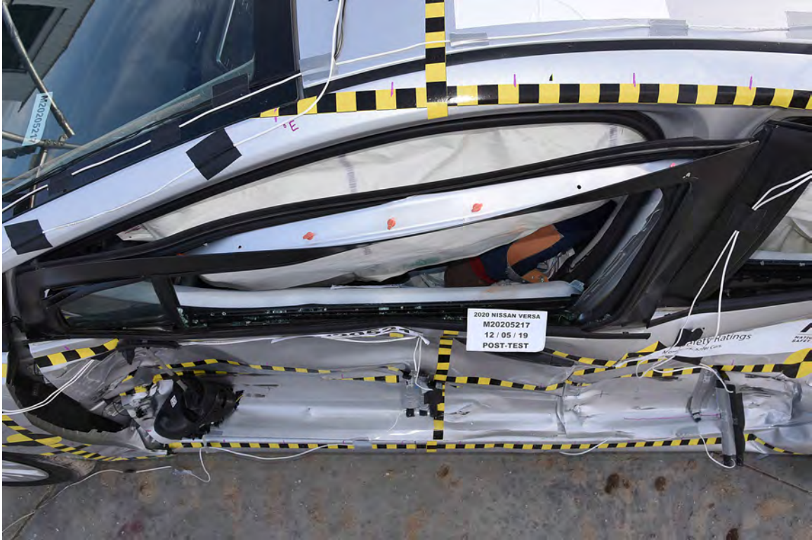
FIGURE 43. Post-Test Driver Dummy and Door Clearance View
