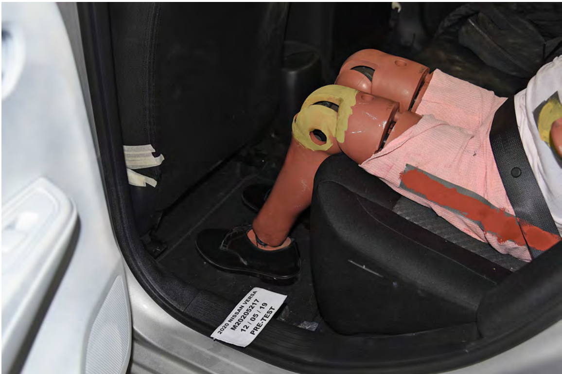
FIGURE 64. Pre-Test Placement of Rear Passenger Dummy's Feet
