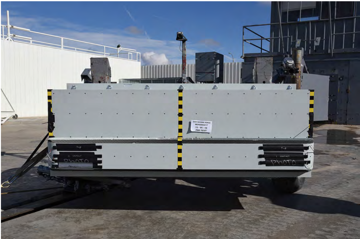
FIGURE 84. Pre-Test Front View of MDB Impactor Face
