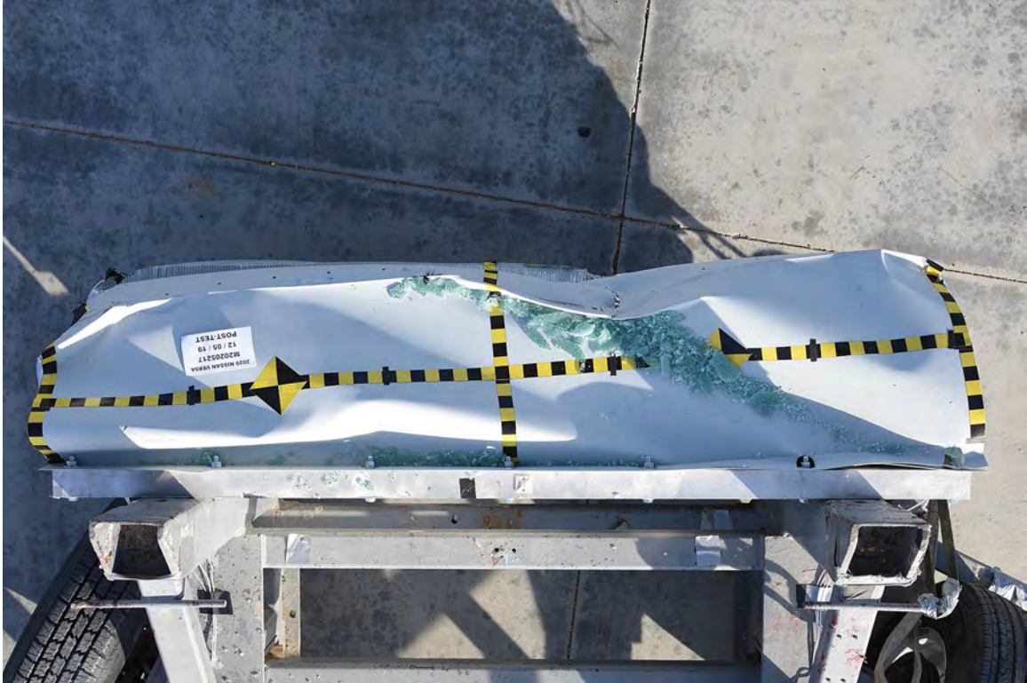
FIGURE 87. Post-Test Top View of MDB Impactor Face
