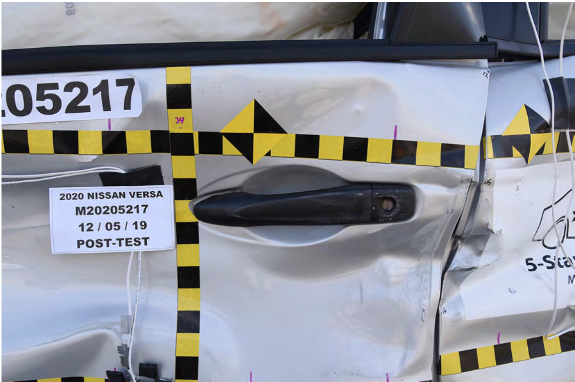
FIGURE 22. Post-Test Left Front Door Latch Close-Up
