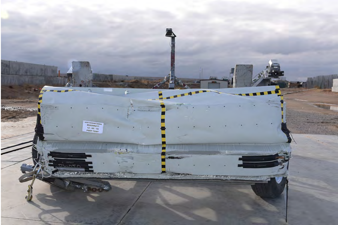
FIGURE 85. Post-Test Front View of MDB Impactor Face
