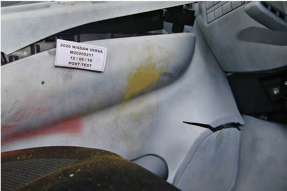
FIGURE 54. Post-Test Driver Dummy Close-Up Knee Contact View
