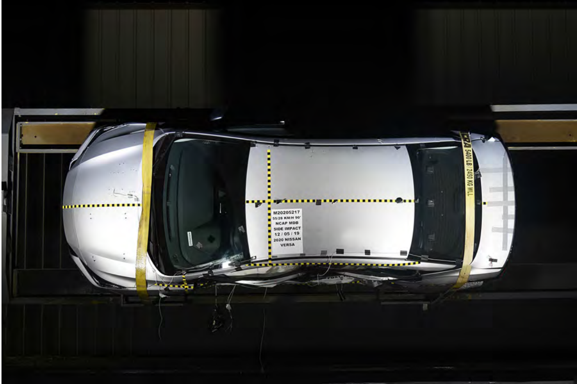
FIGURE 97. FMVSS No. 301 Static Rollover 90 Degrees
