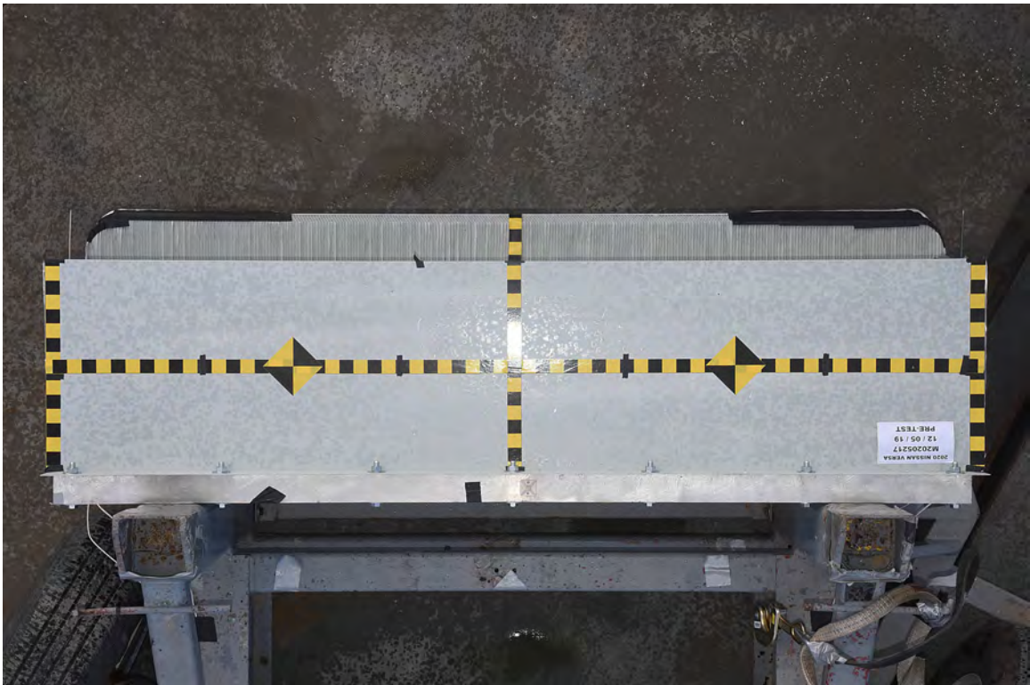
FIGURE 86. Pre-Test Top View of MDB Impactor Face
