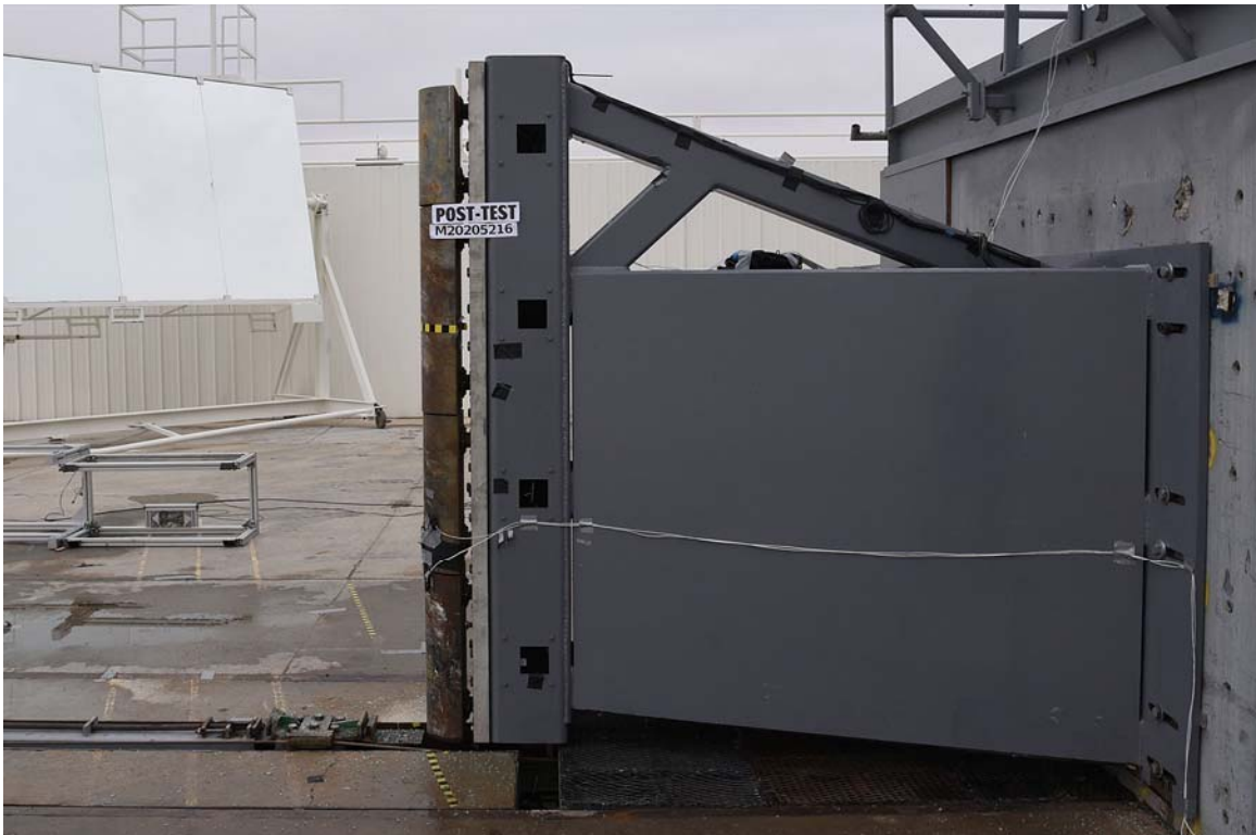
FIGURE 60. Post-Test Pole Barrier Side View
