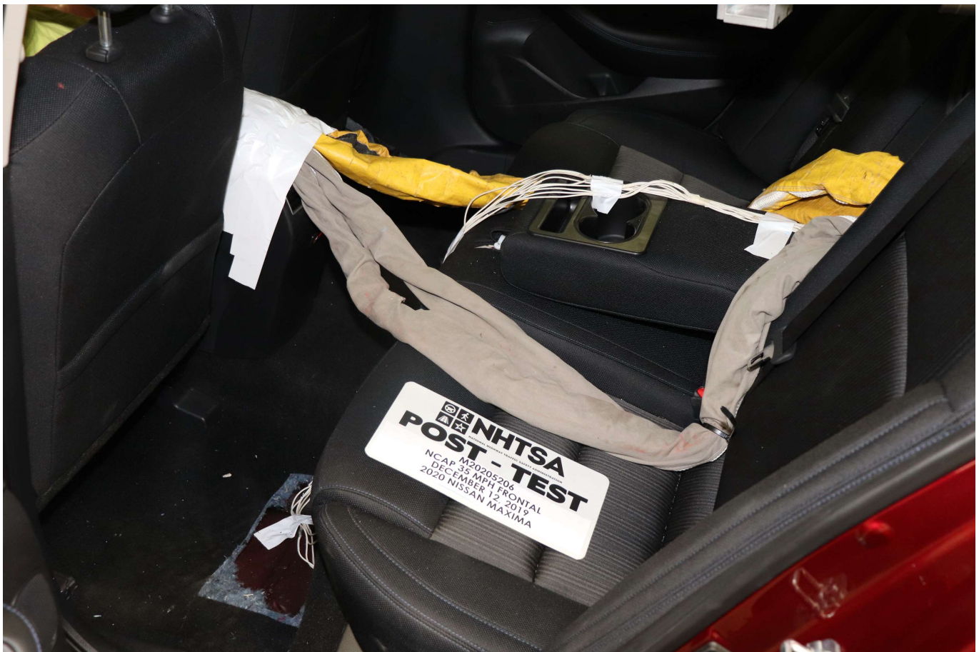
Photo No. 029 - Post-Test Dummy Cable Routing
