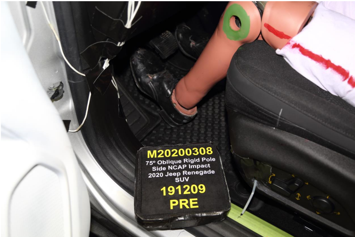
No. 032 Pre-Test Placement of Dummy Feet
