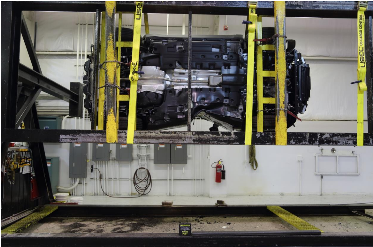
No. 066 FMVSS No. 301 Static Rollover 270 Degrees
