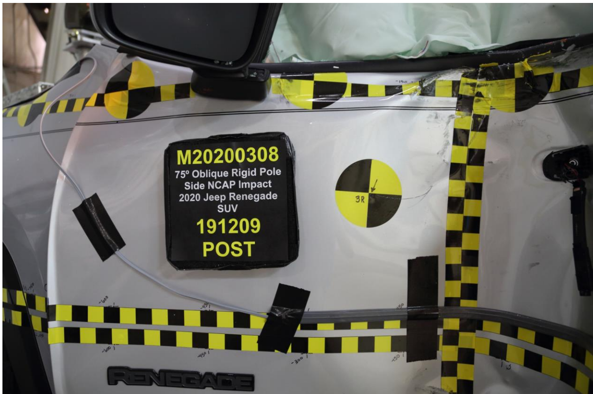
No. 020 Post-Test Close-Up View of Impact Point Target Showing Impact Location
