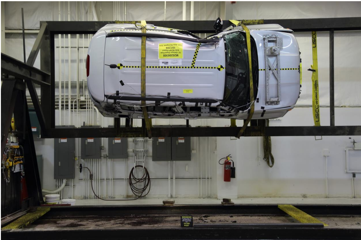
No. 064 FMVSS No. 301 Static Rollover 90 Degrees
