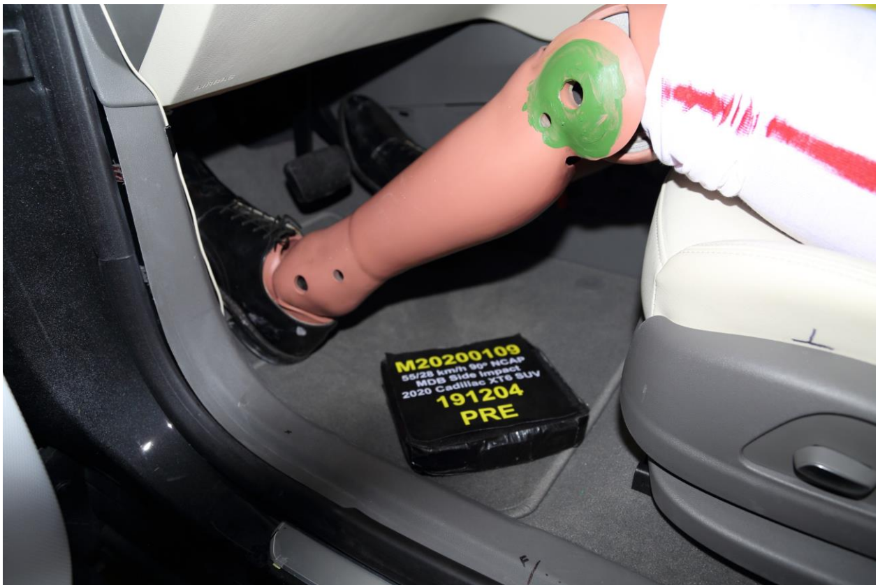
034 Pre-Test Placement of Driver's Dummy Feet
