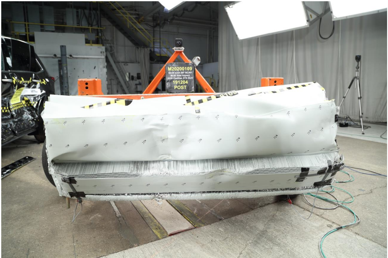
085 Post-Test Front View of MDB Impactor Face
