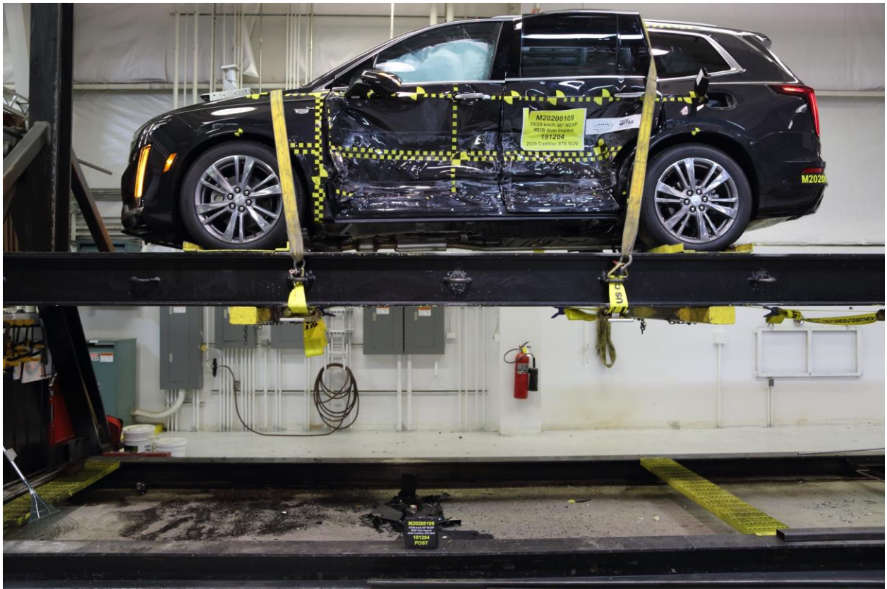
096 FMVSS No. 301 Static Rollover 0 Degrees
