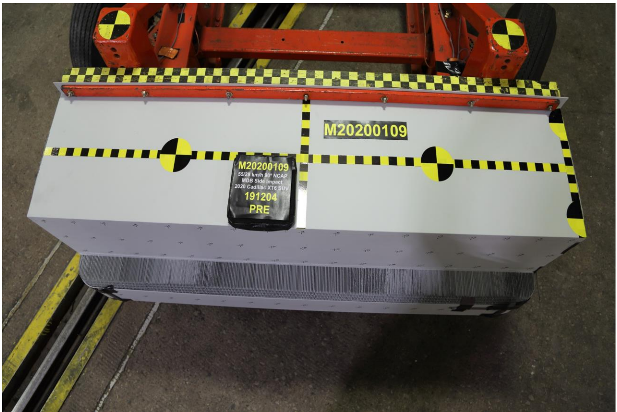
086 Pre-Test Top View of MDB Impactor Face
