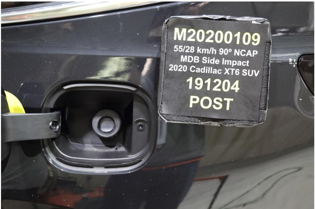
083 Post-Test View of Fuel Filler Cap or Fuel Filler Neck
