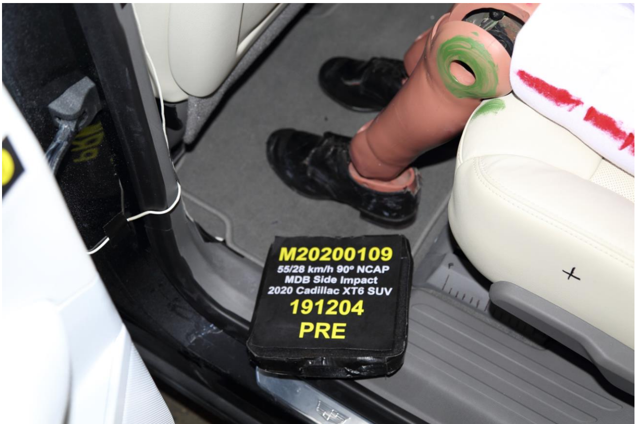
064 Pre-Test Placement of Rear Passenger Dummy's Feet
