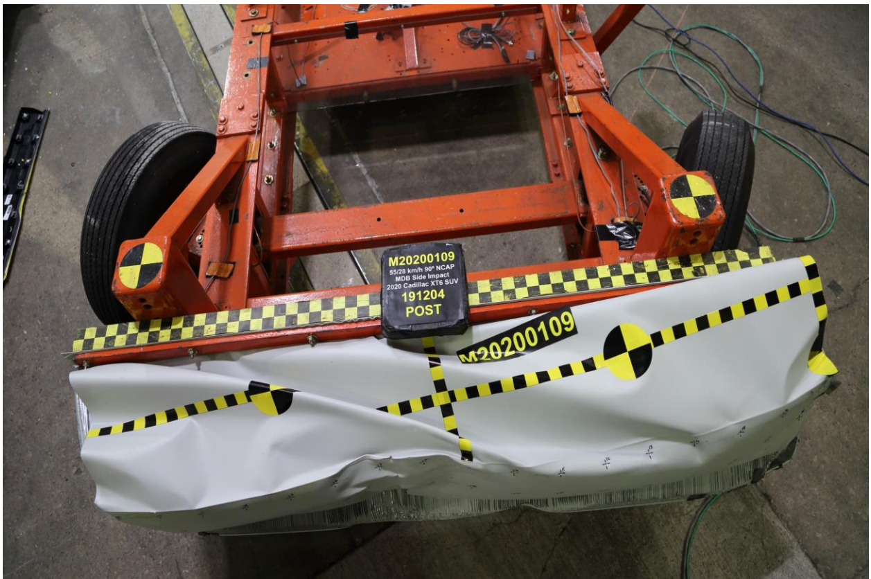
087 Post-Test Top View of MDB Impactor Face
