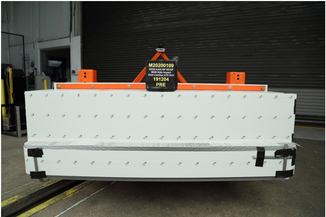
084 Pre-Test Front View of MDB Impactor Face
