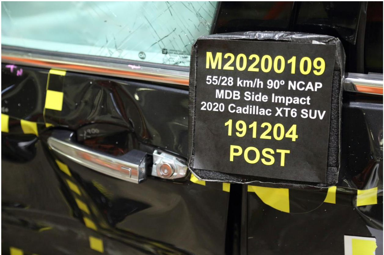
022 Post-Test Left Front Door Latch Close-Up
