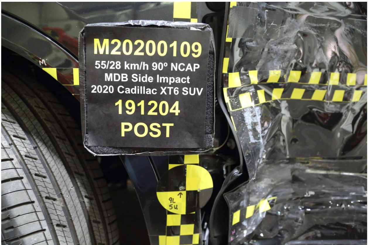
020 Post-Test Close-Up View of Impact Point Target
