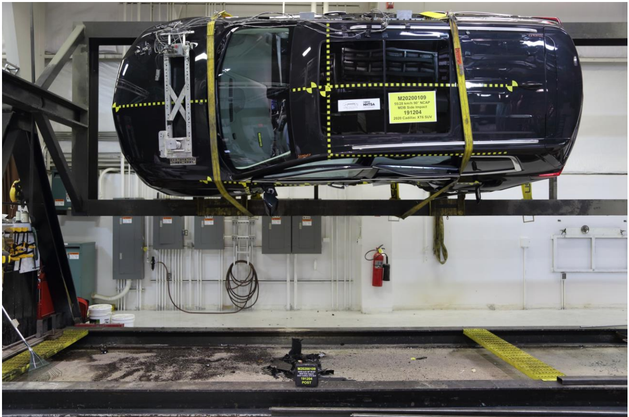
097 FMVSS No. 301 Static Rollover 90 Degrees
