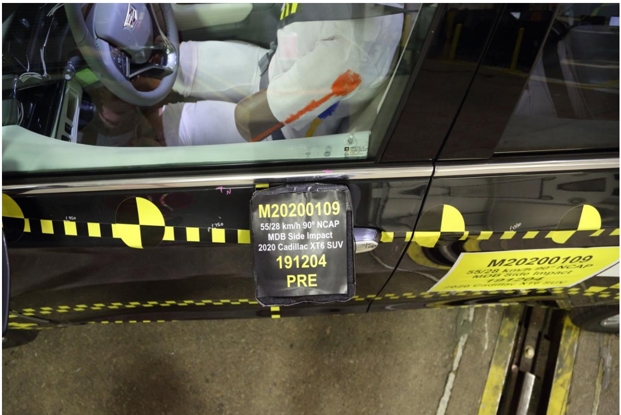
042 Pre-Test Driver Dummy and Door Clearance View
