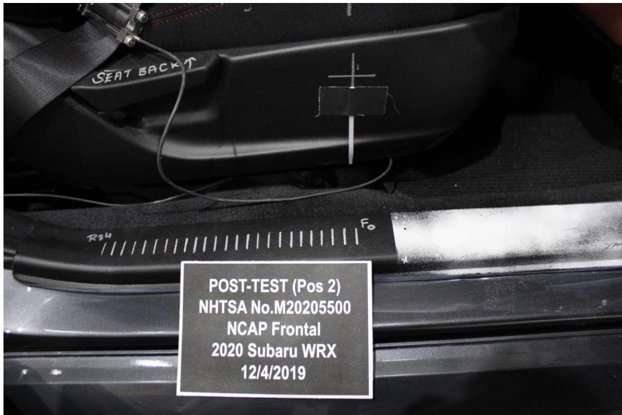
Figure A-60: Post-Test Passenger's Seat Fore-Aft Markings
