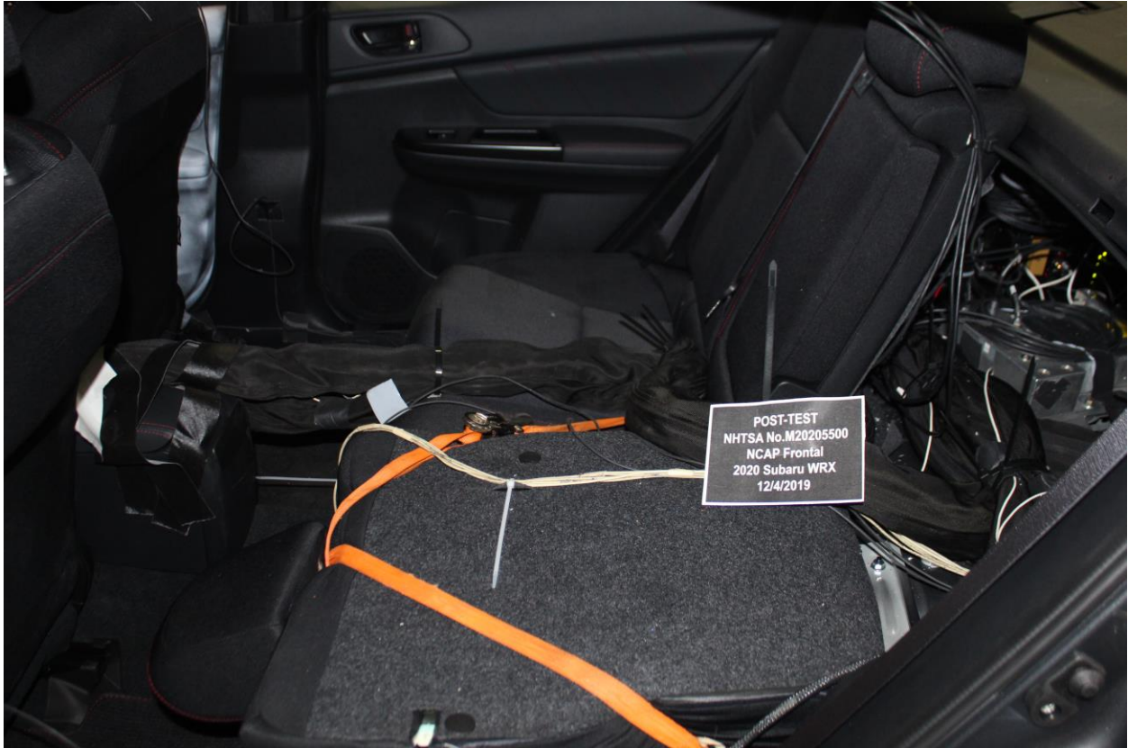
Figure A-29: Post-Test Dummy Cable Routing
