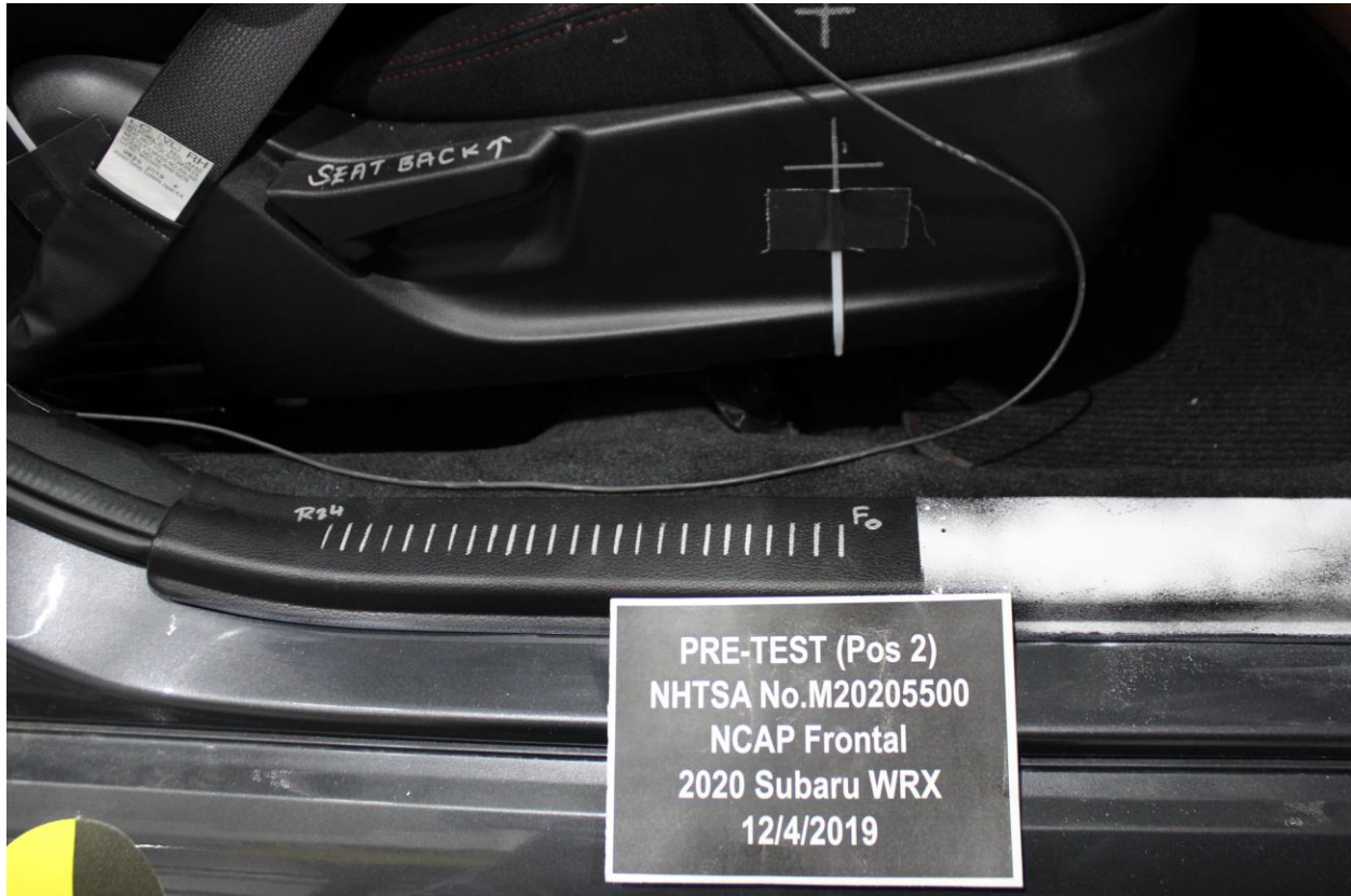
Figure A-59: Pre-Test Passenger's Seat Fore-Aft Markings
