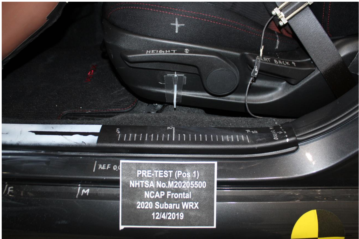
Figure A-36: Pre-Test Driver's Seat Fore-Aft Markings
