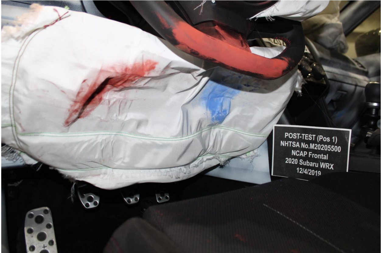
Figure A-45: Post-Test Driver's Side Knee Bolster
