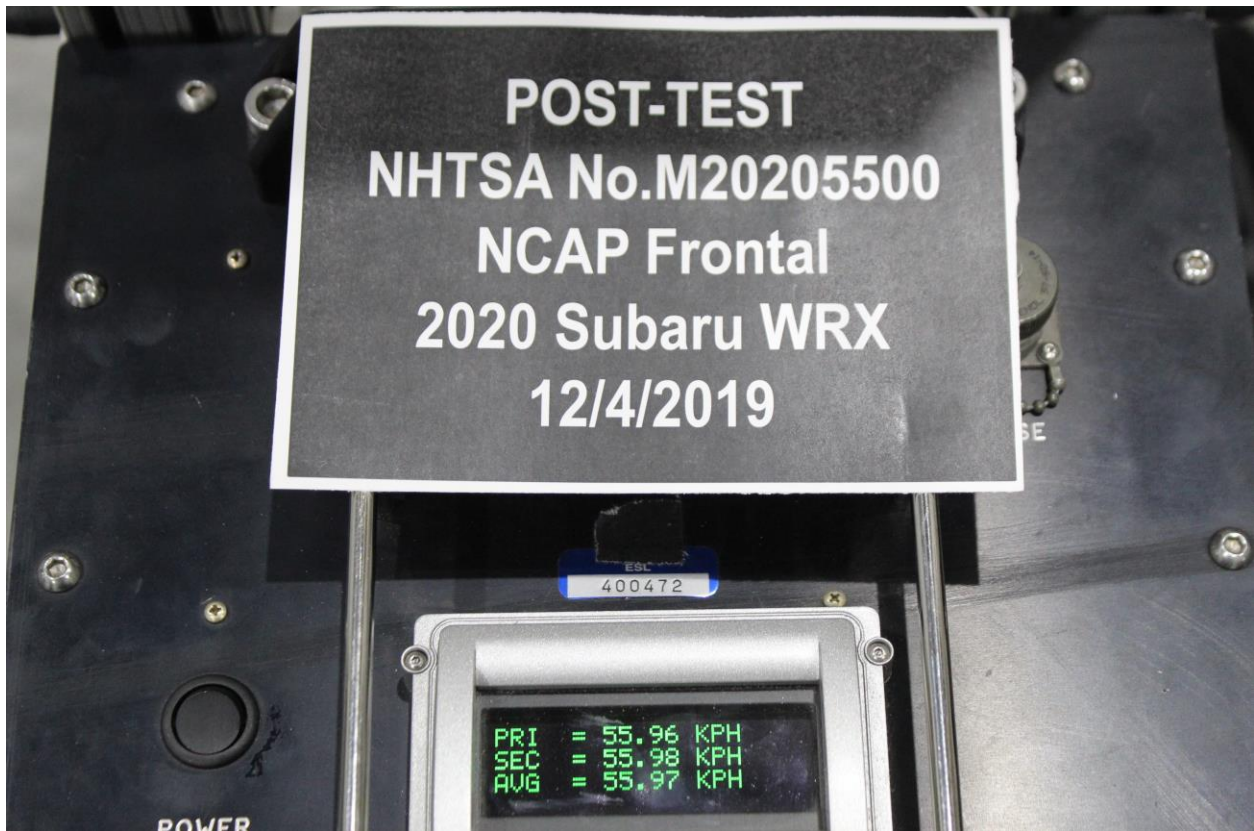
Figure A-76: Post-Test Speed Trap Read-Out
