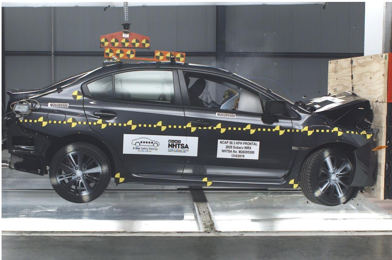
Figure A-82: 2020 Subaru WRX Frontal Impact Event
