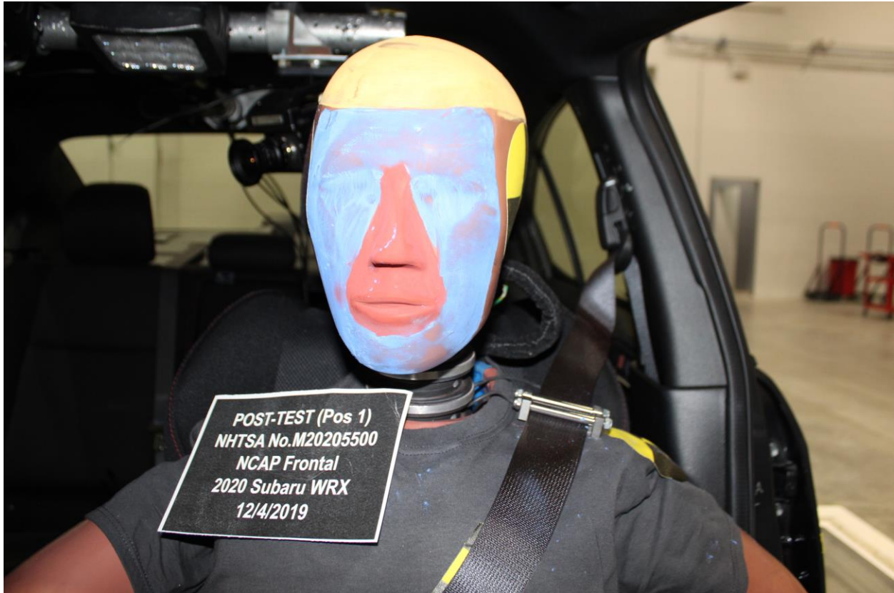
Figure A-48: Post-Test Driver Dummy Face
