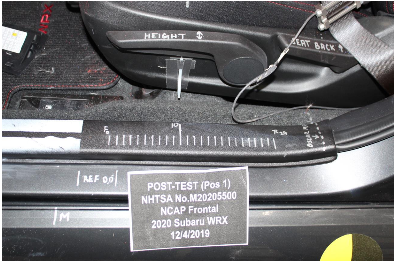
Figure A-37: Post-Test Driver's Seat Fore-Aft Markings
