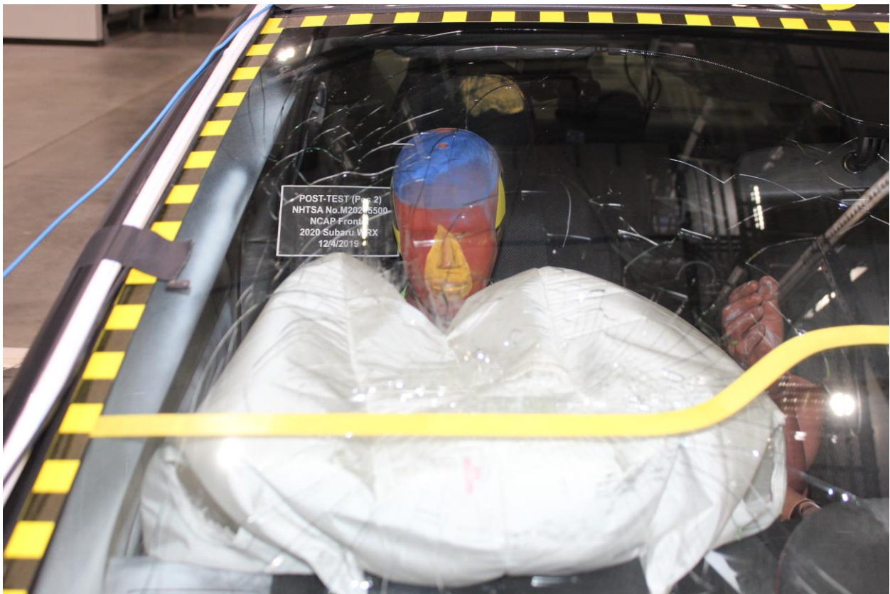
Figure A-54: Post-Test Passenger Dummy Front View
