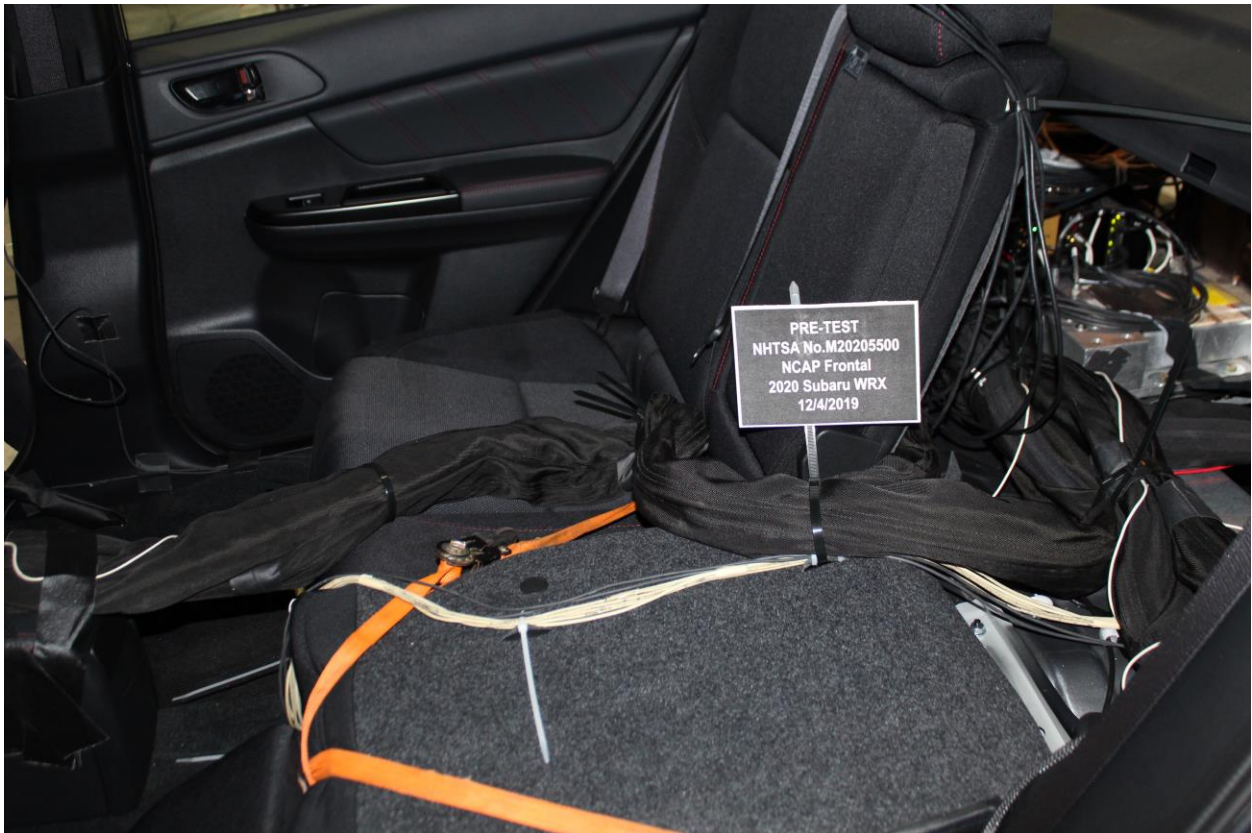
Figure A-28: Pre-Test Dummy Cable Routing
