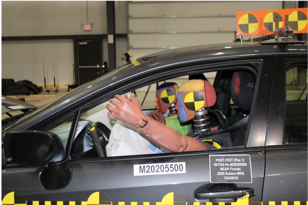
Figure A-33: Post-Test Driver Dummy Window View
