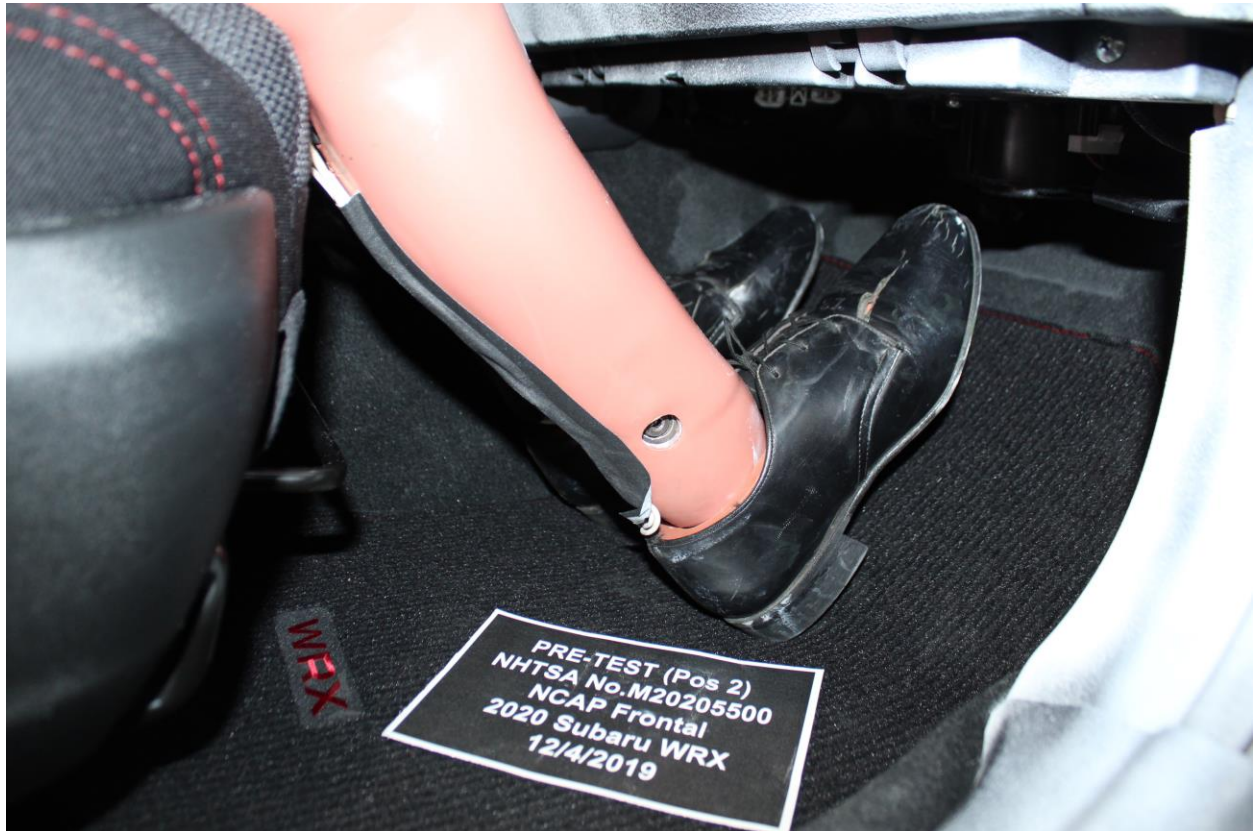
Figure A-65: Pre-Test Passenger Dummy Feet
