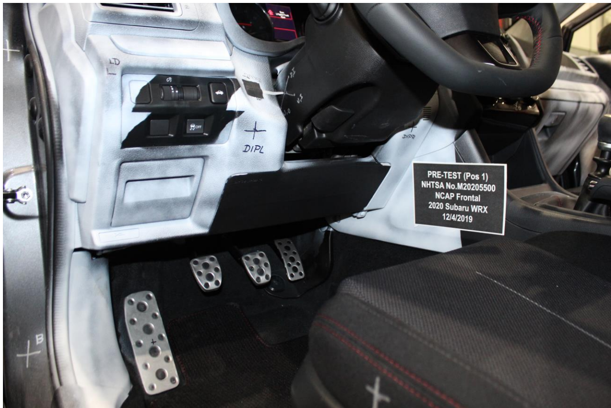
Figure A-44: Pre-Test Driver's Side Knee Bolster
