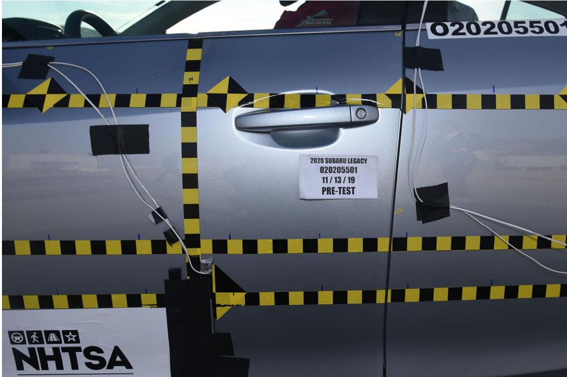
FIGURE 21. Pre-Test Left Front Door Latch Close-Up
