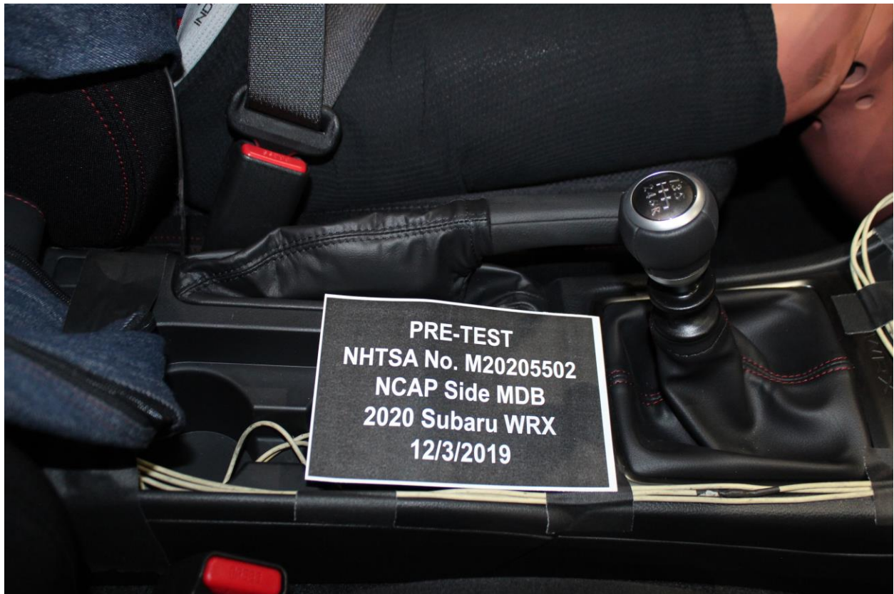
Figure A-37: View of Disengaged Parking Brake
