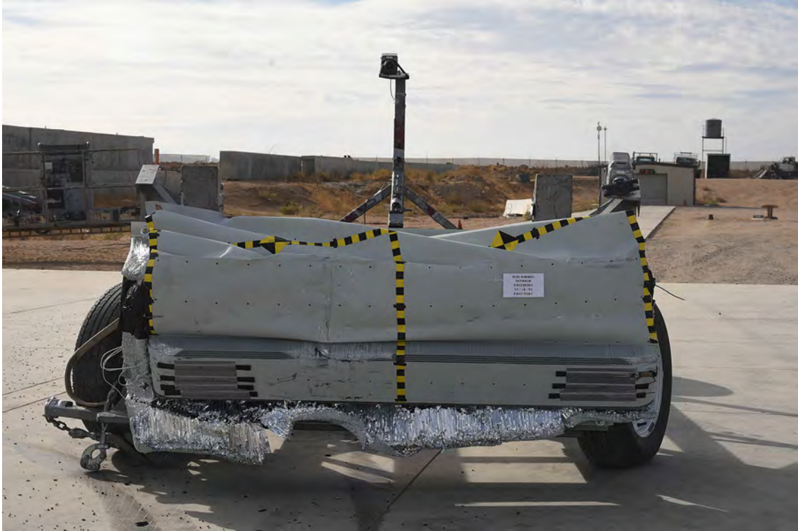
FIGURE 85. Post-Test Front View of MDB Impactor Face
