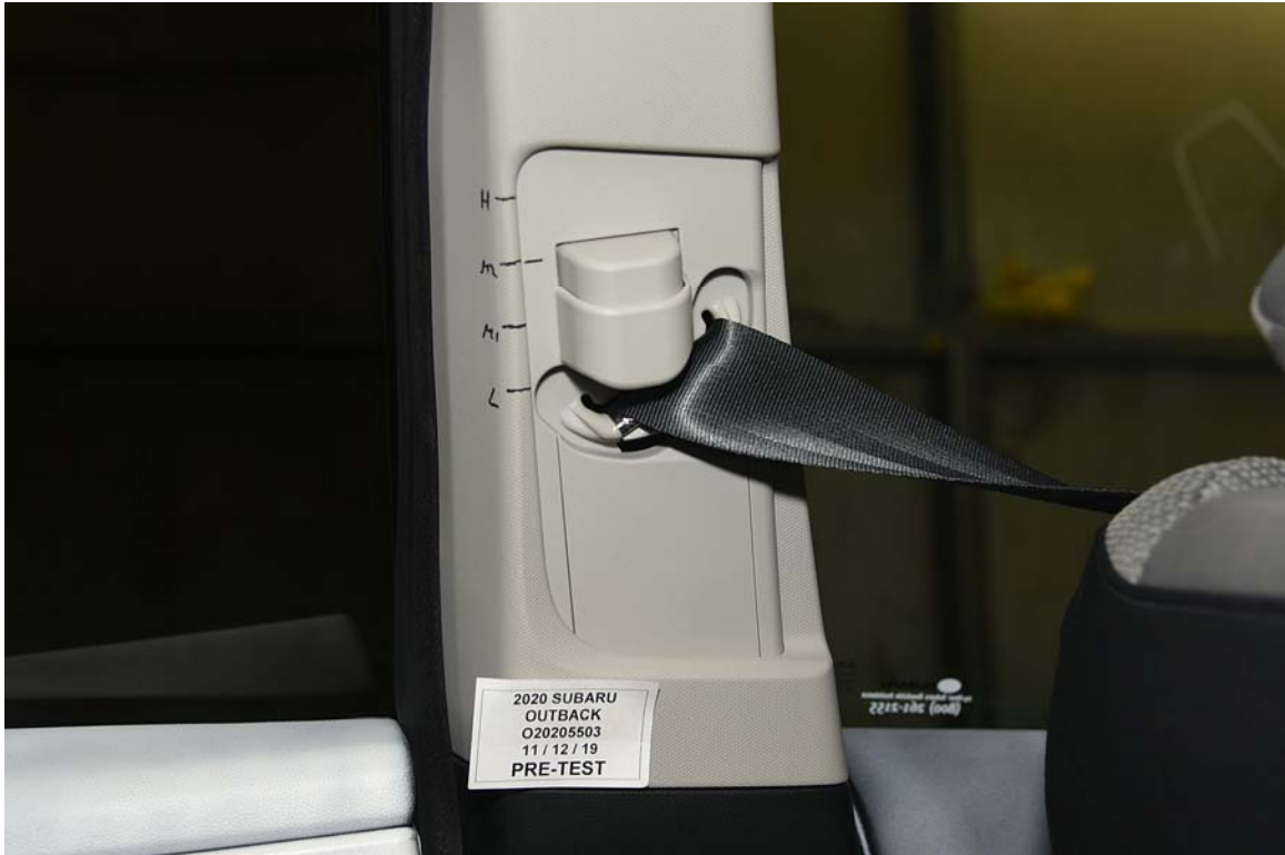
FIGURE 33. Pre-Test View of Belt Anchorage for Dummy
