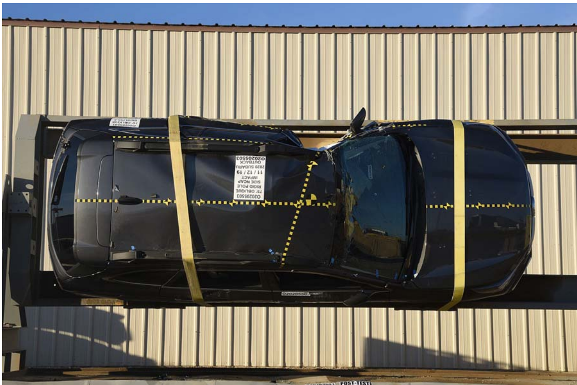
FIGURE 64. FMVSS No. 301 Static Rollover 90 Degrees
