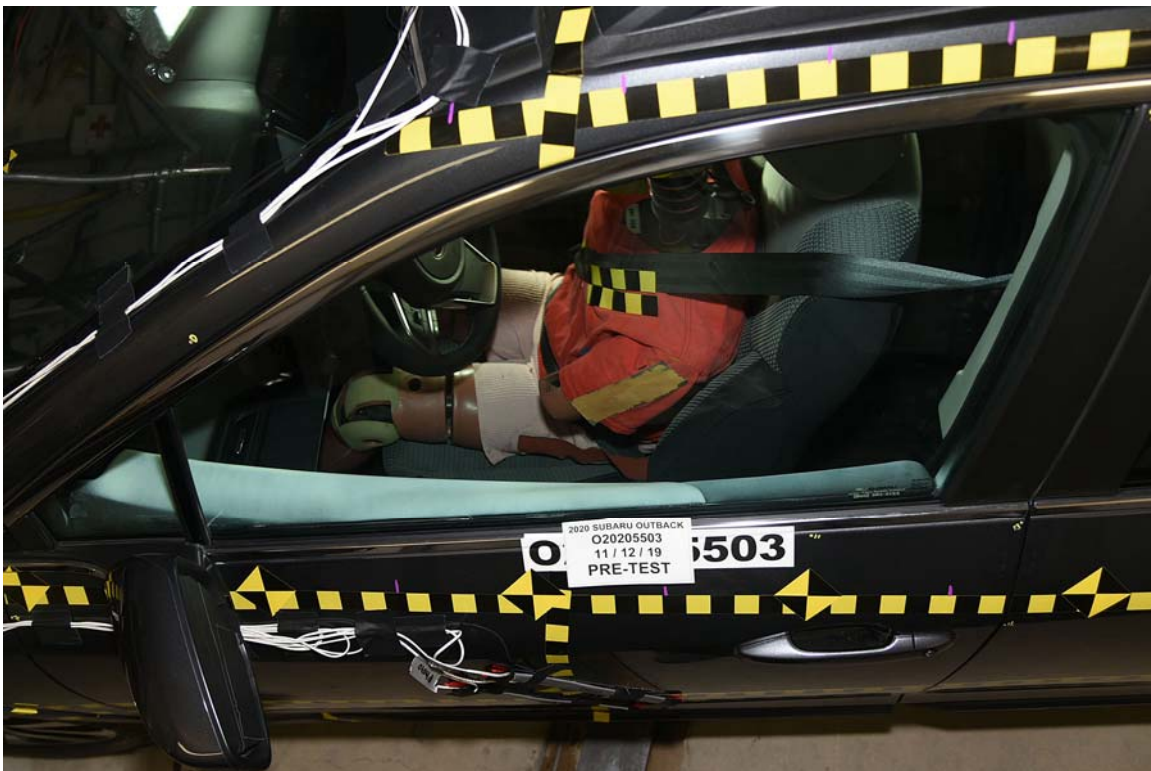
FIGURE 40. Pre-Test Dummy and Door Clearance View
