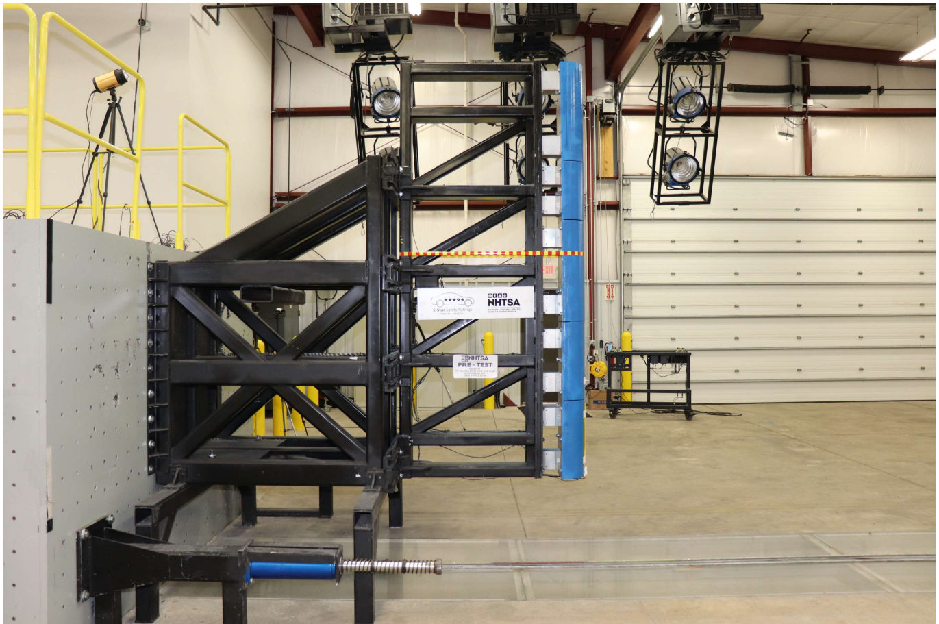
Photo No. 059 - Pre-Test Pole Barrier Side View
