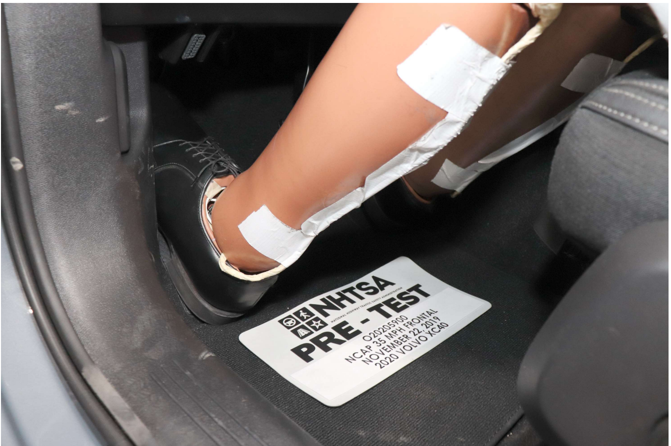
Photo No. 042 - Pre-Test Driver Dummy Feet
