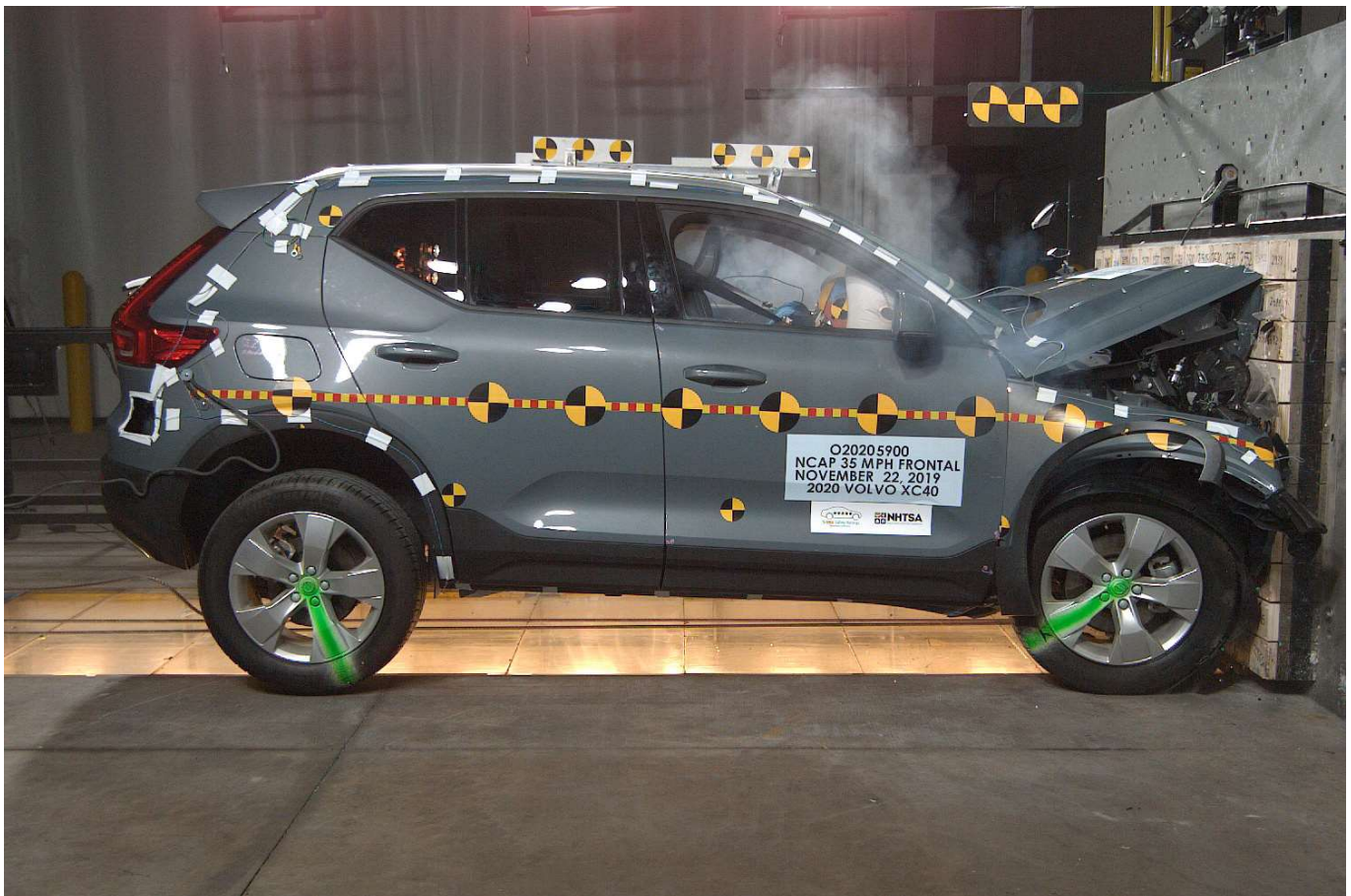
Photo No. 082 - 2020 Volvo XC40 T5 AWD Momentum 5-Door SUV Frontal Impact Event
