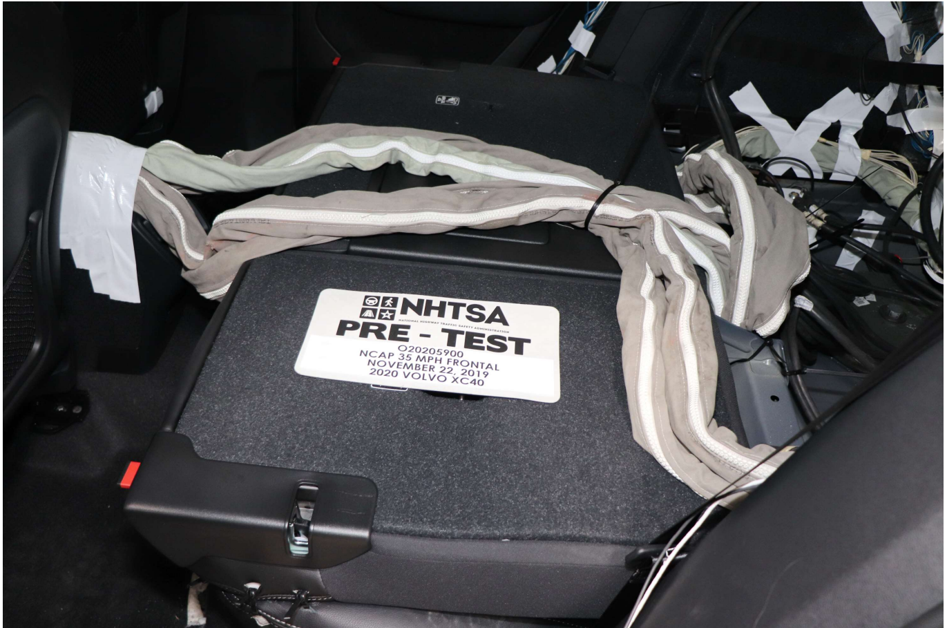
Photo No. 028 - Pre-Test Dummy Cable Routing
