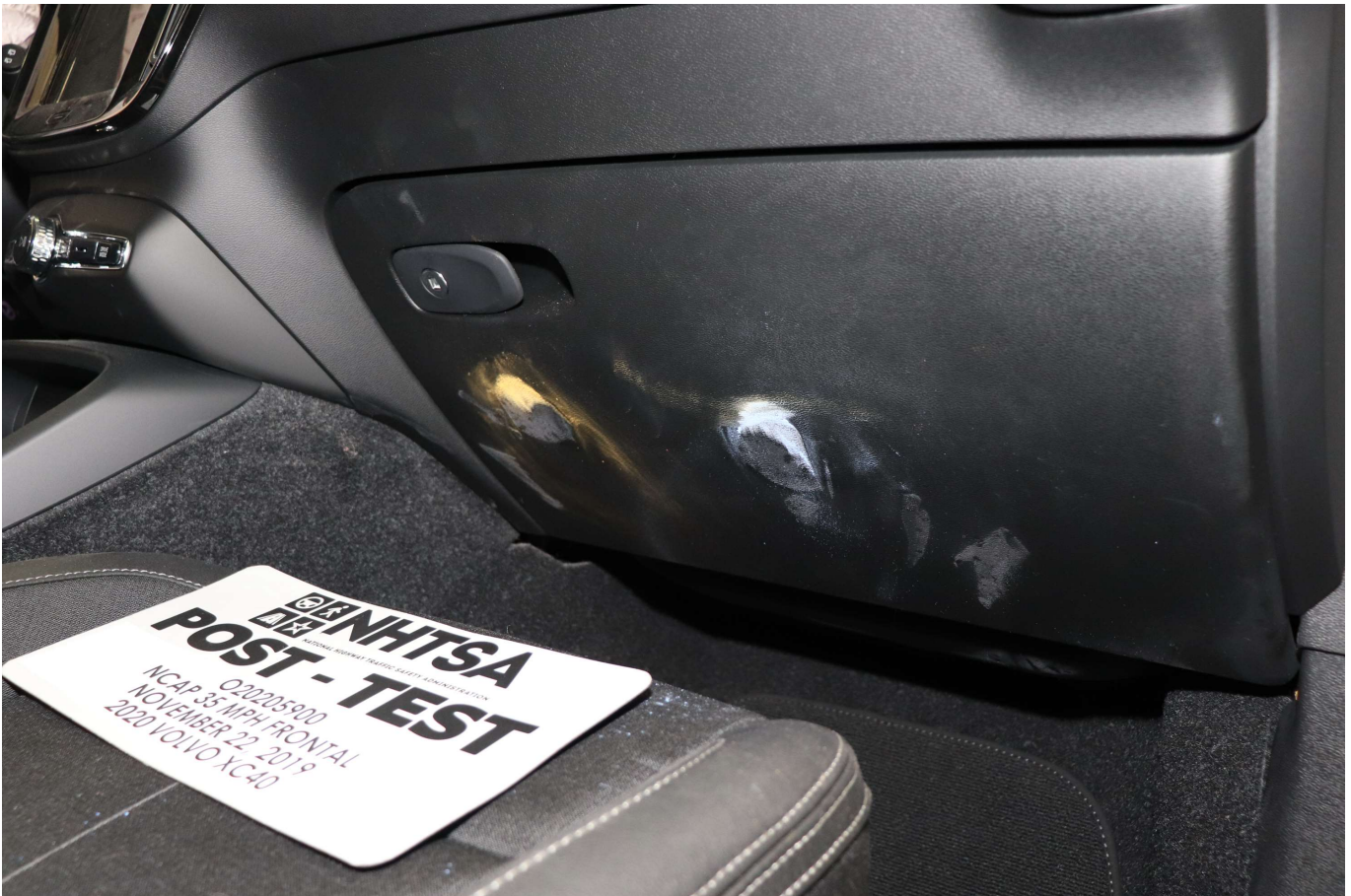
Photo No. 068 - Post-Test Passenger Side Knee Bolster
