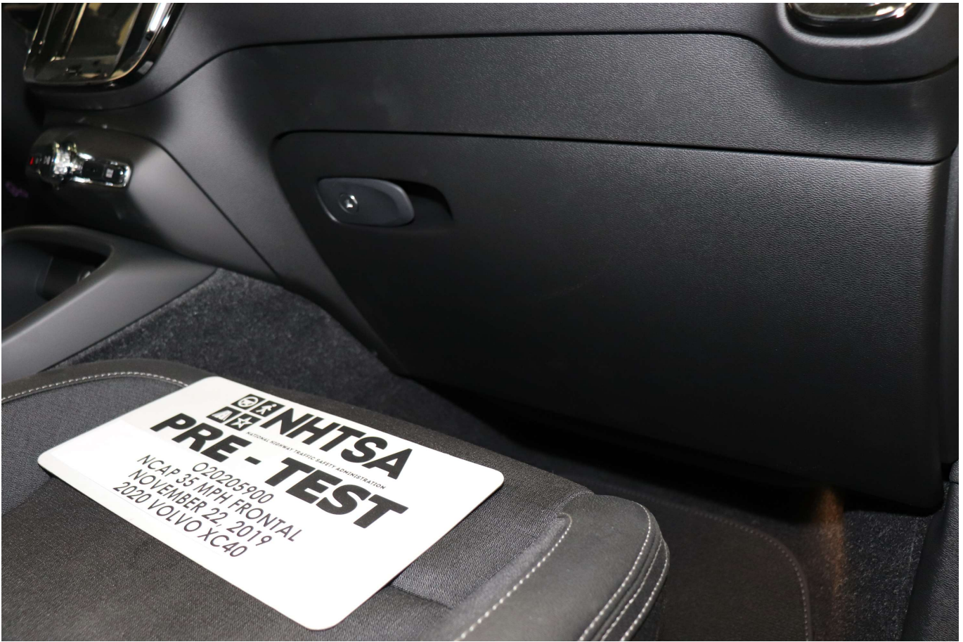
Photo No. 067 - Pre-Test Passenger Side Knee Bolster
