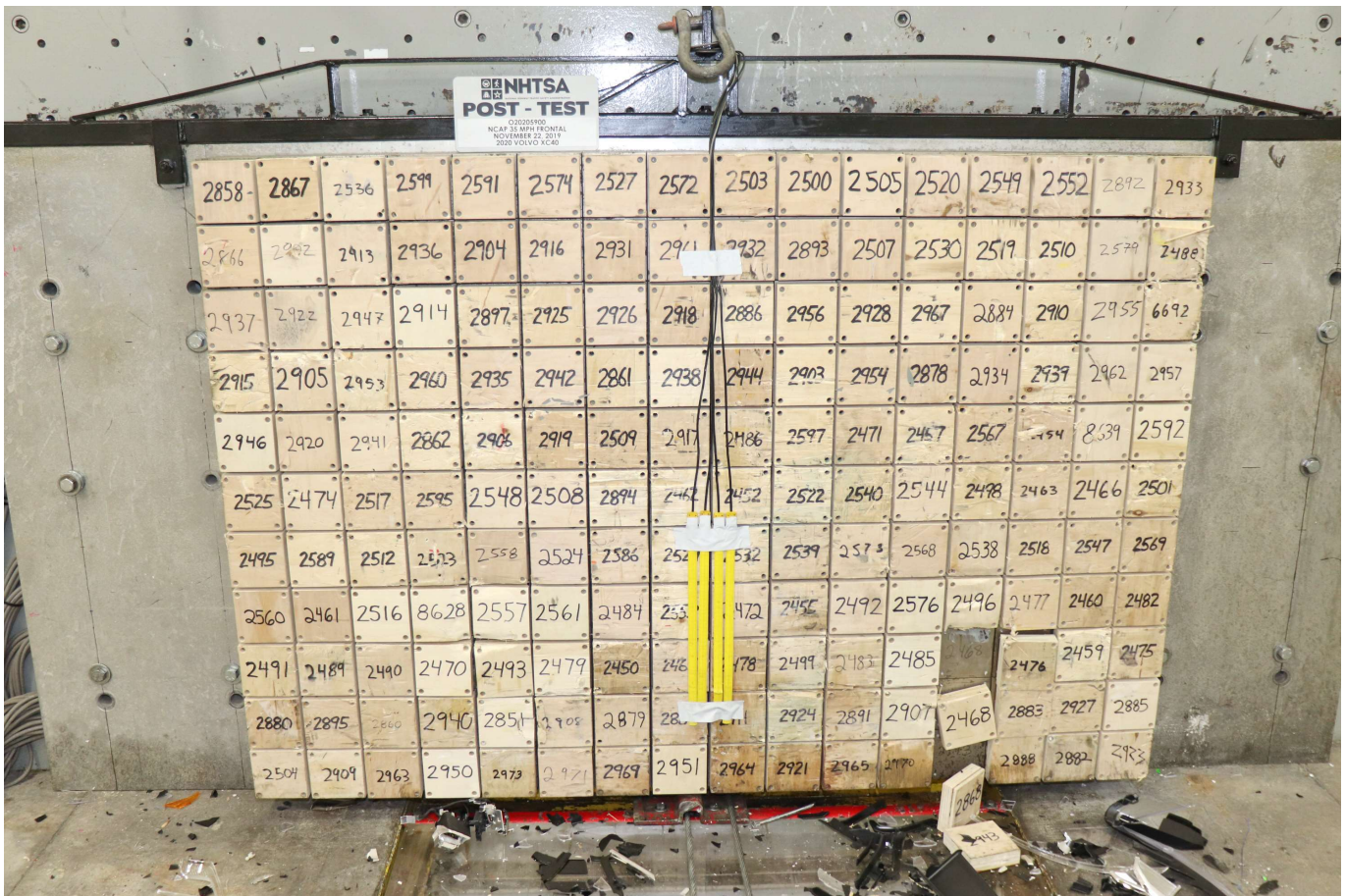
Photo No. 003 - Post-Test Load Cell Wall
