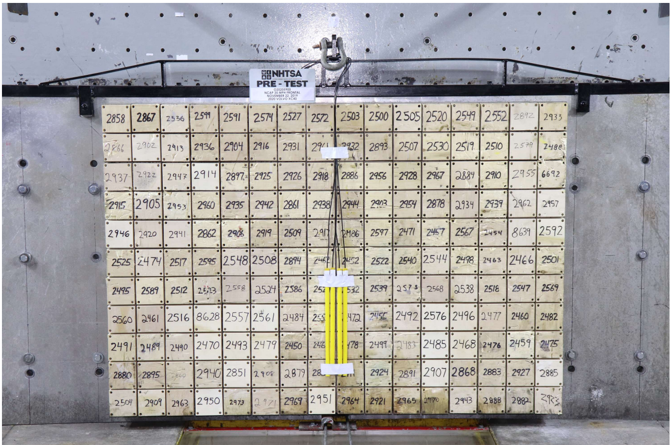
Photo No. 002 - Pre-Test Load Cell Wall
