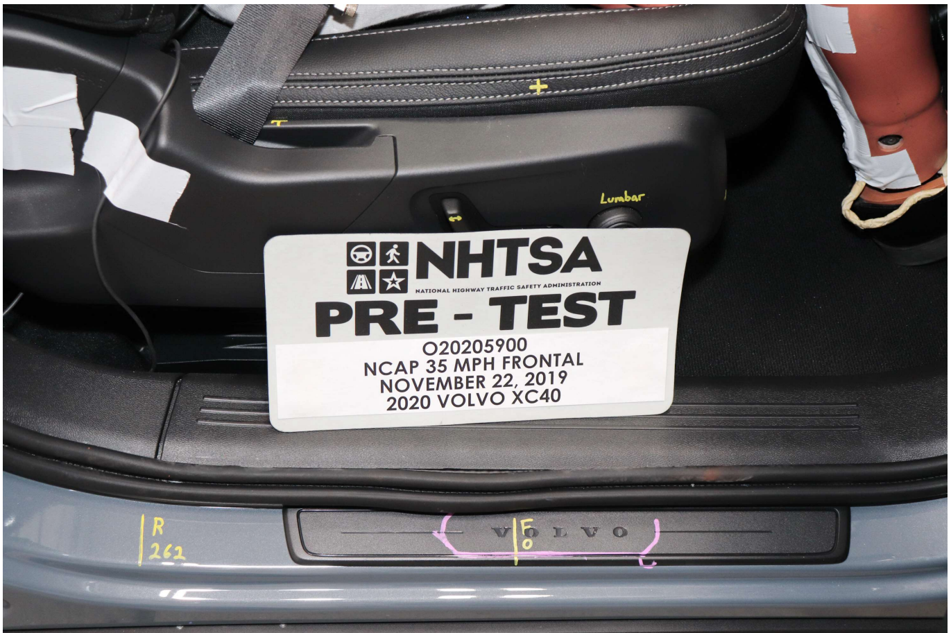
Photo No. 059 - Pre-Test Passenger Seat Fore-Aft Markings
