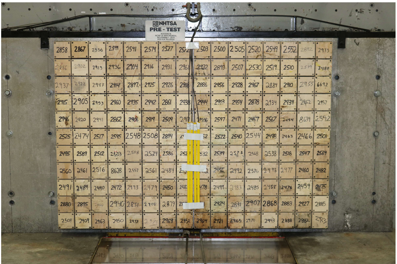
Photo No. 002 - Pre-Test Load Cell Wall
