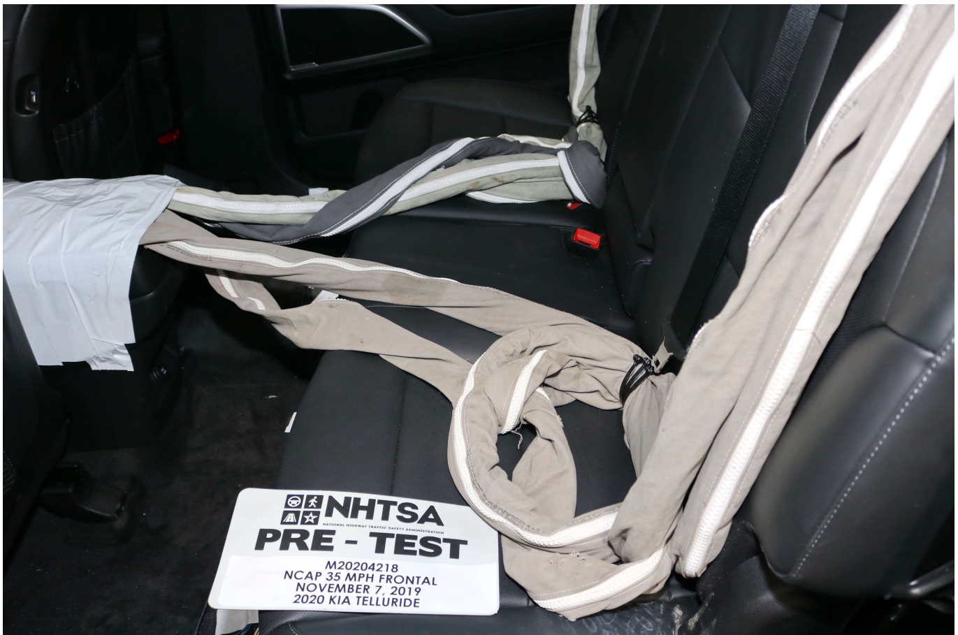
Photo No. 028 - Pre-Test Dummy Cable Routing
