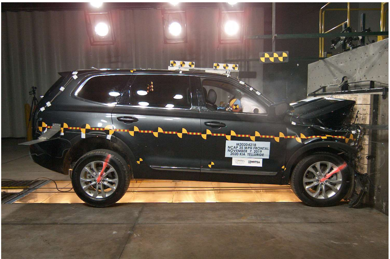
Photo No. 082 - 2020 Kia Telluride LX AWD 5-Door SUV Frontal Impact Event
