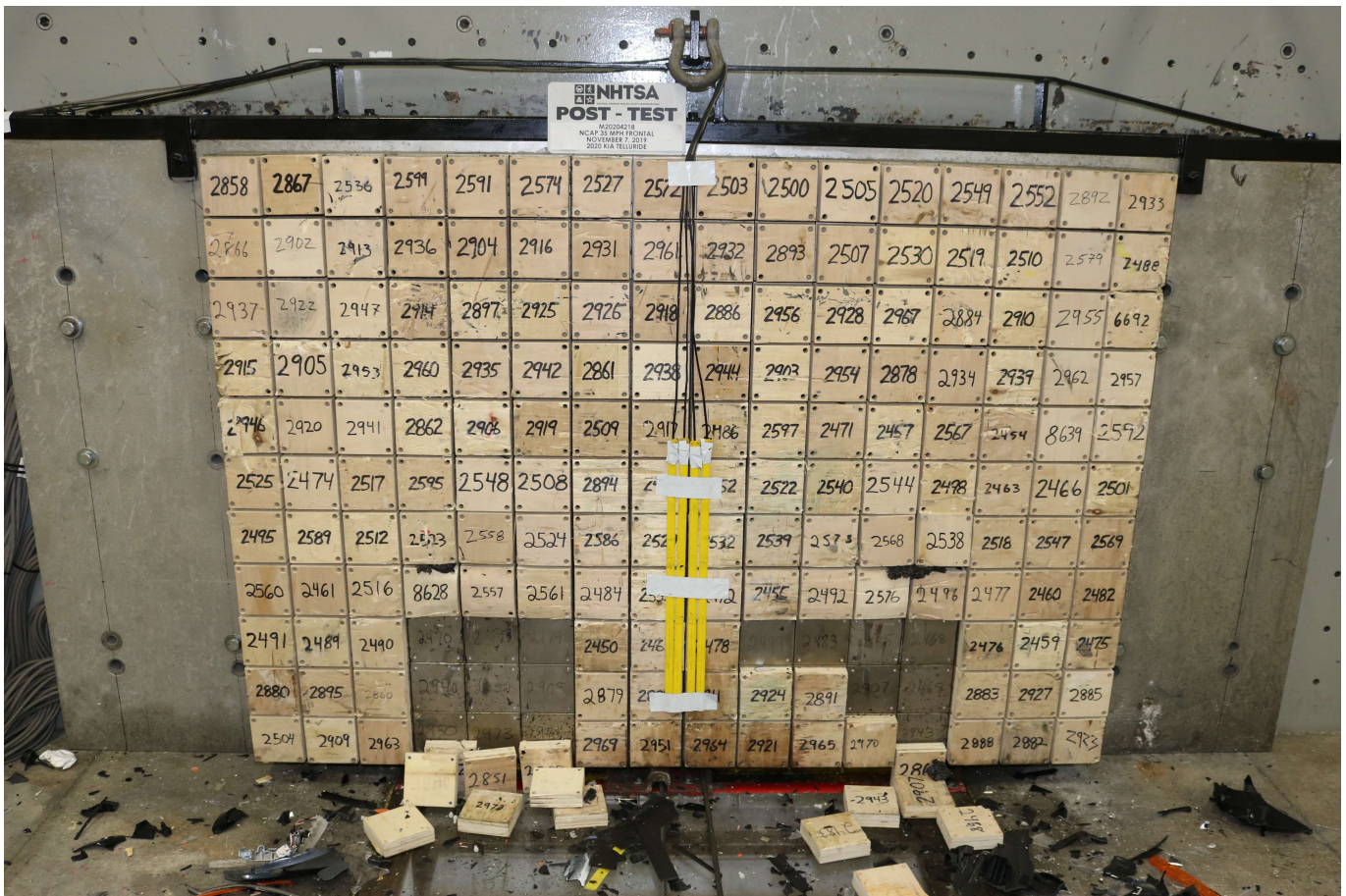
Photo No. 003 - Post-Test Load Cell Wall
