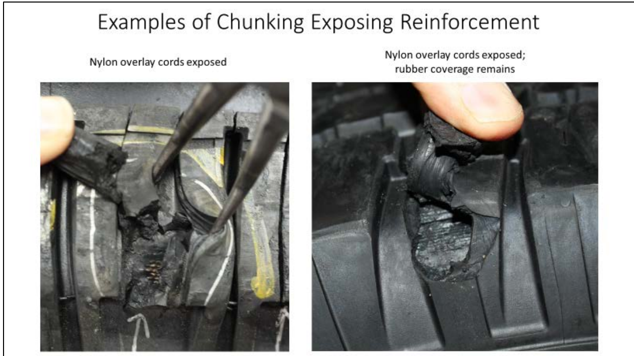
Figure 2. Non-parasitic chunking that exposes reinforcing cords.
