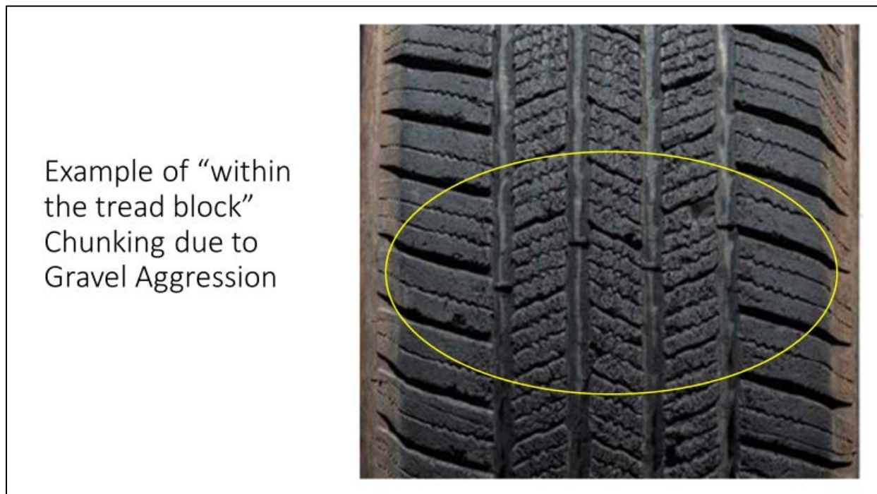
Figure 3. Tread chunking observed in the field due to gravel aggression, which can be visually distinguished from PTBC, which is purely a laboratory testing phenomenon.
