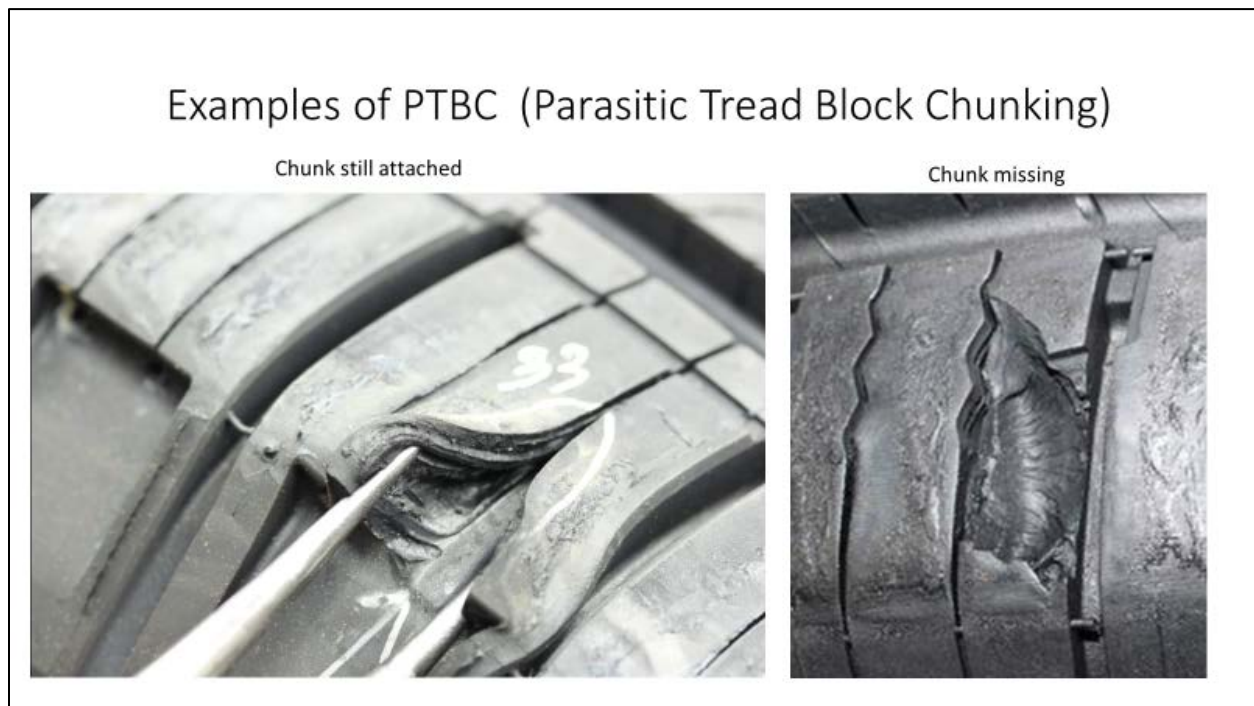
Figure 1. Parasitic Tread Block Chunking (PTBC) example.
