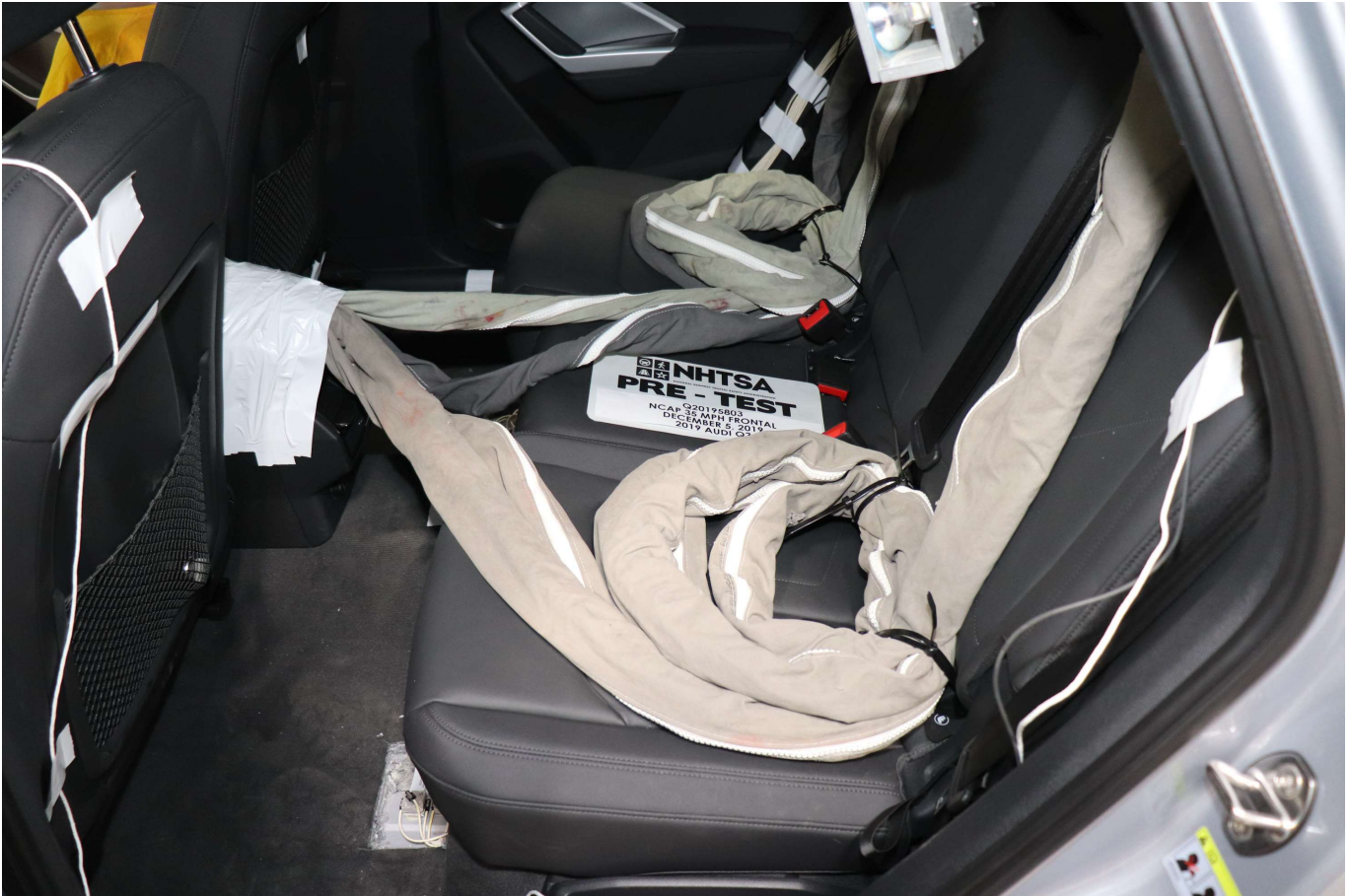
Photo No. 028 - Pre-Test Dummy Cable Routing
