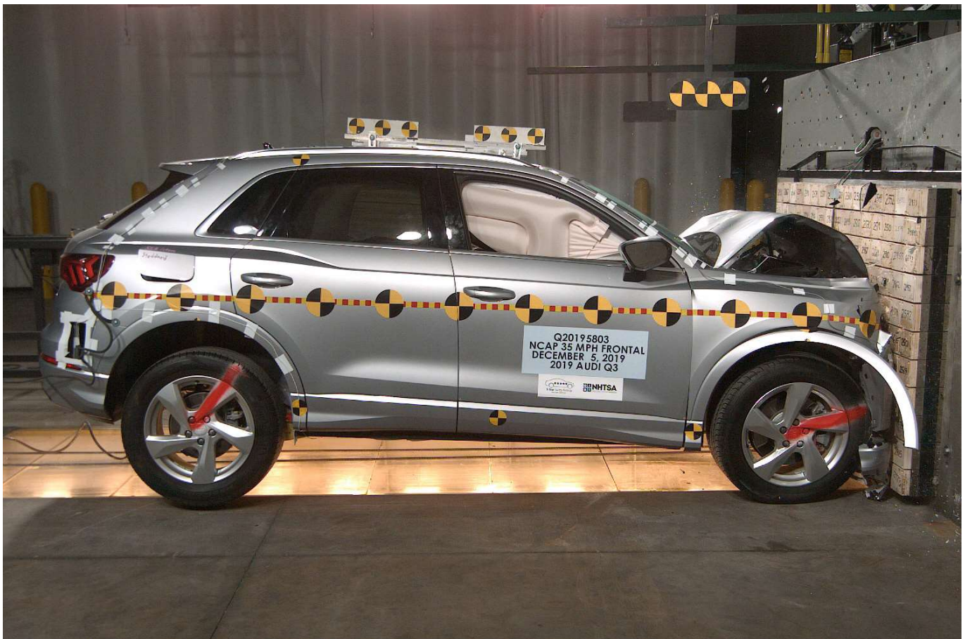
Photo No. 082 - 2019 Audi Q3 5-Door SUV Frontal Impact Event
