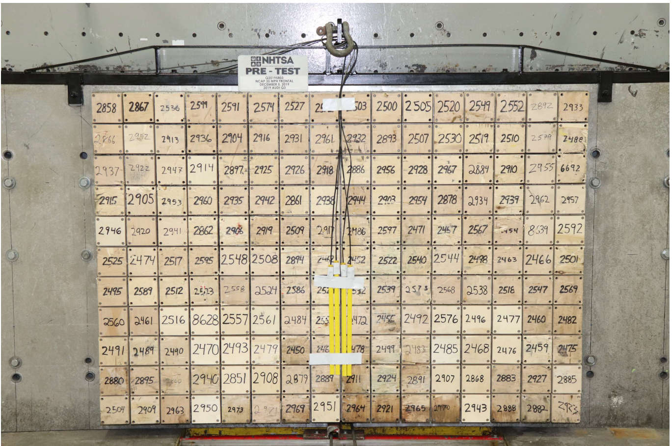
Photo No. 002 - Pre-Test Load Cell Wall
