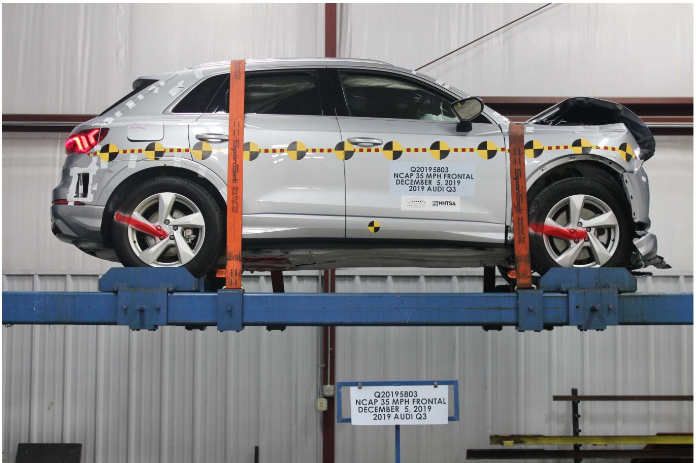
Photo No. 081 - Vehicle at 360 Degrees on Static Rollover Device
