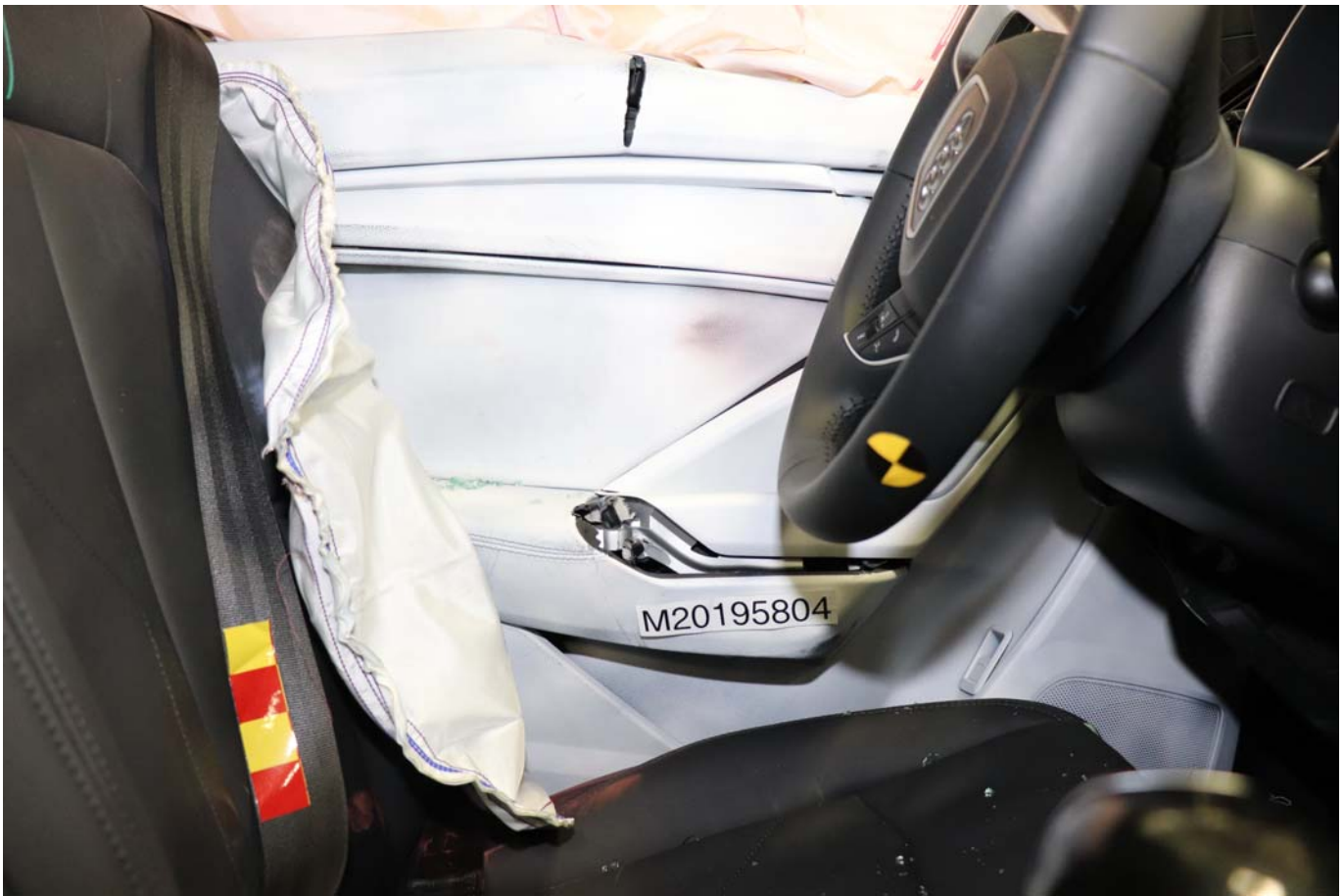
Photo No. 071 - Post-Test View of Shattered Vehicle Inner Door Panel
