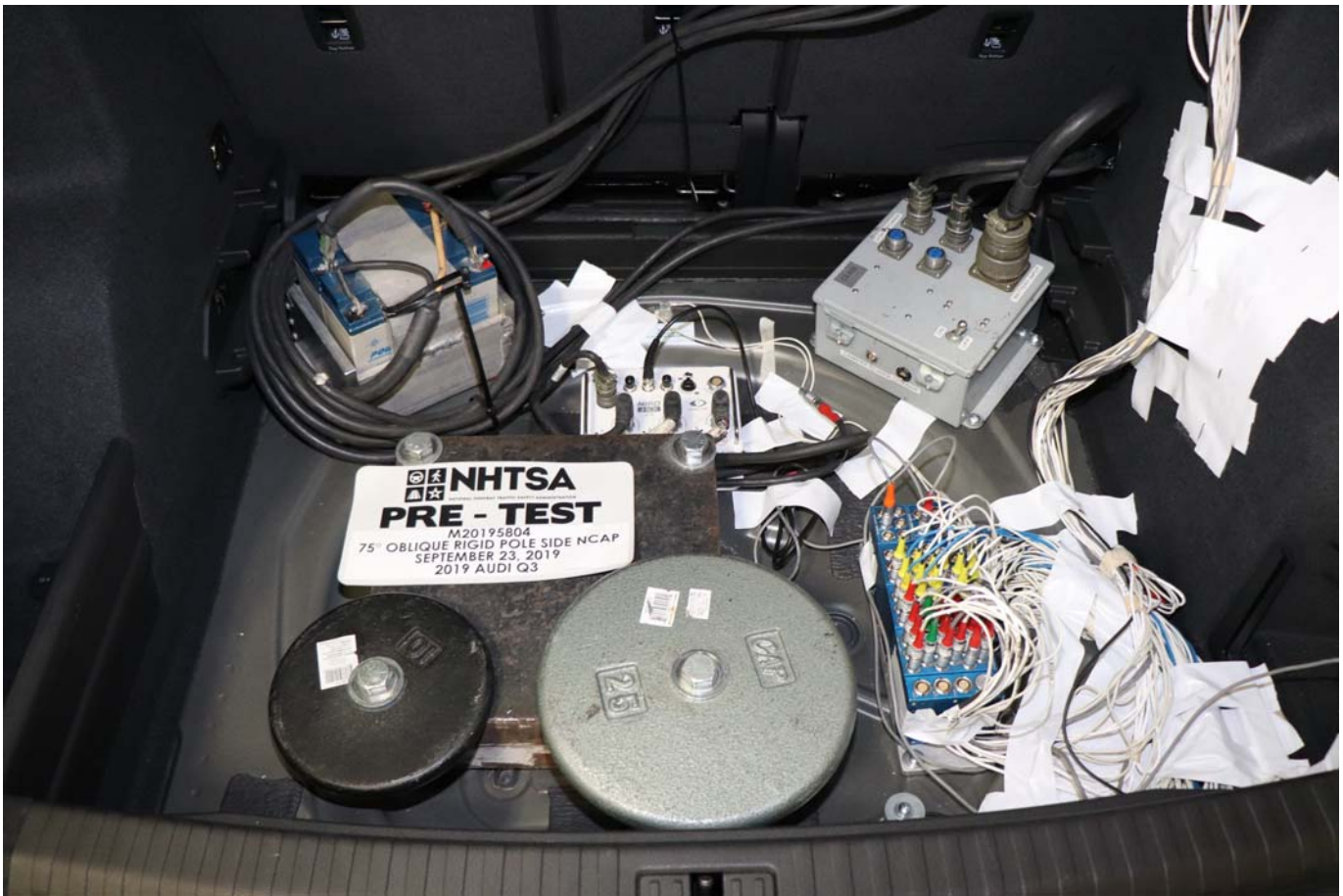
Photo No. 061 - Pre-Test Ballast View
