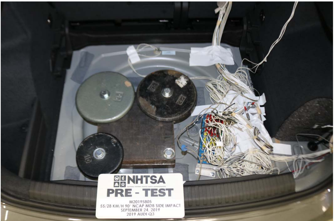
Photo No. 094 - Pre-Test Ballast View
