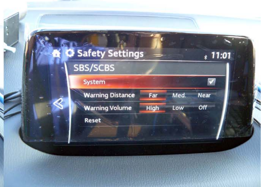
Figure A12. FCW System Setting Menus
