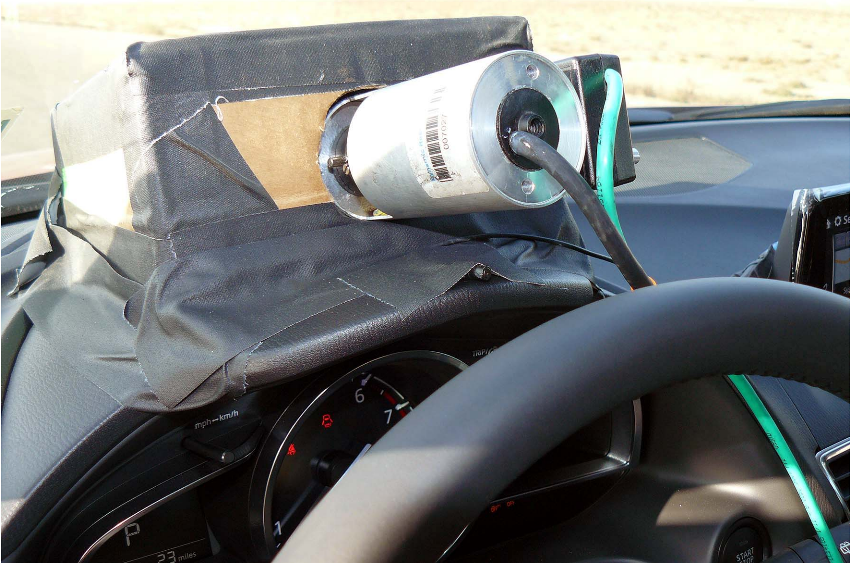
Figure A9. Sensor for Detecting Auditory and Visual Alerts
