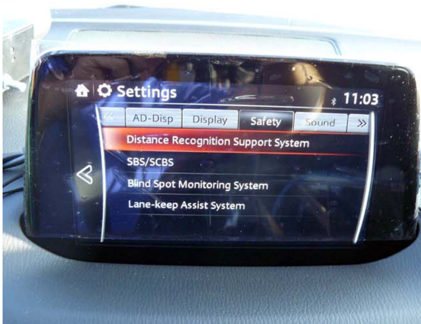
Figure A12. FCW System Setting Menus
